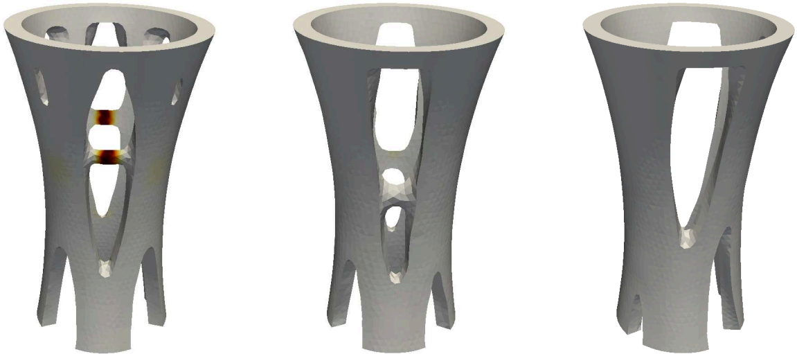
Figure 6.35: damage variable \alpha at the final time computed for the optimized shapes in Fig.6.32, damage model (6.17), isotropic degradation (6.75), imposed displacement (6.84)
