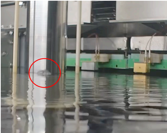
(a) Bubble from the High Voltage FeedThrough
