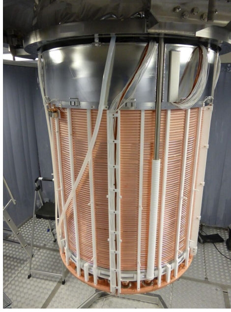
Figure 2.7: Picture of the XENON1T TPC fieldcage.
