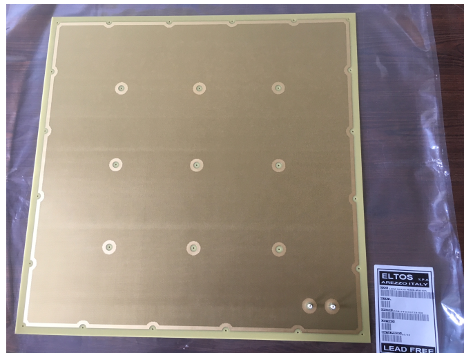
Figure 3.6: LEM used in ProtoDUNE Dual-Phase (CFR-35). The nine central holes are used to screw the LEM and anode together. The two bottom right pins are for high voltage connection.
