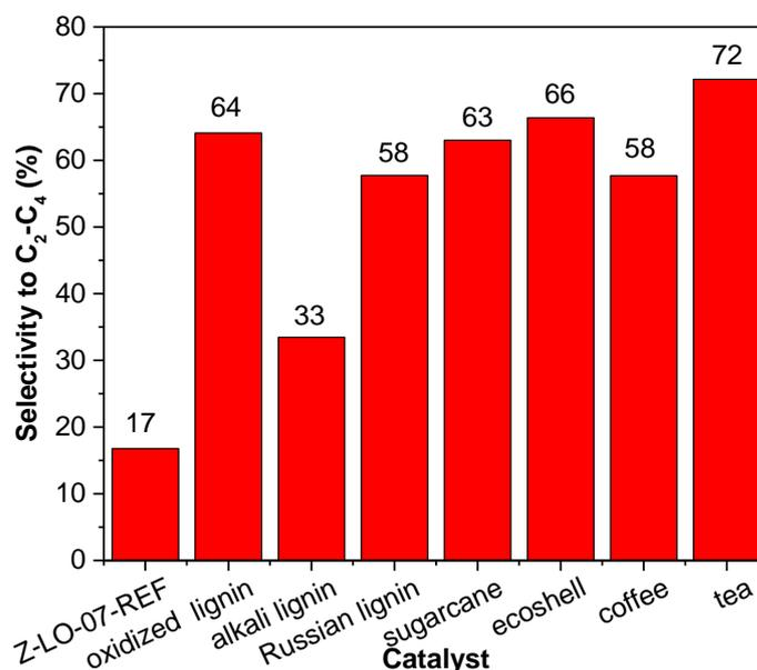
**Figure 4.10** Selectivities in light olefins (C<sub>2</sub>-C<sub>4</sub>) over Z-LO-07-REF and Z-LO-07 zeolites with different kinds of biomass (300 mg).
