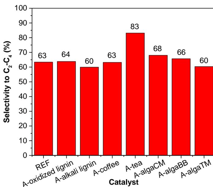
**Figure 4.15** Selectivities towards light olefins (C<sub>2</sub>-C<sub>4</sub>) over A-REF and biomass-derived A-ZSM-5. Reaction conditions: 450 °C, WHSV = 2 h<sup>-1</sup>, catalyst weight = 60 mg, TOS = 1 h.
