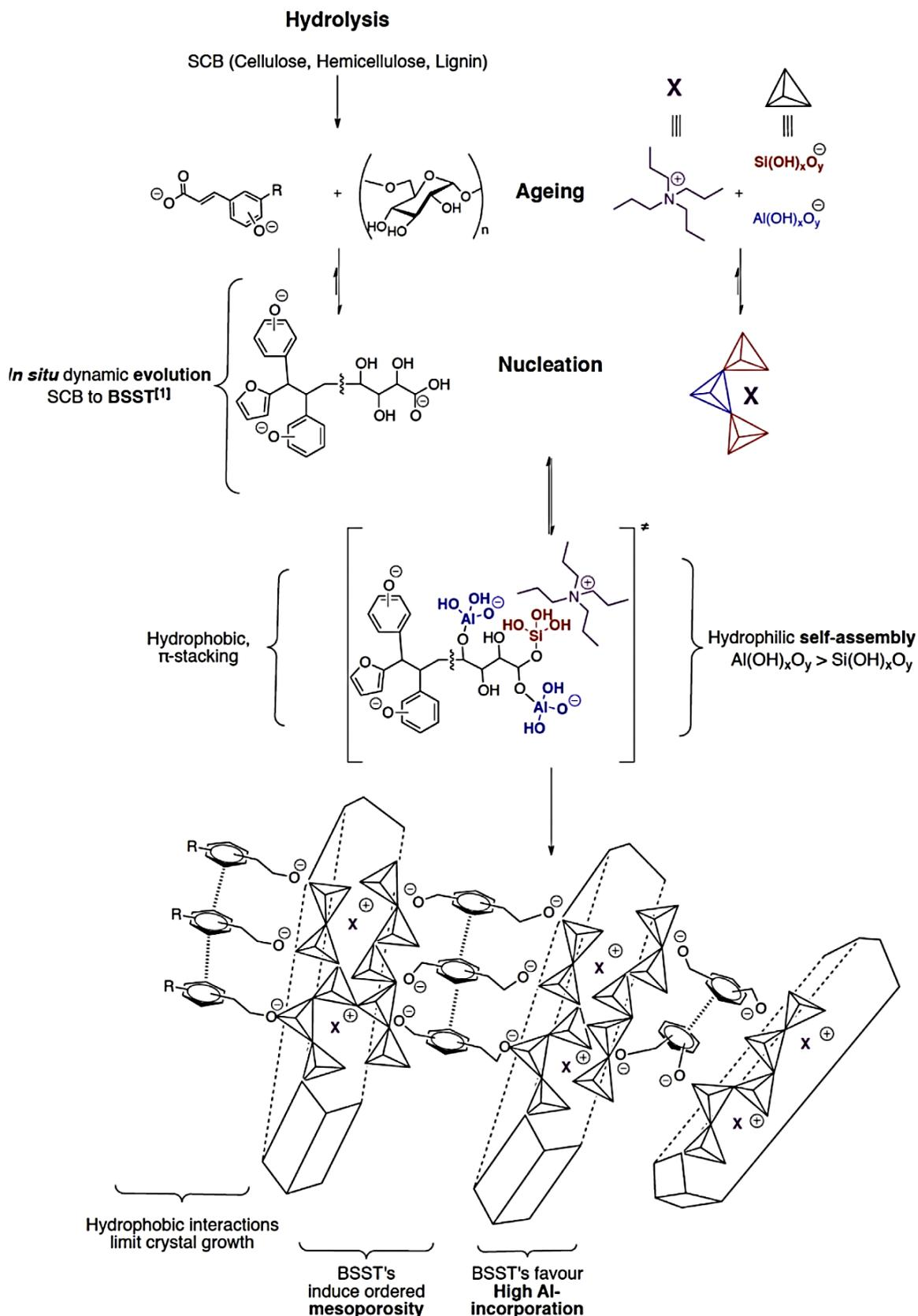
**Figure 1.20** Proposed mechanism involving BSST-assisted zeolite synthesis.<sup>6</sup>
