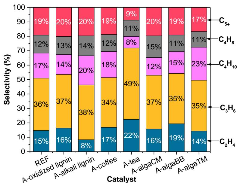
**Figure 4.14** Selectivities towards ethylene, propylene, isobutane, butylenes, and C<sub>5</sub><sup>+</sup> hydrocarbons over A-REF and biomass-derived ZSM-5 by using A method.
