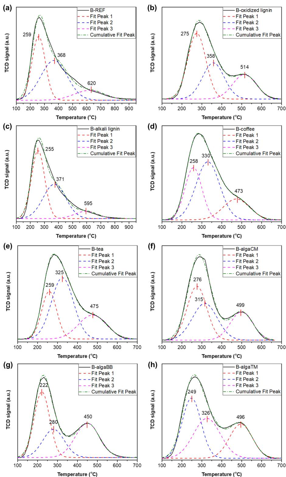
**Figure 3.9** NH<sub>3</sub>-TPD profiles and their corresponding deconvolution peaks into Gaussian peaks (R<sup>2</sup> > 0.99) of B method-ZSM-5 (a) without biomass, and with different biomasses: (b) oxidized lignin, (c) alkali lignin, (d) coffee, (e) tea, (f) algaCM, (g) algaBB, (h)algaTM.
