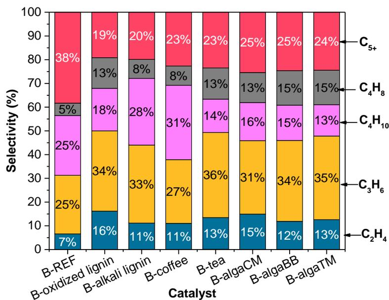
**Figure 4.24** Selectivities in methane, ethylene, propylene, isobutane, butylenes, and C<sub>5</sub><sup>+</sup> hydrocarbons over B-REF and biomass-derived ZSM-5 using B method. Reaction conditions: 450 °C, WHSV = 2 h<sup>-1</sup>, catalyst weight = 60 mg, TOS = 1 h.
