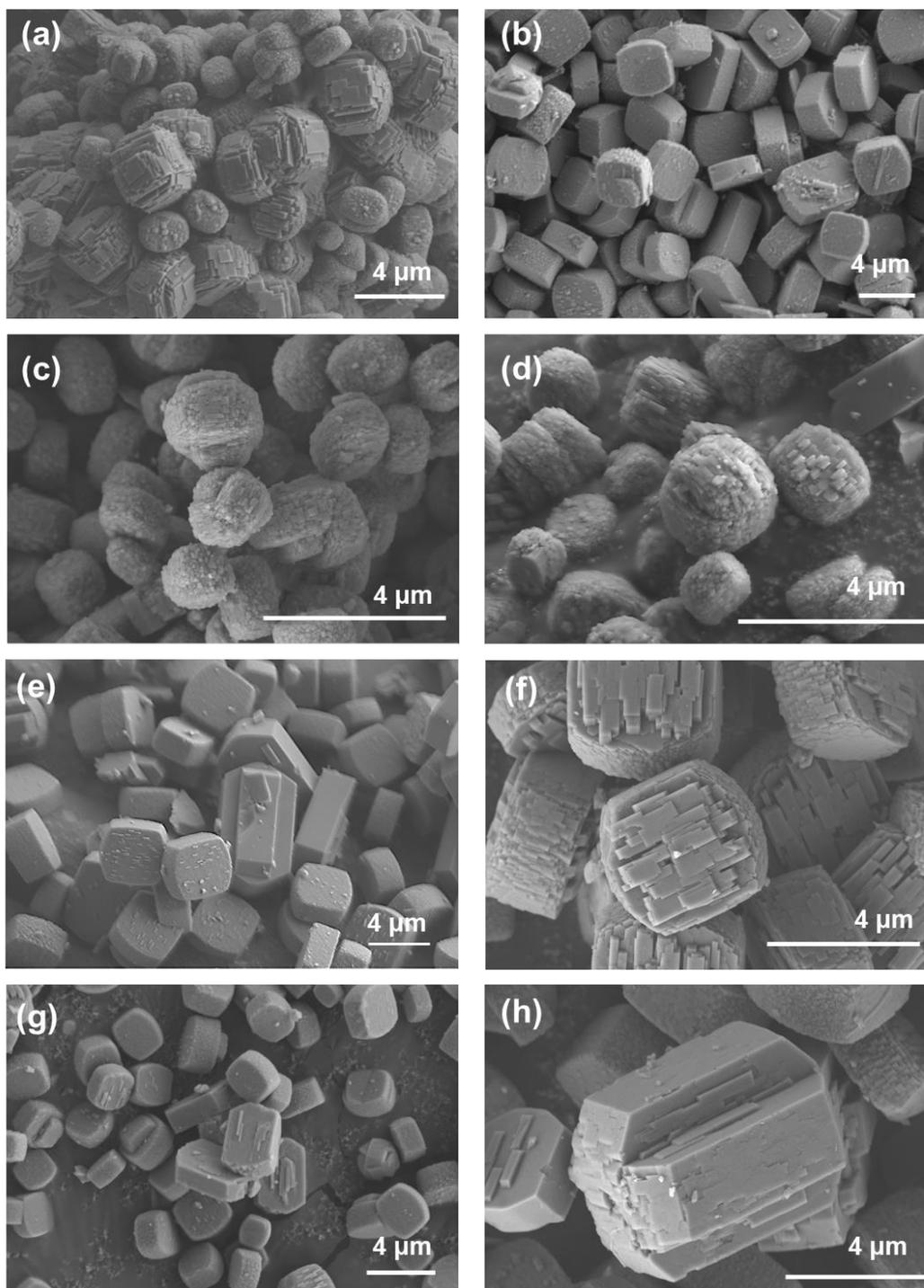
**Figure 3.7** SEM images of (a) B-REF-2d, (b) B-oxidized lignin-2d-300, (c) B-alkali lignin-2d-300, (d) B-coffee-2d-300, (e) B-tea-2d-300, (f) B-algaCM-2d-300, (g) B-algaBB-2d-300, (h) B-algaTM-2d-300.
