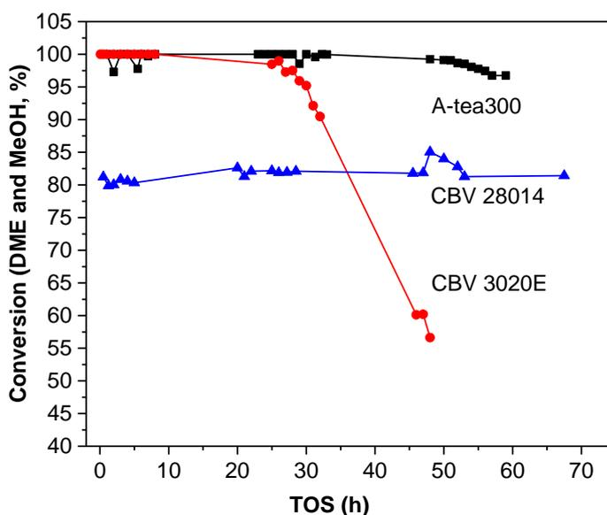
**Figure 4.19** Comparison of methanol (and dimethyl ether) conversion over as-synthesized A-tea300 catalyst and two commercial zeolites (CBV 28014, and CBV 3020E). Reaction conditions: 450 °C, WHSV = 2 h<sup>-1</sup>, catalyst weight = 60 mg.
