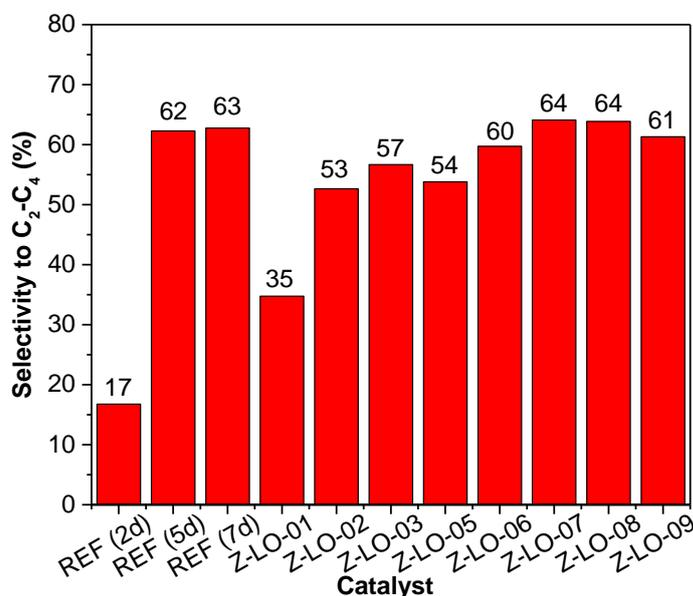
**Figure 4.4** Selectivities in C<sub>2</sub>-C<sub>4</sub> light olefins over different zeolites formed with Z-LO-REF (2d) to Z-LO-REF (7d), and Z-LO-01 to Z-LO-09. Reaction conditions: 450 °C, WHSV = 2 h<sup>-1</sup>, catalyst mass = 60 mg, TOS = 1 h.
