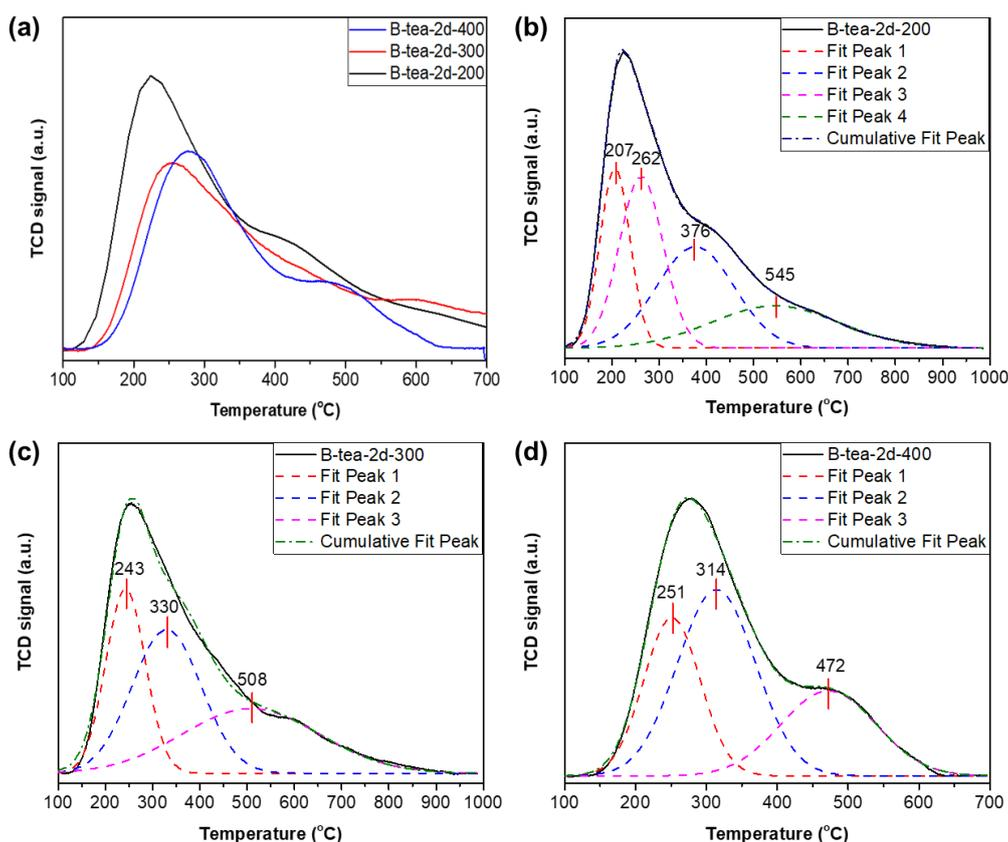
**Figure 3.13**  $\text{NH}_3$ -TPD profiles and their corresponding deconvolution peaks (experiment and fit) of ZSM-5 by B method with different amount of tea waste.
