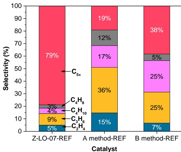
**Figure 4.6** Selectivity in the different products during the methanol conversion over three different zeolites. Reaction conditions: 450 °C, WHSV = 2 h<sup>-1</sup>, catalyst weight = 60 mg, TOS = 1 h.
