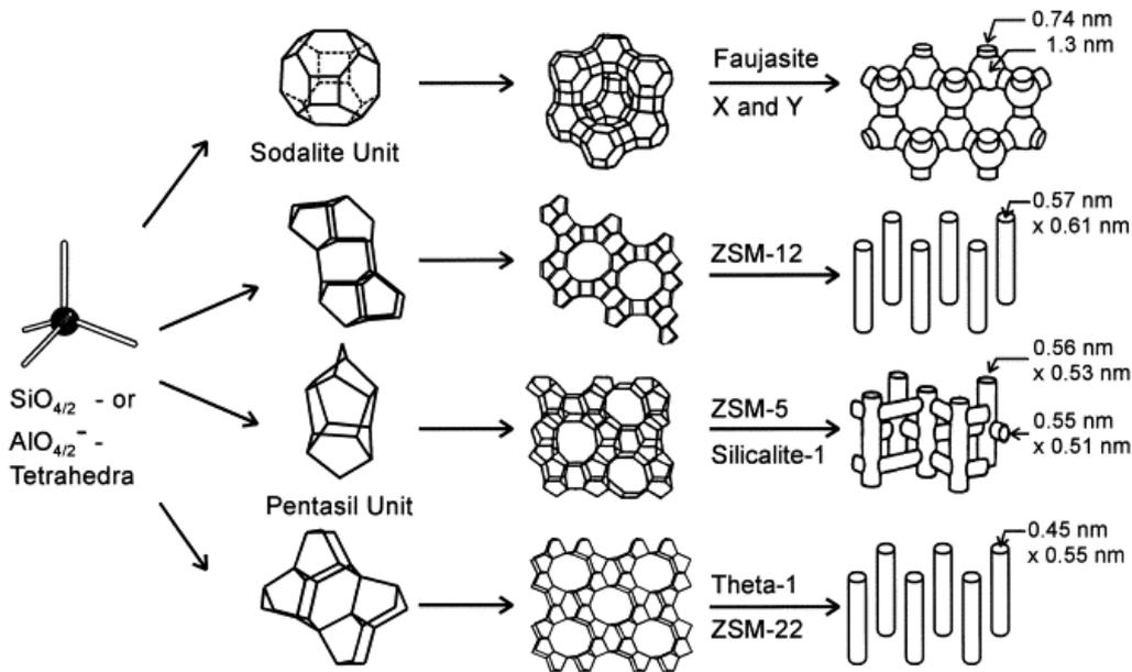
**Figure 1.3** Development of zeolite framework from PBU.
