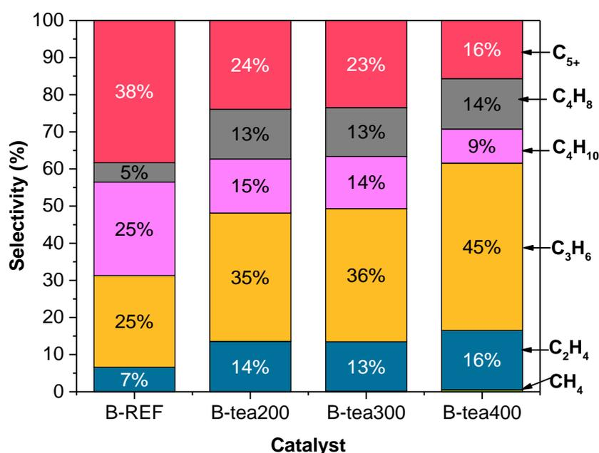
**Figure 4.27** Selectivity distribution of methanol to different hydrocarbons over B-REF and ZSM-5 prepared by B method with different amount of spent tea leaves (200, 300 and 400 mg).
