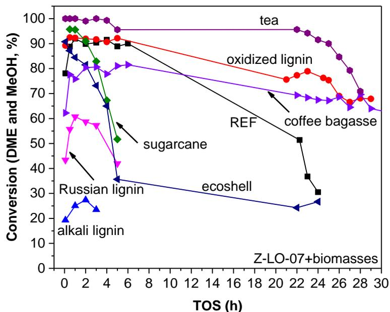
**Figure 4.8** Long term stability in the MTO reaction of as-synthesized ZSM-5 zeolites with 300 mg of various biomasses. Reaction conditions: 450 °C, WHSV = 2 h<sup>-1</sup>, catalyst weight = 60 mg.
