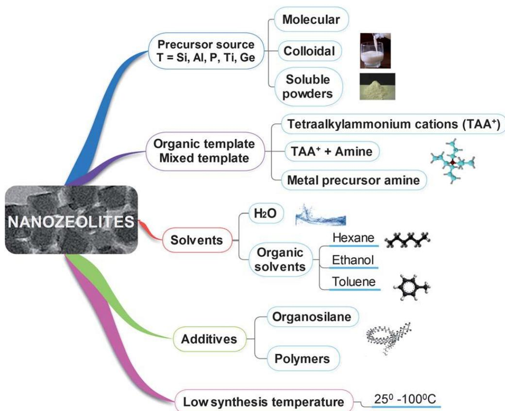
**Figure 1.6** Summary of the key parameters controlling the formation of zeolite frameworks.<sup>75</sup>
