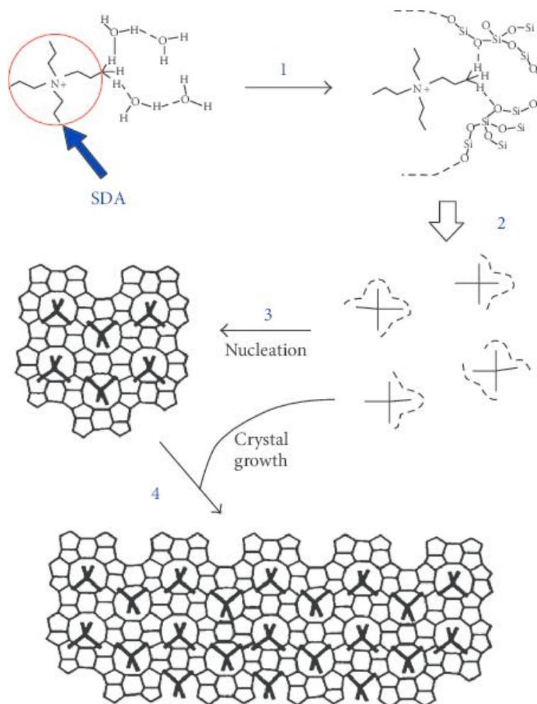
**Figure 1.4** Schematic diagram of the zeolite crystallization mechanism involving TPA<sup>+</sup> as structure-directing agent.<sup>69</sup>
