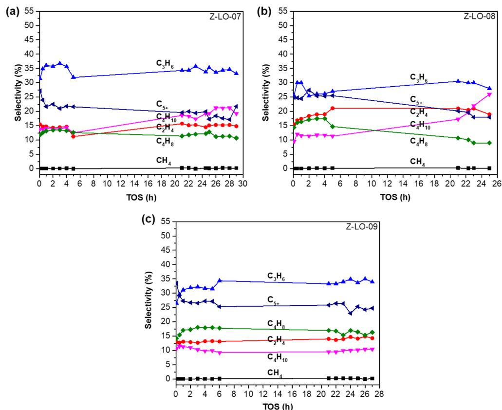
**Figure 4.2** Variation of selectivities towards methane, ethylene, propylene, isobutane, butylenes, and  $C_5^+$  with time-on-stream (TOS) over Z-LO-07, 08 and 09 catalysts. Reaction conditions: 450 °C, WHSV = 2 h<sup>-1</sup>, catalyst weight = 60 mg.
