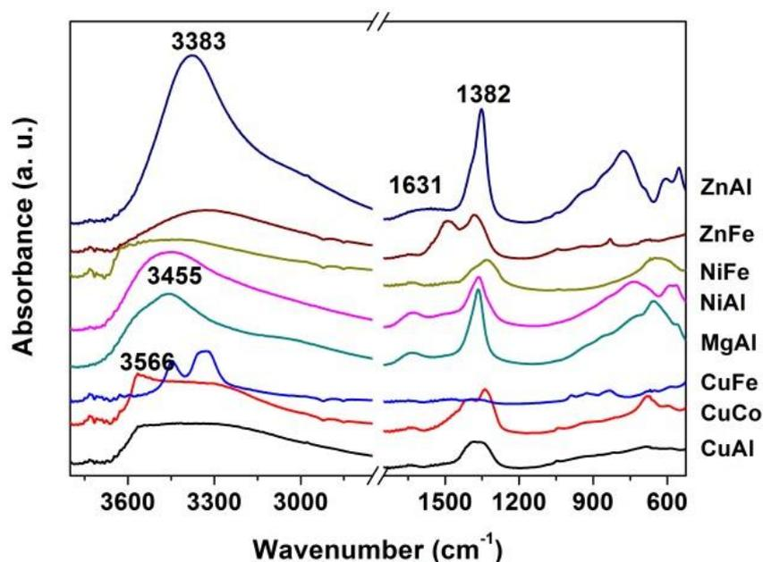
**Figure 6.3** FTIR spectra of as-prepared LDH samples.
