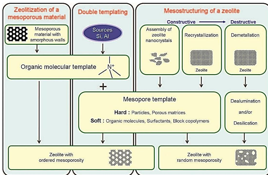
**Figure 1.10** Overview of the various synthesis routes towards zeolite materials combining micro- and mesopores.<sup>93</sup>
