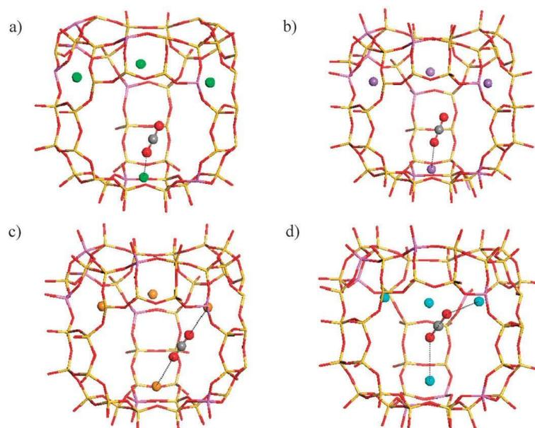
**Figure 1.14** Optimized adsorption mode of one CO<sub>2</sub> molecule in Y zeolite where the CO<sub>2</sub> molecule is oriented towards the supercage: (a) M=Li, (b) M=Na, (c) M=K, (d) M=Cs.<sup>134</sup>
