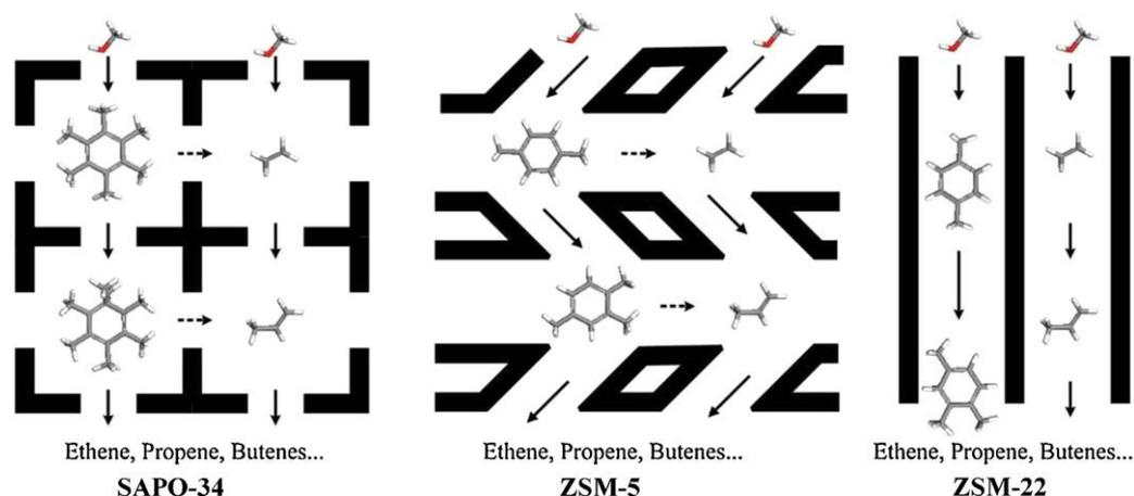
**Figure 1.21** Comparison of reaction routes of methanol conversion over zeolites with different pore structures.
