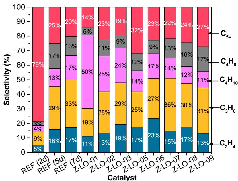
**Figure 4.3** Product distributions during the MTO reaction over Z-LO-REF from 2 to 7 days and ZSM-5 zeolites from Z-LO-01 to Z-LO-09 at 450 °C. Reaction conditions: WHSV = 2 h<sup>-1</sup>, catalyst weight = 60 mg, TOS = 1 h.
