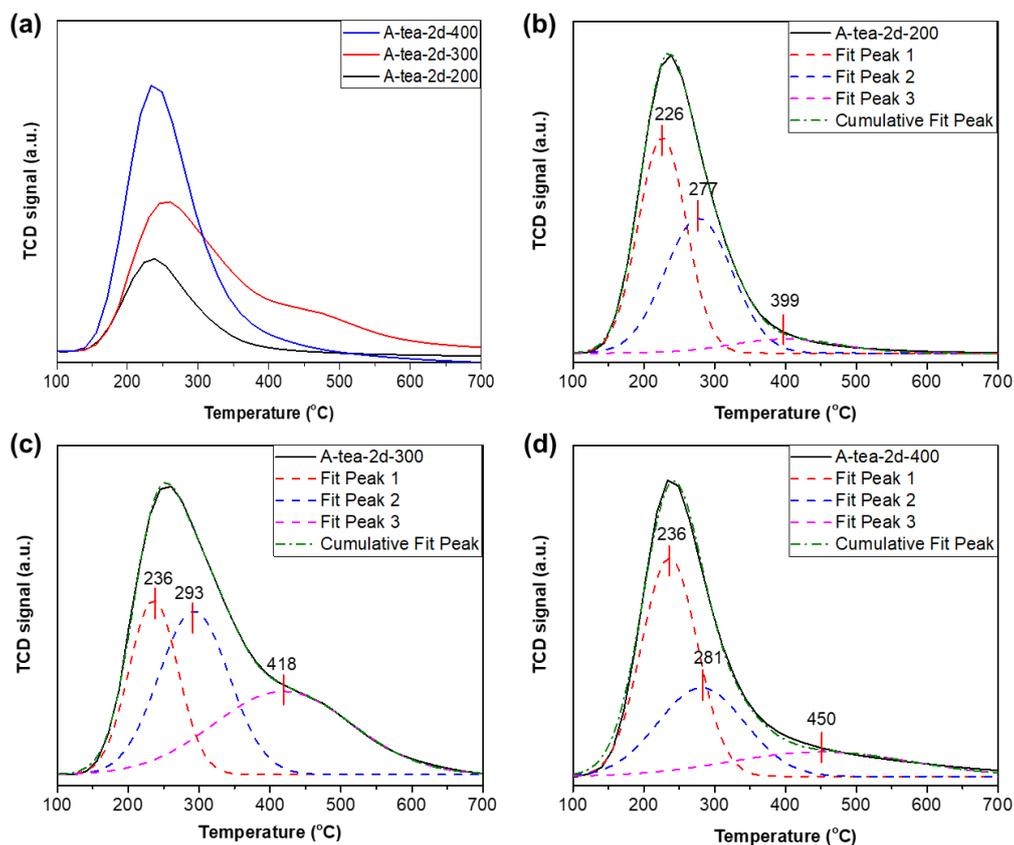
**Figure 3.12** NH<sub>3</sub>-TPD profiles and their corresponding deconvolution peaks into Gaussian peaks ( $R^2 > 0.99$ ) of ZSM-5 by A method with different amount of tea waste.
