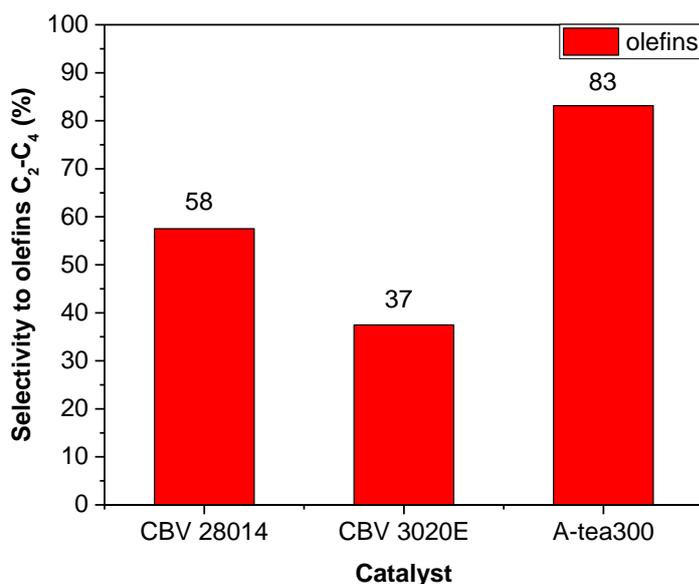
**Figure 4.21** Selectivities towards ethylene, propylene and butylenes over A-tea300 and CBV 28014 and CBV 3020E zeolites at 450 °C.
