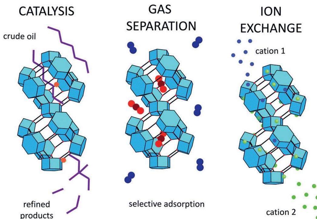
**Figure 1.12** Three main application fields of zeolites in chemical industry.<sup>121</sup>
