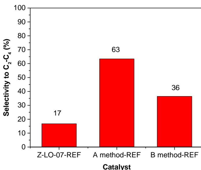
**Figure 4.7** Selectivities to light olefins ( $C_2$ - $C_4$ ) over three reference ZSM-5 catalysts. Reaction conditions: 450 °C, WHSV = 2 h<sup>-1</sup>, catalyst weight = 60 mg, TOS = 1 h.
