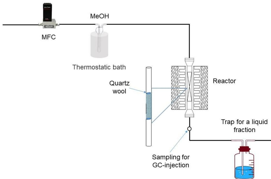
**Figure 2.1** Experimental set-up for the MTO reaction.
