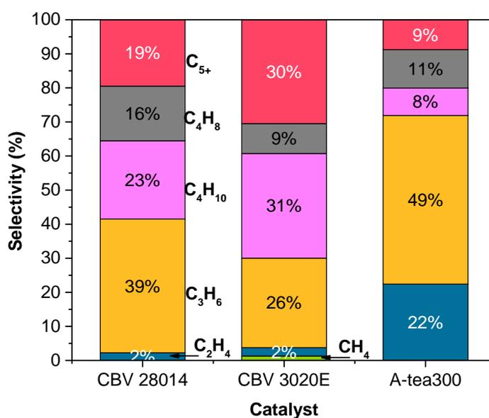
**Figure 4.20** Selectivity in the MTO reaction over A-tea300 zeolites and CBV28014 and CBV 3020E zeolites: 450 °C, WHSV = 2 h<sup>-1</sup>, catalyst weight = 60 mg, TOS = 1 h.
