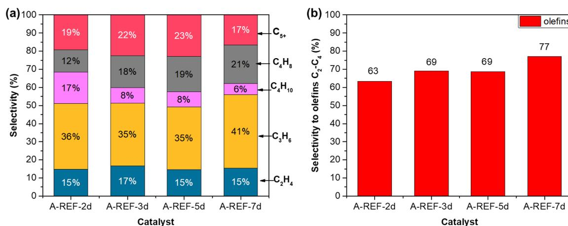
**Figure 4.12** Selectivities towards (a) ethylene, propylene, isobutane, butylenes, and C<sub>5</sub><sup>+</sup> and (b) light olefins (C<sub>2</sub>-C<sub>4</sub>) over catalysts synthesized by A method at different hydrothermal durations (2, 3, 5 and 7 days).
