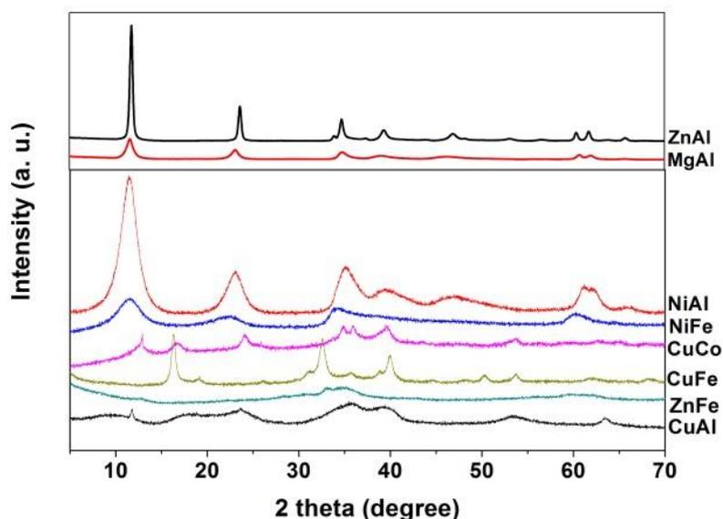
**Figure 6.2** XRD patterns of as-prepared LDH samples.
