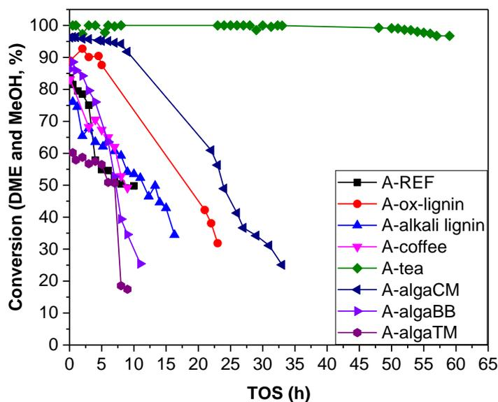
**Figure 4.13** Methanol conversion with time-on-stream over A-REF and different biomasses-derived ZSM-5 by using A method. (biomasses: oxidized lignin, alkali lignin, coffee and tea residue and three kinds of algae).
