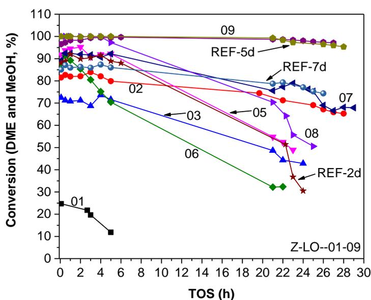
**Figure 4.1** Methanol conversion with time-on-stream over the Z-LO-01 to 09 catalysts prepared with different hydrothermal time and biomass consumption, and three reference zeolites prepared with corresponding time. Reaction conditions: 450 °C, WHSV = 2 h<sup>-1</sup>, catalyst weight = 60 mg.
