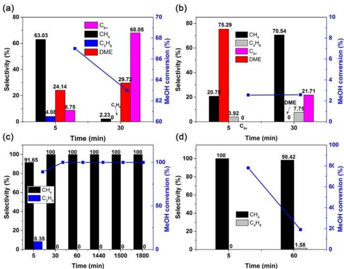
**Figure 6.8** Methanol conversion as well as selectivities towards the different product obtained over LDO catalysts. (a) CuCoO<sub>x</sub>, (b) CuFeO<sub>x</sub>, (c) NiFeO<sub>x</sub> and (d) ZnFeO<sub>x</sub>.
