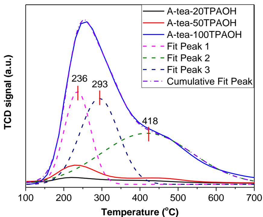
**Figure 3.21** NH<sub>3</sub>-TPD profiles of the tea leaves-assisted ZSM-5 catalysts with different amount of template and the corresponding deconvolution peaks of A-tea-100TPAOH. (Gaussian peaks ( $R^2 > 0.99$ ))
