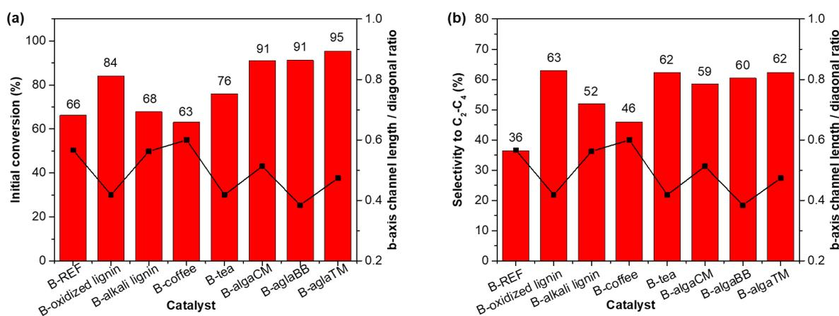
**Figure 5.9** Relationships between (a) initial conversion (1 h TOS) and the b-axis channel length / diagonal ratio, and (b) selectivity toward light olefins (1 h TOS) and the b-axis channel relative length over different catalysts.
