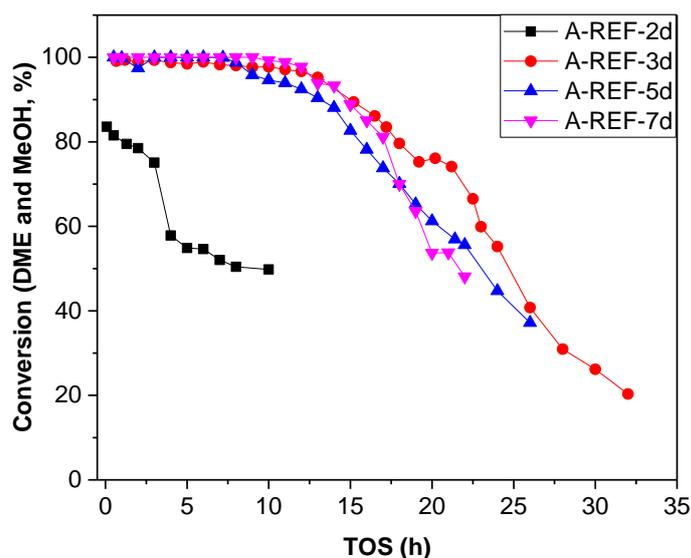
**Figure 4.11** Comparison of methanol conversion results with time-on-stream over ZSM-5 synthesized by A method at different hydrothermal times (2, 3, 5 and 7 days). Reaction conditions: 450 °C, WHSV = 2 h<sup>-1</sup>, catalyst weight = 60 mg.
