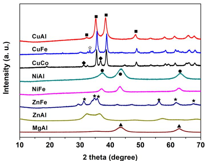
**Figure 6.6** XRD patterns of calcined samples. (■) CuO, (●) NiO, (◆) Cu<sub>0.92</sub>Co<sub>2.08</sub>O<sub>4</sub> (JCPDS 37-0878), (▲) MgAl<sub>2</sub>O<sub>4</sub> (JCPDS 33-0853), (★) ZnO and (☆) Fe<sub>2</sub>O<sub>3</sub>.
