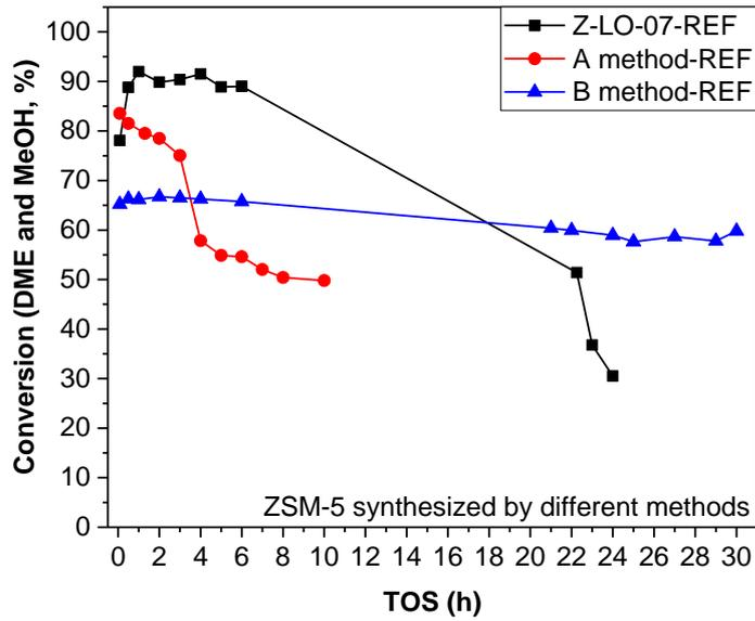
**Figure 4.5** Methanol conversion versus time-on-stream (TOS) over pristine ZSM-5 zeolites synthesized by three different methods. Reaction conditions: 450 °C, WHSV = 2 h<sup>-1</sup>, catalyst weight = 60 mg.
