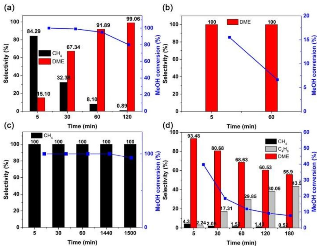
**Figure 6.7** Methanol conversion over LDO catalysts as well as selectivities towards the different products [%] obtained over (a)  $\text{CuAlO}_x$ , (b)  $\text{MgAlO}_x$ , (c)  $\text{NiAlO}_x$  and (d)  $\text{ZnAlO}_x$ .
