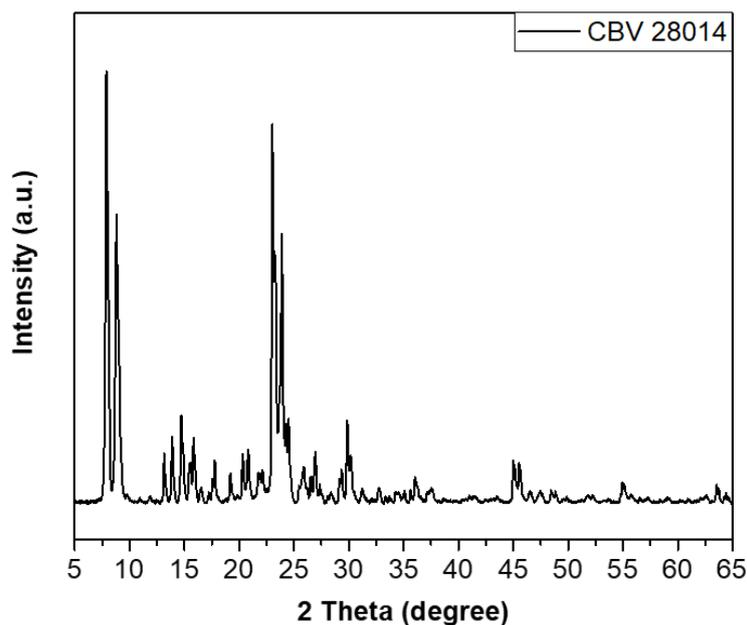
**Figure 3.14** XRD patterns of pristine commercial ZSM-5 zeolite CBV 28014.
