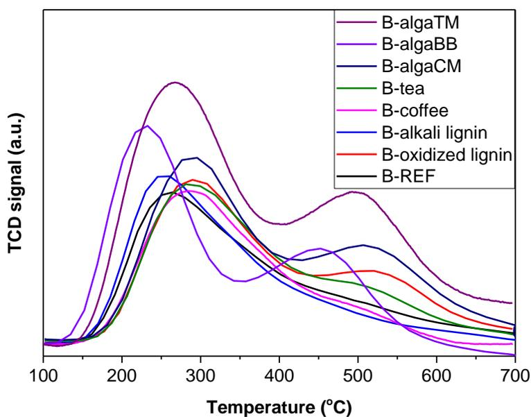
**Figure 3.8** NH<sub>3</sub>-TPD profiles of B method-ZSM-5 catalysts produced with different biomasses.
