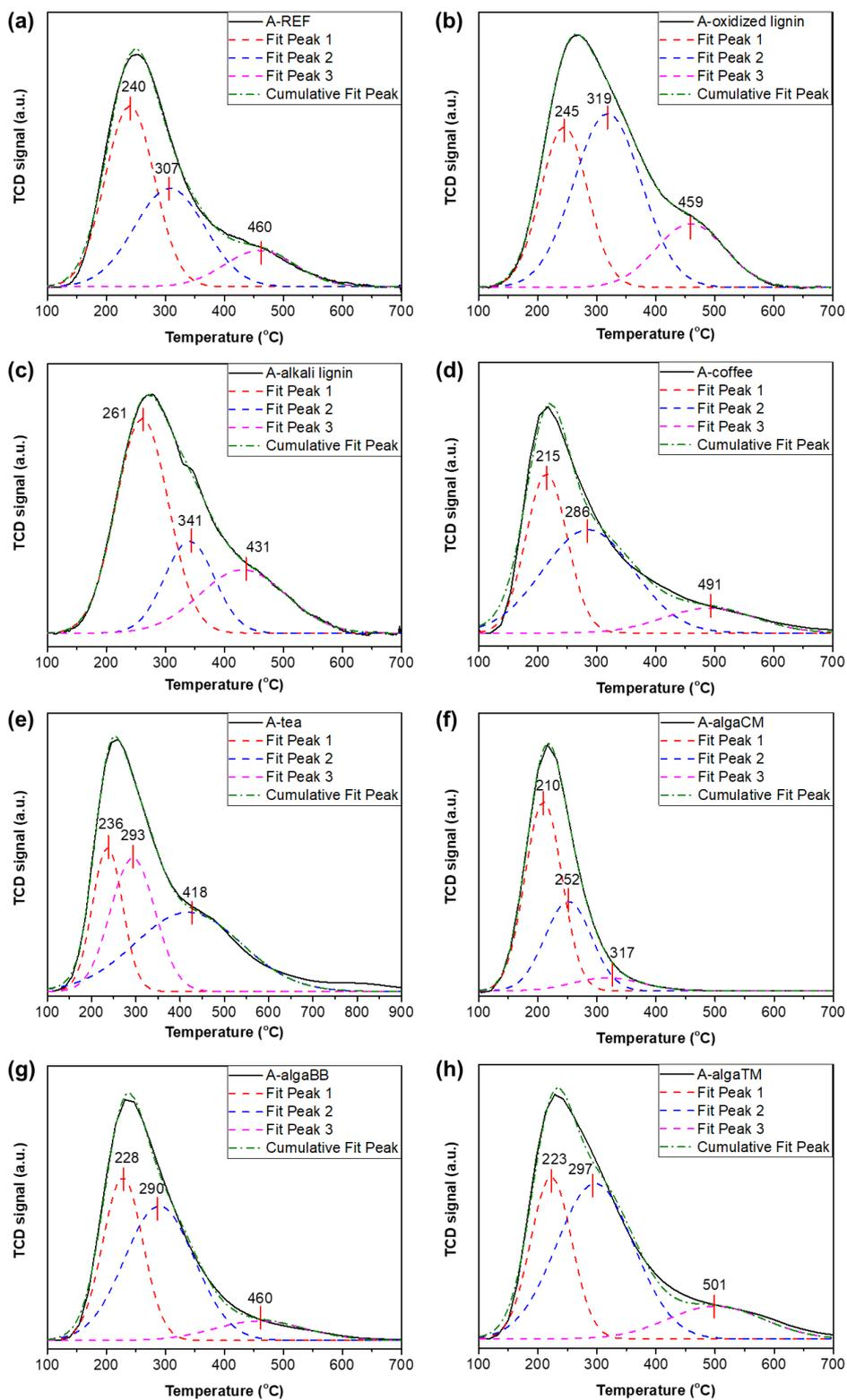
**Figure 3.5**  $\text{NH}_3$ -TPD profiles and their corresponding deconvolution peaks into Gaussian peaks ( $R^2 > 0.99$ ) of A method-ZSM-5 (a) without biomass, and with different biomasses: (b) oxidized lignin, (c) alkali lignin, (d) coffee, (e) tea, (f) algaCM, (g) algaBB, (h) algaTM.
