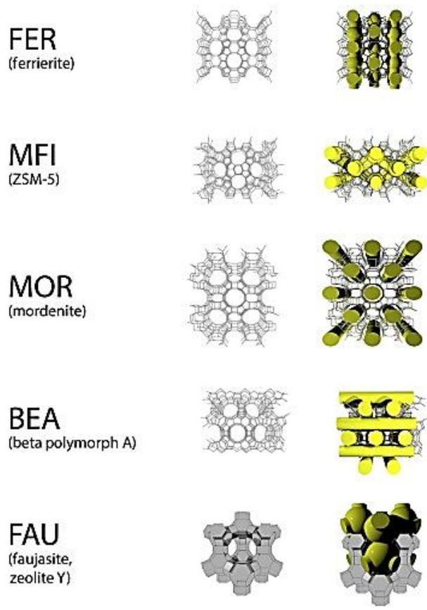
**Figure 1.16** The structures of the Big Five zeolites.<sup>147</sup>
