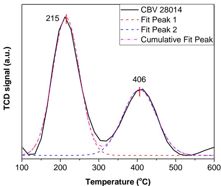
**Figure 3.15** NH<sub>3</sub>-TPD profile and its corresponding deconvolution peaks of commercial CBV 28014 zeolite. (Deconvolution of the NH<sub>3</sub>-TPD curves into Gaussian peaks ( $R^2 > 0.99$ ))
