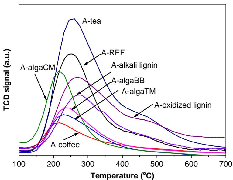
**Figure 3.4** NH<sub>3</sub>-TPD profiles of A method-ZSM-5 catalysts obtained with different biomasses.
