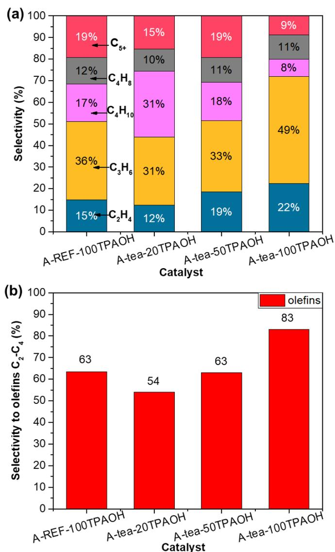
**Figure 4.31** Selectivities in (a) methane, ethylene, propylene, isobutane, butylenes and C<sub>5</sub><sup>+</sup> and (b) C<sub>2</sub>-C<sub>4</sub> light olefins over A-REF-100%TPAOH, A-tea-20%, 50% and 100%TPAOH catalysts. Reaction conditions: 450 °C, WHSV = 2 h<sup>-1</sup>, catalyst weight = 60 mg, TOS = 1 h.
