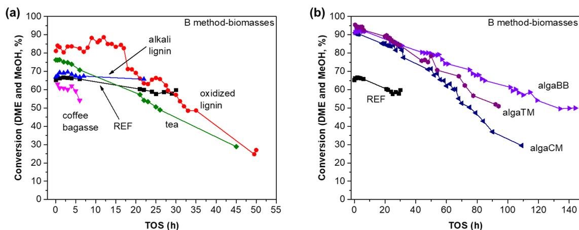
**Figure 4.23** Methanol (and dimethyl ether) conversion over B-REF and ZSM-5 prepared by B method with different kinds of biomasses (oxidized lignin, alkali lignin, coffee and tea residues and three kinds of algae).
