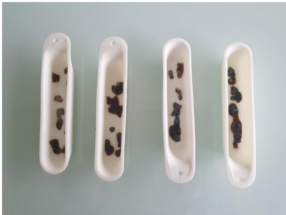
Figure 4.2: Straw melting and reacting with the Alumina crucible (10 cm length, 2 cm width, and 2 cm height) in the pellet test at 1000 °C and 1h.
