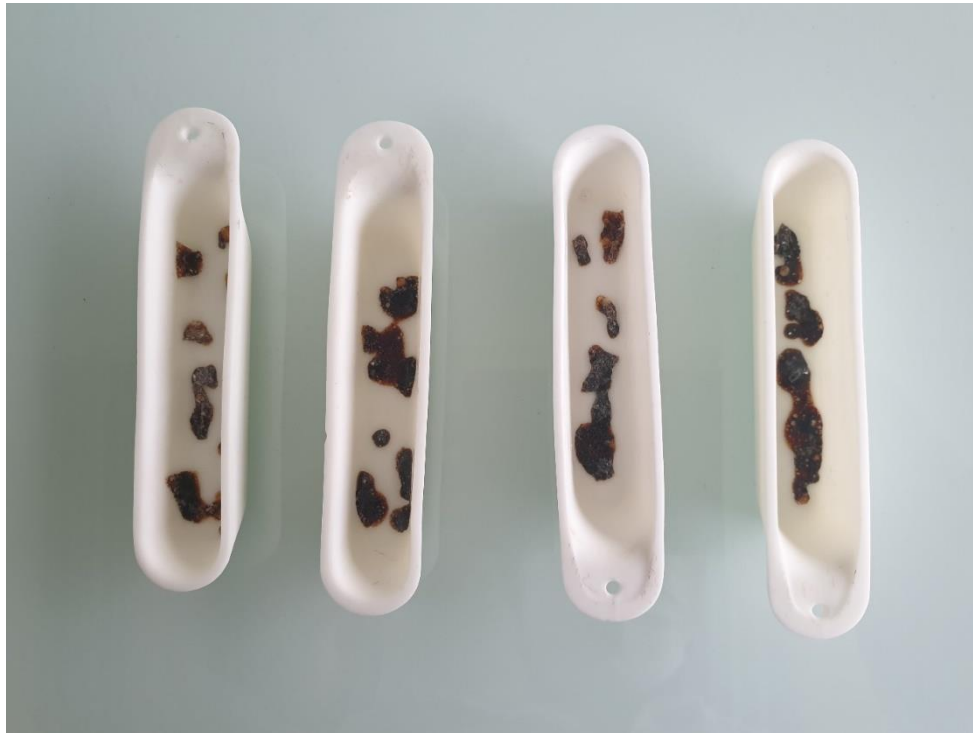
Figure 2.4: Alumina crucible (10 cm length, 2 cm width, and 2 cm height) used in the pellet test.
