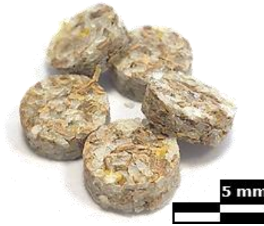
Figure 3-5. Picture of pressed pellets of wood and polyethylene.
