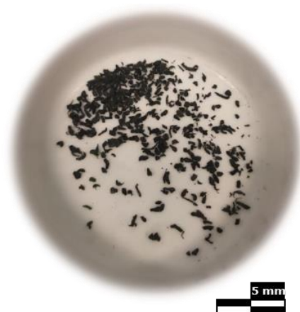
Figure 4-17. Char of the wood/PE mixture after pyrolysis at 800°C.
