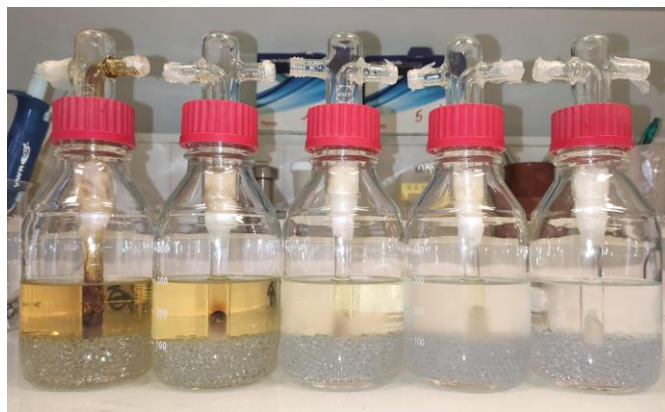
Figure 4-8. Picture of the tar impingers after a pyrolysis test.
