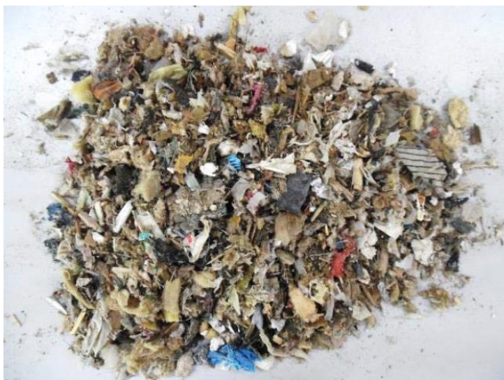
Figure D-1. Photograph of the supplied SRF fluff.
