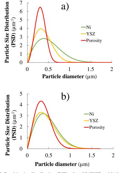
Fig V- 2. Particle size distribution (PSD) of: a) Ni-8YSZ and b) Ni-3YSZ microstructures.
