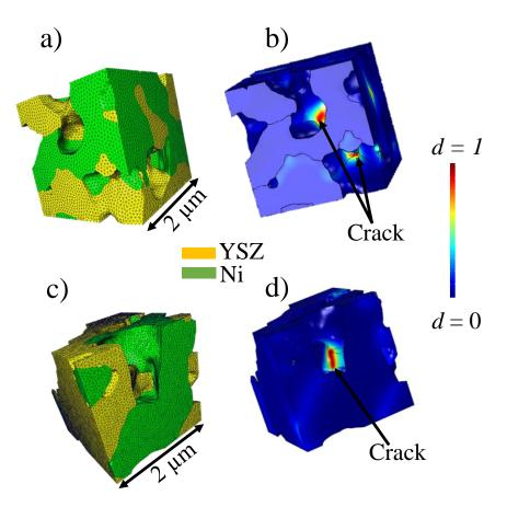
Fig V- 3. Meshes of the simulated Ni-YSZ volumes of 2<sup>3</sup> μm<sup>3</sup>: a) Ni-8YSZ, c) Ni-3YSZ. Micro-cracks simulated by PFM in b) Ni-8YSZ, d) Ni-3YSZ at a critical degree of oxidation of 3% and 11%, respectively.
