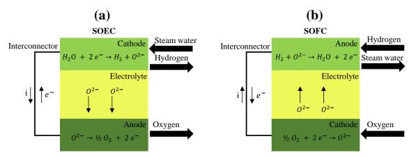
Fig I-1. Operating principle in (a) electrolyzer and (b) fuel cell modes.
