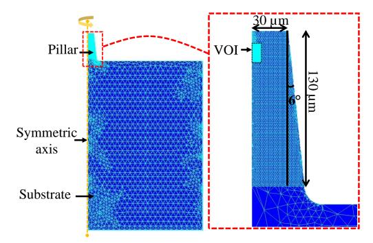
Fig IV- 3. Mesh of the tapered pillar attached to the pellet with axisymmetric conditions. A zoom on the pillar is shown together with the location of the Volume Of Interest (VOI) for the simulation at the microstructure scale using the meshes shown in Fig. IV-2.
