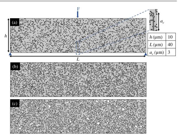
Fig IV- 1. Synthetic porous microstructures with different pore volume fractions ε (solid phase in grey): a) 10%, b) 20%, c) 30%.
