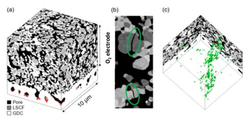
Fig I- 5. (a) LSCF-based O<sub>2</sub> electrode imaged by FIB-SEM serial sectioning after segmentation. (b) Close-up view in the EsB grayscal data showing cracks. (c) 3-D view of the cracks detected in the imaged sample volume [49].
