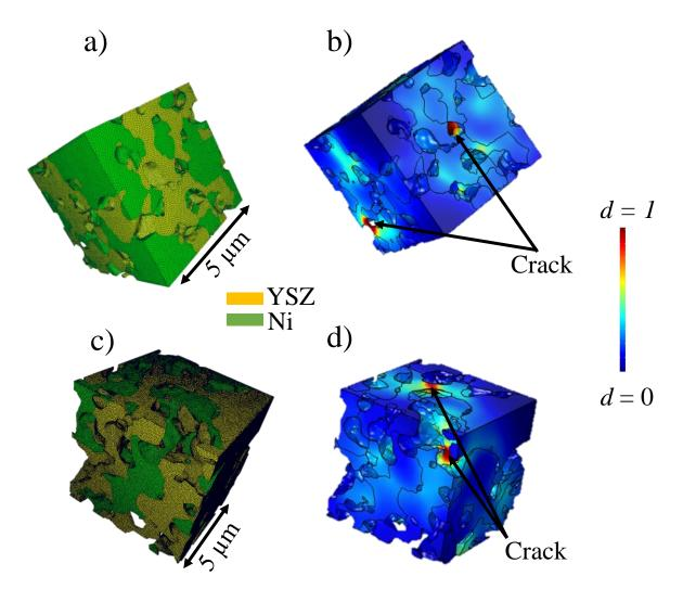
Fig V- 4. Meshes of the simulated solid phases in the Ni-YSZ volumes of  $5^3 \mu m^3$ : a) Ni-8YSZ, c) Ni-3YSZ. Micro-cracks simulated by PFM in b) Ni-8YSZ, d) Ni-3YSZ.
