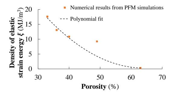
Fig IV- 9. Evolution of the density of elastic strain energy as a function of porosity ( $\ell = 0.8 \ \mu m$ ).
