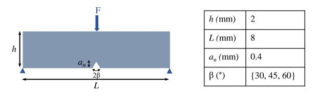
Fig III- 5. Three-point-bending test on a V-notched sample.
