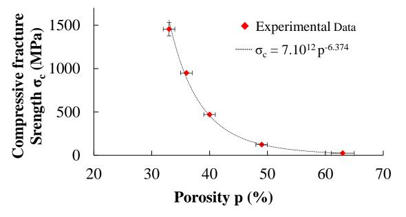
Fig II- 12. Compressive fracture strength as a function of porosity in 8YSZ ceramics, fitted by a power law model.
