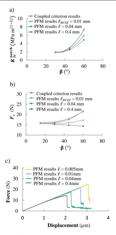
Fig III- 9. Dependence of the mechanical response of the V-notched 8YSZ sample on the opening angle considering different values of the length scale parameter  $\ell$ : a) apparent fracture toughness, b) critical force triggering crack initiation.  $\ell_{8YSZ}$  refers to the length scale parameter that provides close agreement between the coupled criterion and the PFM results over the whole considered range of notch angles, c) force-displacement curves at a V-notch angle 2 $\beta$  of 120°.
