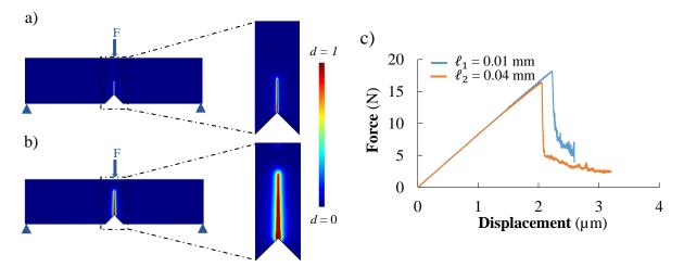
Fig III- 8. Visualization of the crack pattern initiated from a notch at an opening angle  $2\beta$  of 90° for: a)  $\ell_1 = 0.01$  mm, b)  $\ell_2 = 0.04$  mm. c) Force-Displacement curves considering the 8YSZ material at a V-notch angle  $2\beta$  of 90° for  $\ell_1 = 0.01$  mm and  $\ell_2 = 0.04$  mm.
