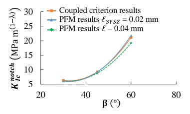
Fig III- 10. Dependence of the apparent fracture toughness on the opening angle for the 3YSZ material considering different values of the length scale parameter  $\ell$ .  $\ell_{3YSZ}$ refers to the length scale parameter that provides close agreement between the coupled criterion and the PFM results over the whole considered range of notch angles.
