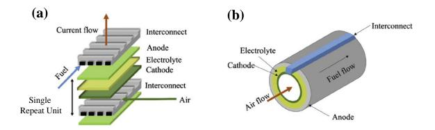
Fig I- 2. Solid Oxide Cell designs: (a) planar and, (b) tubular [11] (illustrated here in SOFC mode with air and fuel supplied to the cell. In this case, the anode and cathode are the H<sub>2</sub> and O<sub>2</sub> electrodes, respectively).
