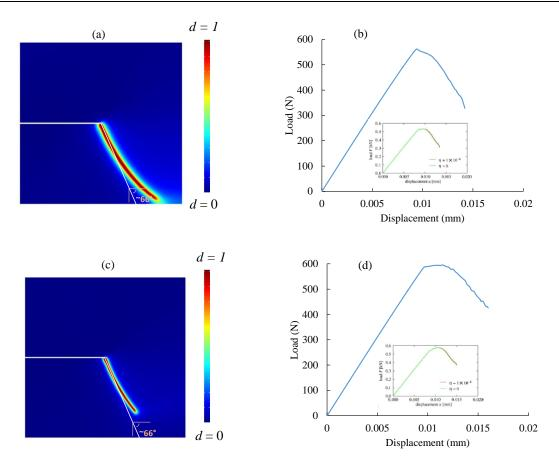
Fig III- 4. Phase field reasults for a single edge notched sample under shear loading: pattern crack with a)  $\ell_1 = 0.015$  mm, c)  $\ell_2 = 0.0075$  mm and load-displacement response with b)  $\ell_1 = 0.015$  mm, d)  $\ell_2 = 0.0075$  mm. The insert in (b) and (d) corresponds to the results reported in Miehe et al. [13].
