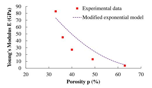
Fig II- 10. Young's modulus as a function of porosity for 8YSZ porous ceramics. Comparison with the modified exponential model proposed in [132] considering a Young's modulus of  $E_0 = 216$  GPa for dense 8YSZ [103] and an intrinsic elastic modulus [E] = 2.2 [132].
