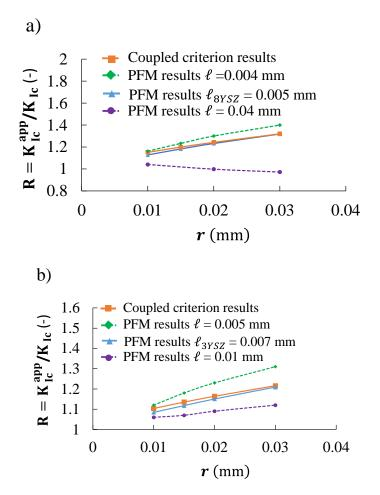
Fig III- 11. The dependence of the relative toughness on the cavity radius considering different values of the length scale parameter  $\ell$  for: a) 8YSZ material, b) 3YSZ material.  $\ell_{8YSZ}$  and  $\ell_{3YSZ}$  refer to the length scale parameters that provide close agreement between the coupled criterion and the PFM results over the whole considered range of cavity radii.
