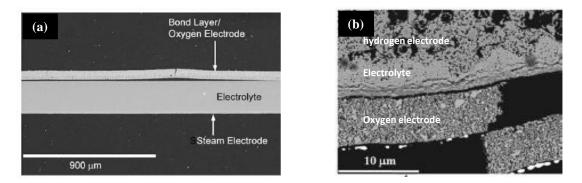
Fig I- 4. Oxygen electrode delamination in an: a) electrolyte-supported cell [35], b) hydrogen electrode-supported cell [39].
