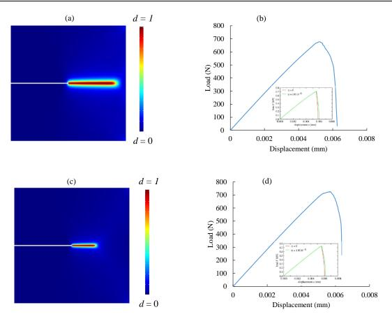
Fig III- 3. Phase field reasults for a single edge notched sample under tensile loading: pattern crack with a)  $\ell_1 = 0.015$  mm, c)  $\ell_2 = 0.0075$  mm and load-displacement response with b)  $\ell_1 = 0.015$  mm, d)  $\ell_2 = 0.0075$  mm. The insert in (b) and (d) corresponds to the results reported in Miehe et al. [13].
