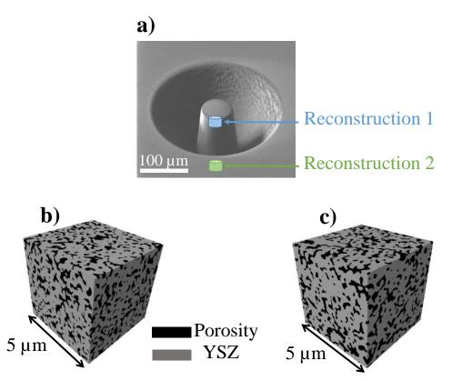
Fig II- 7. FIB-SEM segmented reconstructions of the sample sintered at 1270°C: a) illustration of the two regions of interest, 3D rendering volumes extracted from the whole FIB-SEM reconstructions b) Reconstruction 2: nearby the well in which is the pillar is centered, c) Reconstruction 1: in the pillar.
