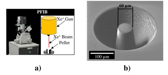
Fig II- 1. Procedure for micro-pillar preparation: a) schematic representation of the Xe<sup>+</sup> pFIB, b) example of a typical specimen obtained after the milling.
