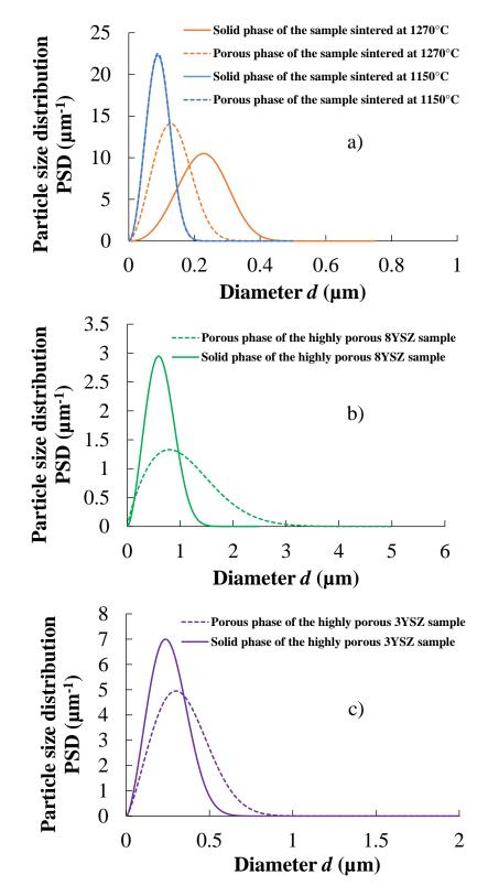
Fig II- 8. Particle size distributions of the solid and porous phases of: a) 8YSZ samples sintered at 1270°C (porosity: 33%) and 1150°C (49%), b) highly porous 8YSZ sample (63%), c) highly porous 3YSZ sample (63%).
