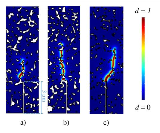
Fig IV- 4. Cartographies displaying crack paths within the porous microstructures: a) first realization at  $\varepsilon$  (porosity) = 20%, b) second realization at  $\varepsilon$  = 20%, c) first realization at  $\varepsilon$  = 10%. ( $\ell_{3YSZ}$  = 0.1 µm).
