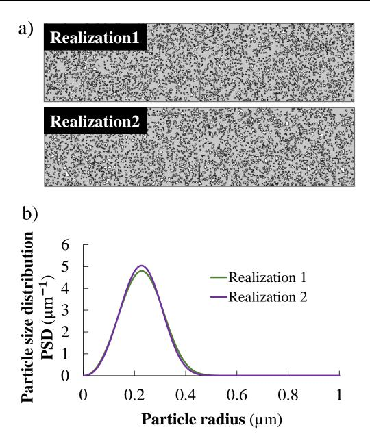
Fig IV- 5. Comparison between two generated synthetic microstructures with  $\varepsilon = 20\%$ : a) visualization of the two realizations of the microstructure, b) Solid phase size distributions (2D) computed on the two realizations.
