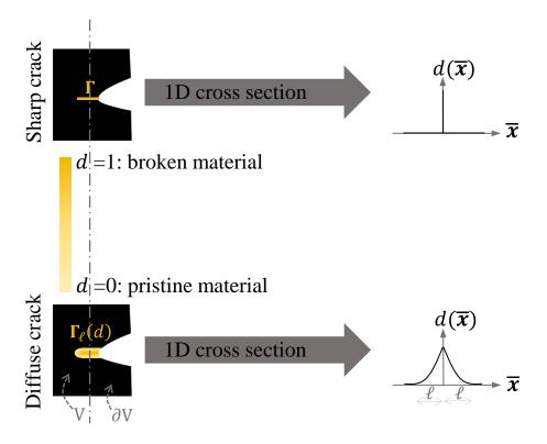
Fig III- 1. Sharp and diffuse crack description.
