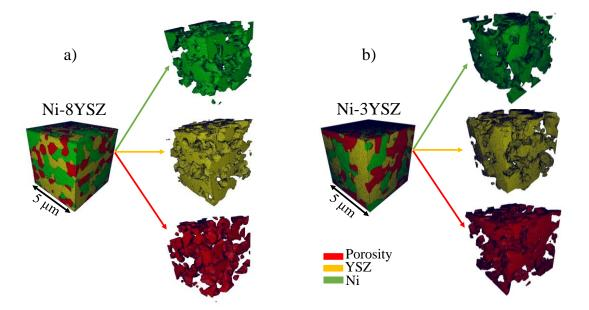
Fig V- 1. Meshes of the computation domain illustrated for the total volume and for each phase separately: a) Ni-8YSZ, b) Ni-3YSZ.
