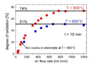
Fig I- 8. Degree of oxidation as a function of air flow rate for two operating temperatures (600°C and 800°C) [40].
