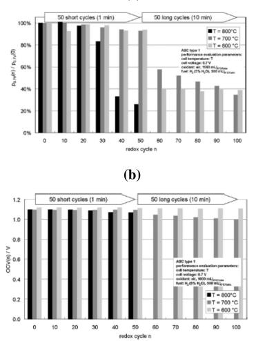
Fig I- 12. Evolution of electrochemical performances of anode-supported cell upon redox cycling for three temperatures (800°C, 700°C and 600°C): a) normalized power density, b) open current voltage [40].
