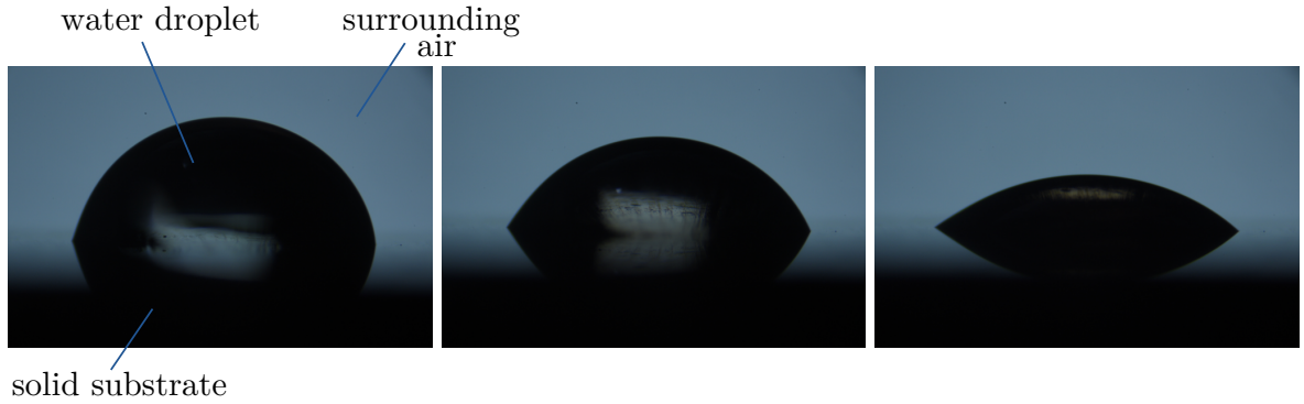
Fig. 3.4 – Example of raw photos of a pinned pure water droplet at different times of the evaporation ( V_0 = 10 \mu\text{L} and RH = 10\% ). The droplet and the solid substrate appear in black and the surrounding air in grey.
