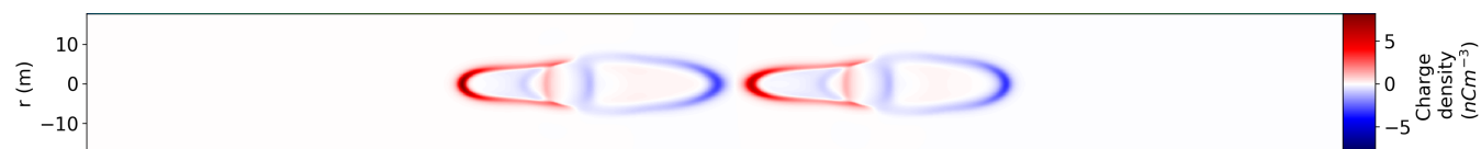
Figure 12: 2-D cross sectional view of the charge density of two double-headed streamers at an altitude of 70 km. The blue color corresponds to a negative net charge while the red color corresponds to an excess positive charge.
