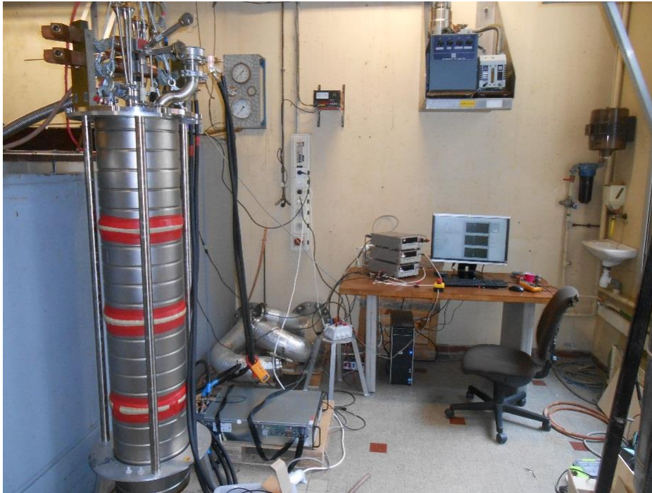
Fig. 98. Experimental set up of a DP test in self-field.
