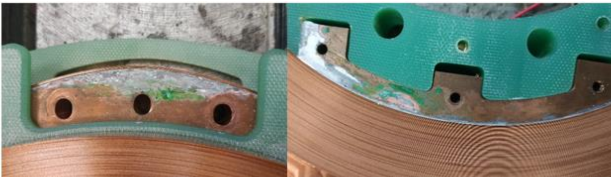
Fig. 110. Solder flux traces (green) on the inner and outer contacts of the DPs.
