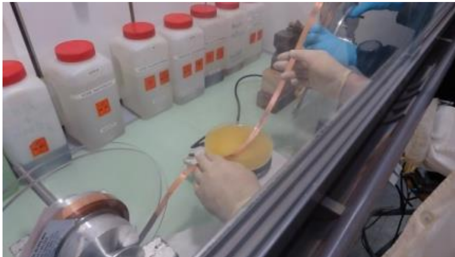
Fig. 90. Conductor de-insulation for soldering contacts.
