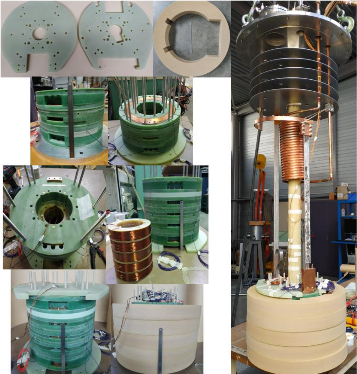
Fig. 124. Photos of the different stages of the solenoid assembly.
