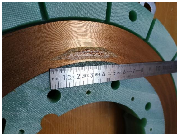
Fig. 115. Visualization of DP damage due to conductor transition.
