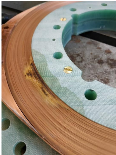
Fig. 38. Melting of the conductor after the appearance of an unprotected hot spot in an REBCO insulated magnet.
