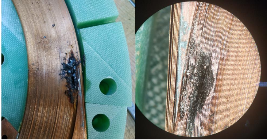
Fig. 122. Melting of the conductor on several turns due to a short circuit causing a hole in the winding.
