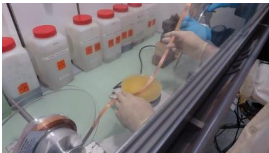
Fig. 90. Conductor de-insulation for soldering contacts.
