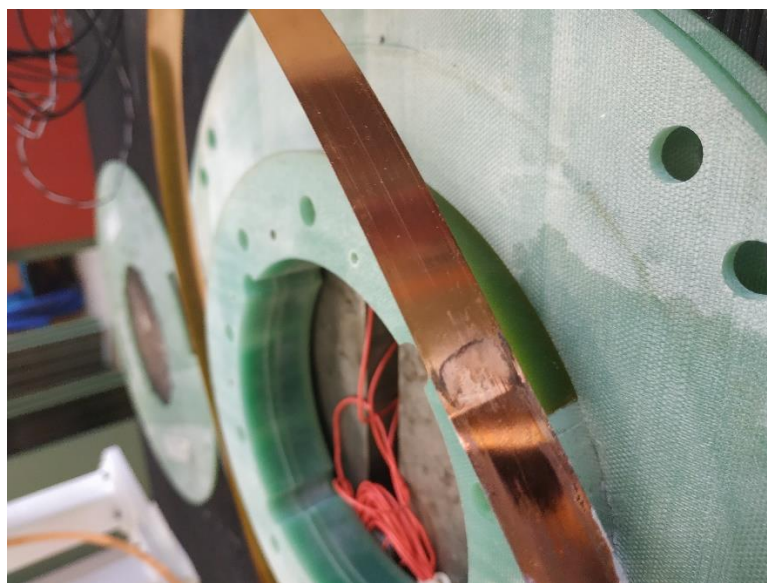
Fig. 113. Pinched conductor at the exit of the inner contact.
