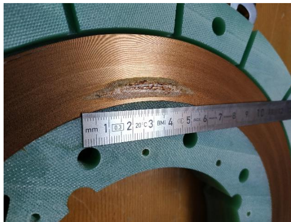
Fig. 115. Visualization of DP damage due to conductor transition.
