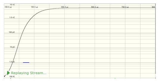
Figure 5-19: Rise time of about 200 µs observed for control signal on Omicron due to low bandwidth of MPD600 (timescale on top)
