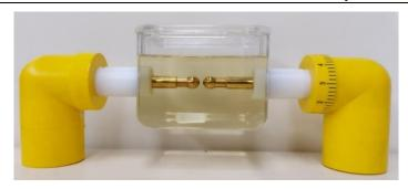
Figure 3-13: Dielectric liquid in Baur cell with sphere-sphere electrodes maintained at 2.5 mm gap
