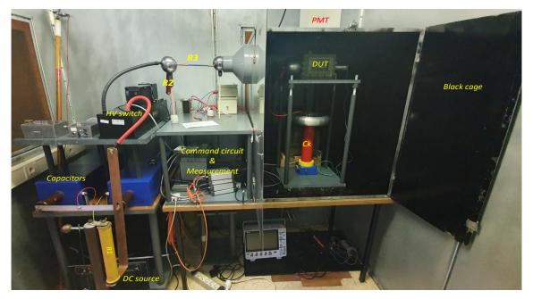
Figure 5-8: Photograph of the square voltage test bench developed in Ampère laboratory, Ecully, France
