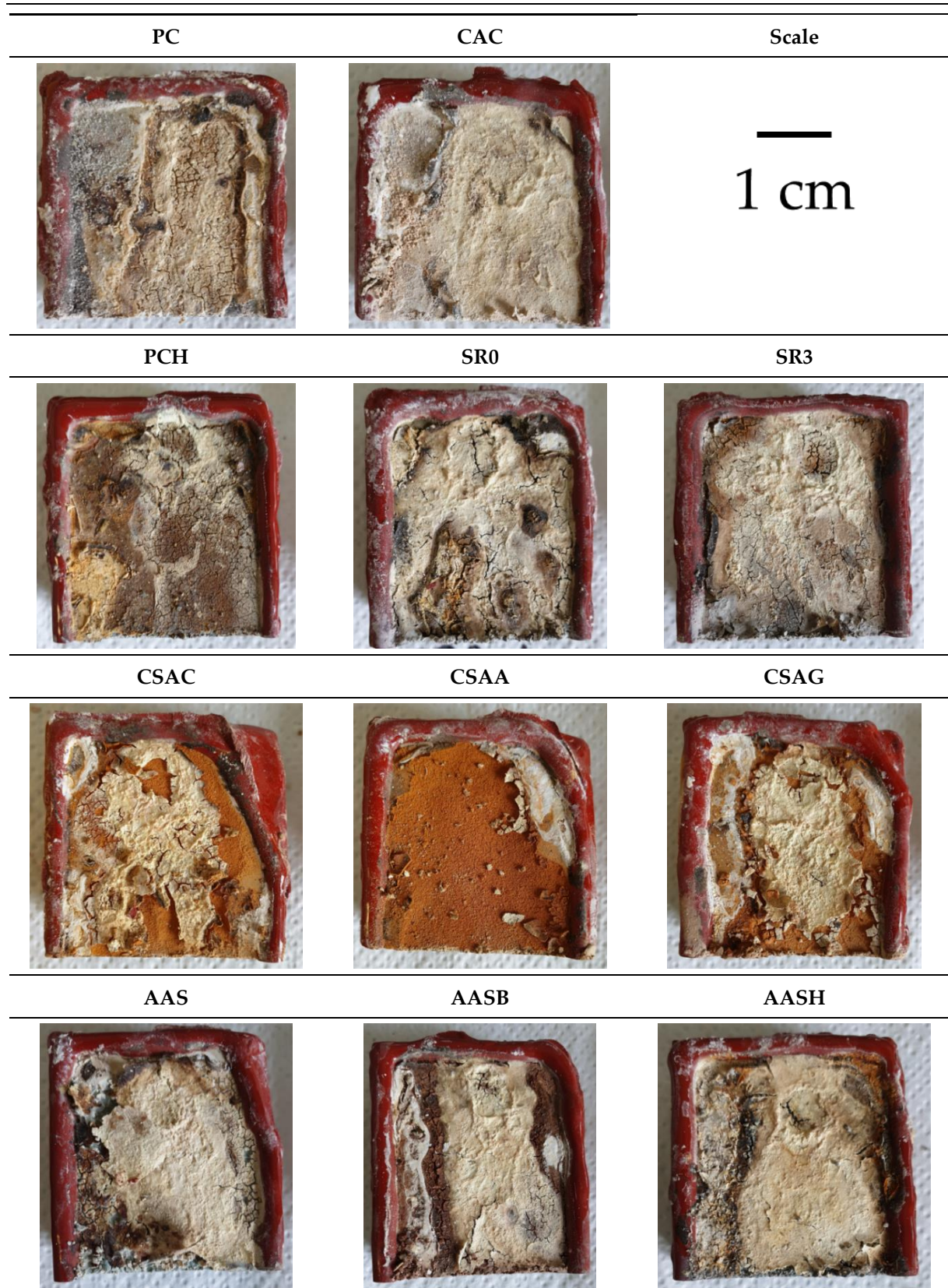
Figure V-1. Visual observations of the deteriorated surface of the different specimens at the end of the exposure period (3 months) to the BAC test
