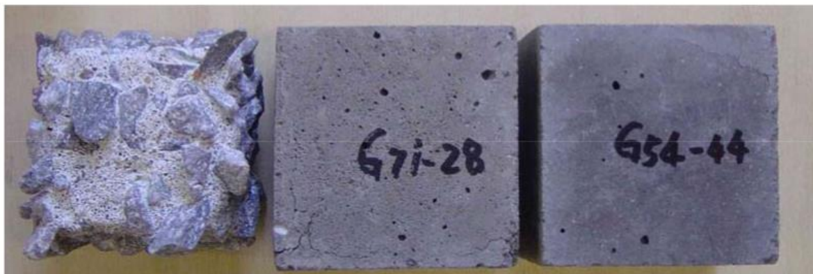
Figure I-43. The concrete specimens exposed to 10% \text{H}_2\text{SO}_4 (Left: Control concrete after 28 days; Middle and Right : FA-based geopolymer concretes after 56 days) [160]
