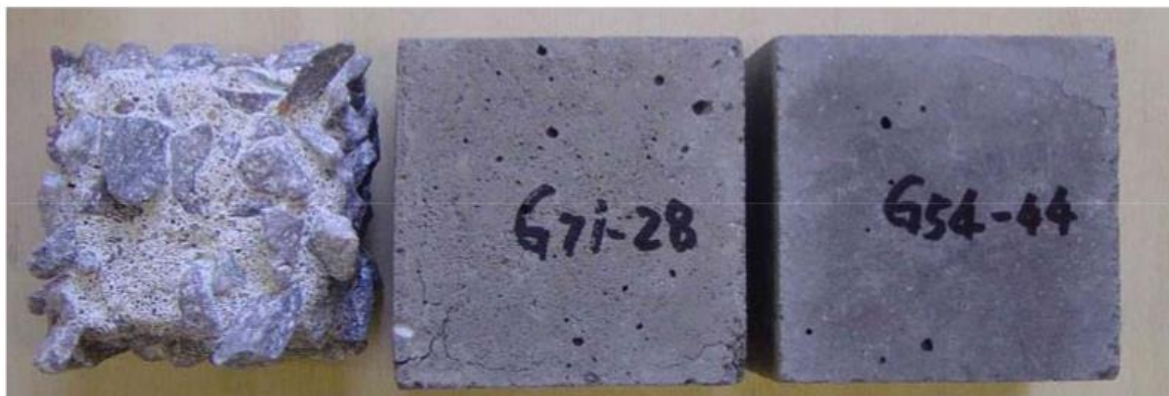
Figure I-43. The concrete specimens exposed to 10% H_2SO_4 (Left: Control concrete after 28 days; Middle and Right : FA-based geopolymer concretes after 56 days) [160]
