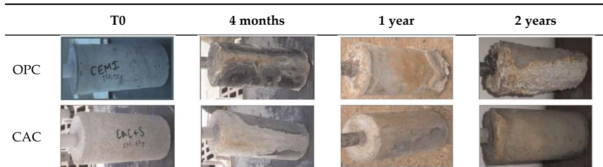
Figure I-10. Observed visual changes on OPC & CAC mortars, unbrushed, over 2 years of exposure in sewage environment [44]
