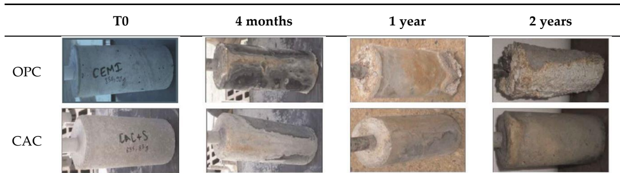
Figure I-10. Observed visual changes on OPC & CAC mortars, unbrushed, over 2 years of exposure in sewage environment [44]
