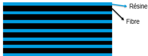
Figure 3-19 Structure du composite 6PN
