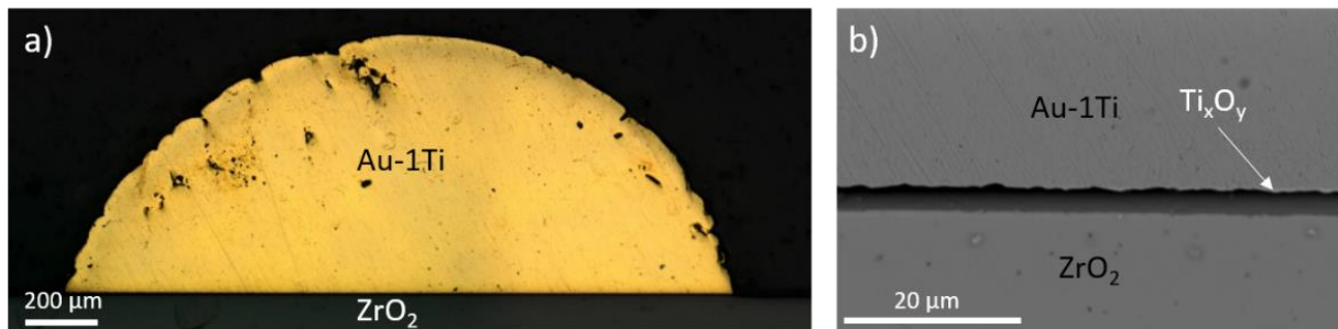
Figure 78: Optical (a) and SEM (b) images of the cross-section of Au-1Ti alloy / polished zirconia sample after an isothermal holding for 10 min at 1170°C (14 min of contact in liquid state).
