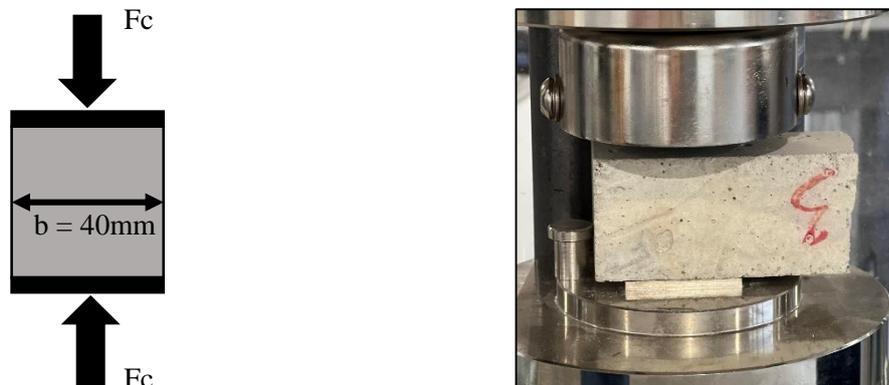
Figure II-24: Essai de compression
