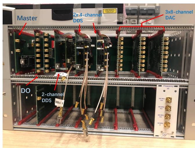
Figure 3.7: A picture of the control rack, the power supply module in the back converts 240VAC into the \pm 15 V power required by the boards and +7 V used to generate the reference level [68]. Each slot can be inserted into a board, and the upper board is in turn: master board, 16-channel digital output board, 2-channel DDS board, 2 \times 4 -channel DDS board, 3 \times 8 -channel boards, the lower empty slot is for the data acquisition board redpitaya. The 100 MHz-500 MHz multiplier at the bottom left is used to generate the synchronization clock for the master board
