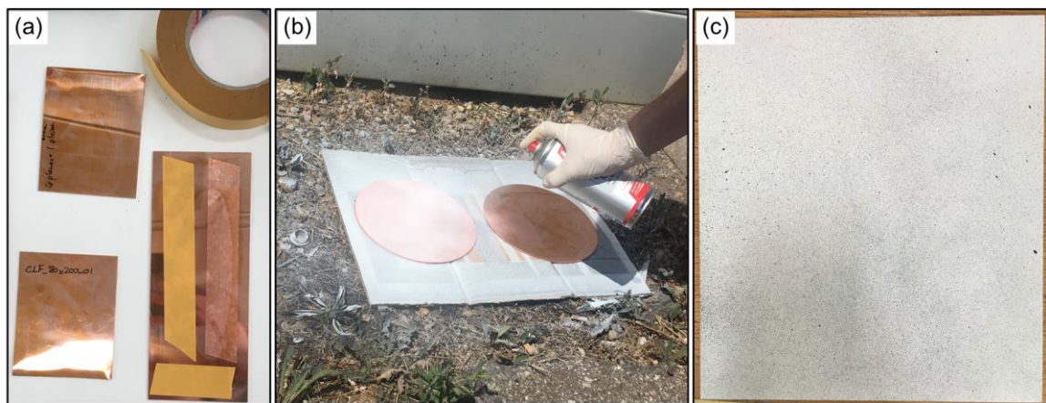
Figure 7.12: Sample preparation before Marciniak tests with (a) sticking a cut blank carrier with a 80 mm x 100 mm blank with double-sided tape, (b) painting of a circular blank with the matte white paint, and (c) the resulting stochastic pattern for DIC made with black paint speckles.
