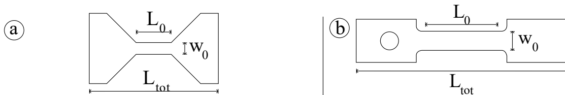
Figure 3.12: Tensile specimen geometry and main dimensions for all tests performed on niobium single crystals. Specimen (b) was used in two different configurations, with or without the hole shown on the left side.
