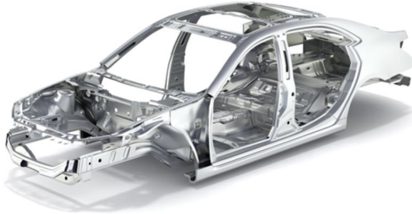
Figure 1.7: Car chassis showing assembled structural sheet–metal parts [43].
