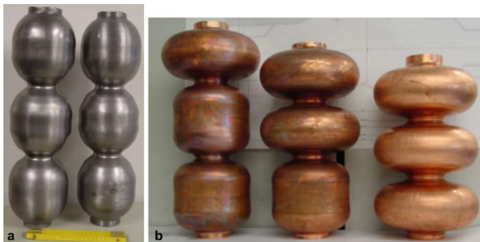
Figure 1.13: (a) niobium tubes deformed after the necking step and (b) copper tubes at different stages of the 1.3 GHz 3-cell fabrication at DESY [68].
