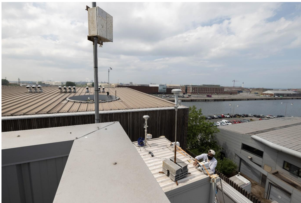
Figure 2-6. View of the shelter in which all the instruments are installed for monitoring. The sampling heads used respectively for the TRAPS, the Beta gauge “MP101” are shown together with the meteorological station. (Credit: Marc Fourmentin).
