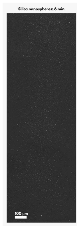
Figure 3-12. TSEM images (Magnification: 25 \times , Accelerating voltage: 15 kV) of the coarse stage samples showing silica microspheres collected for 6 min.
