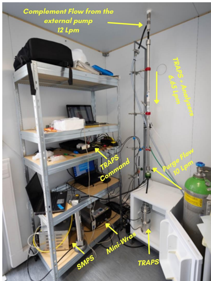
Figure 2-8. Image showing the instruments used for in-situ characterisation of particles during the MIXTAPE campaign. The TRAPS is set inside a fridge (+4°C). Other instruments installed in the shelter such as the SMPS (TSI Inc.), the Optical Particle Counter (OPC) Mini-Wras (Grimm TM ) and the aethalometer AE55 (Mc Gee Scientific) were connected to the same sampling line. (Credit: Marc Fourmentin)
