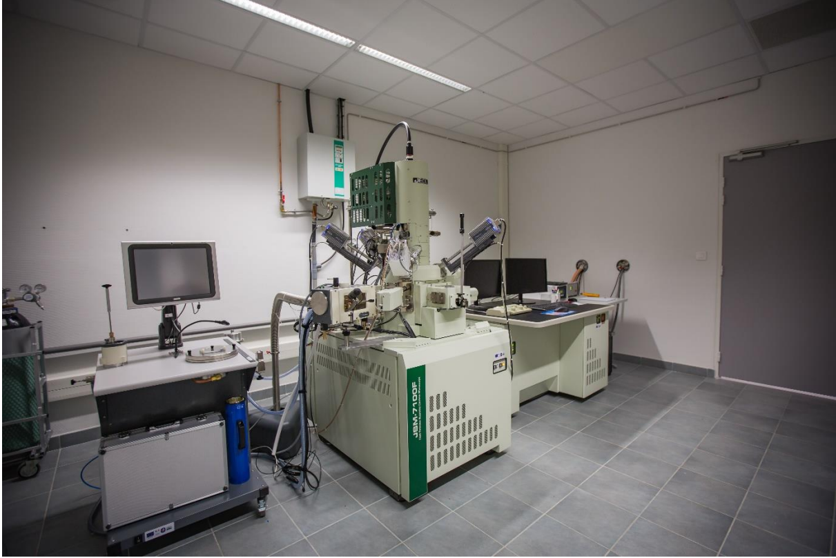
Figure 2-11. Image of the FEG-SEM model JEOL JSM-7100F located inside the IRENE-ULCO research building. (Credit: Marc Fourmentin)
