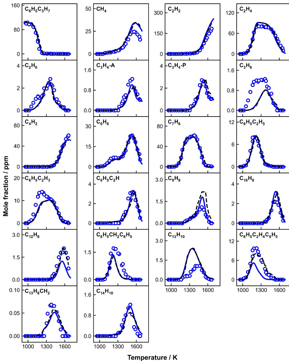
**Figure 5.90:** Species mole fractions as a function of  $T_s$  in *n*-propylbenzene pyrolysis. Symbols: measurements; solid lines: modeling results at constant 20 bar within a fixed reaction time of 4.0 ms; dashed lines: simulations with measured pressure profiles up to a time scale of 10 ms.
