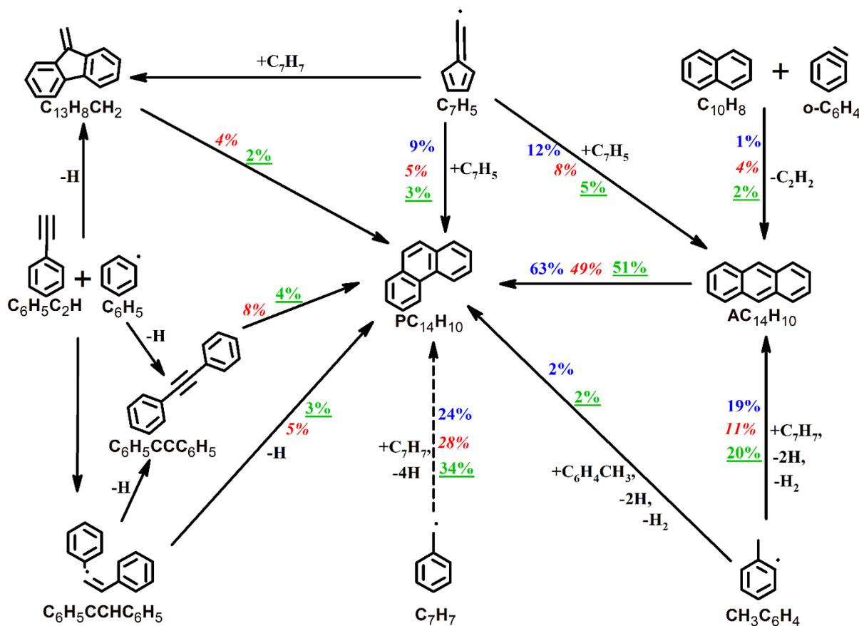
**Scheme 5.13:** Formation pathways for PC<sub>14</sub>H<sub>10</sub> and AC<sub>14</sub>H<sub>10</sub> in the pyrolysis of neat toluene and toluene-propylene and toluene-propyne mixtures at T<sub>5</sub> of 1500 K. The percentage numbers (normal: neat toluene; italic: toluene+propylene; underlined: toluene+propyne) represent the contributions of corresponding reactions to the formation of C<sub>14</sub>H<sub>10</sub> PAHs. The dashed lines represent multiple step reaction processes
