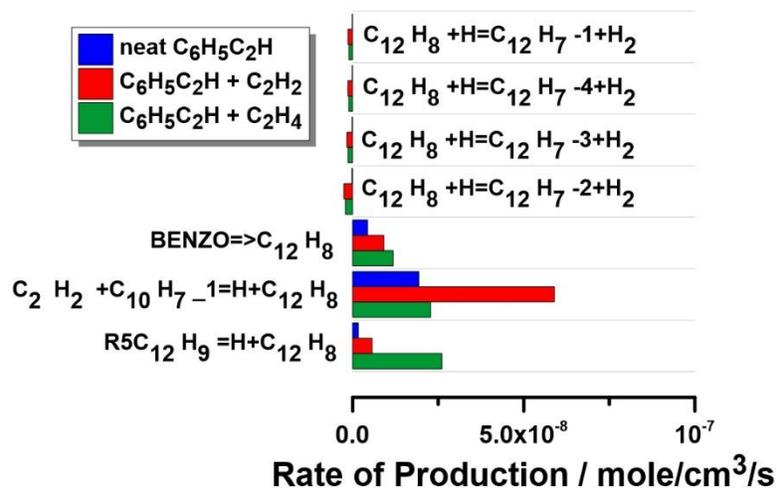
**Figure 5.81:** ROP analysis for C<sub>12</sub>H<sub>8</sub> production at T<sub>5</sub> = 1500 K, P<sub>5</sub> = 20 bar and reaction time = 4ms in the pyrolysis of neat C<sub>6</sub>H<sub>5</sub>C<sub>2</sub>H, C<sub>6</sub>H<sub>5</sub>C<sub>2</sub>H+C<sub>2</sub>H<sub>2</sub> and C<sub>6</sub>H<sub>5</sub>C<sub>2</sub>H+C<sub>2</sub>H<sub>4</sub>.
