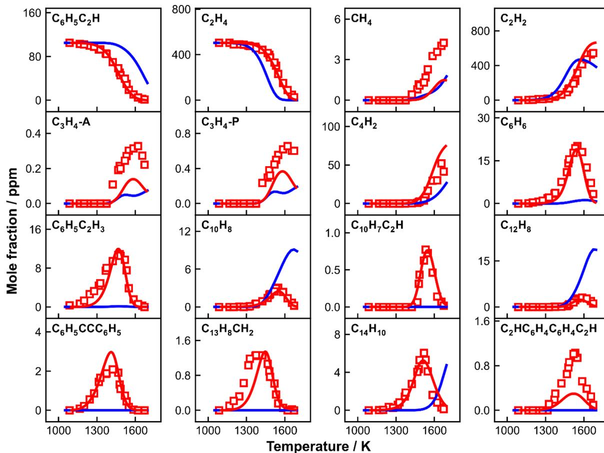
**A 17:** Measured (symbols) and simulated (lines) species mole fraction profiles as a function of  $T_5$  in 105 ppm phenylacetylene+ 504 ppm ethylene co-pyrolysis. Thick solid red lines: simulations using the current kinetic model with the constant  $p_5$  of 20 bar and the nominal reaction time of 4 ms; thick solid blue line: simulations using CRECK model with the constant  $p_5$  of 20 bar and the nominal reaction time of 4 ms.
