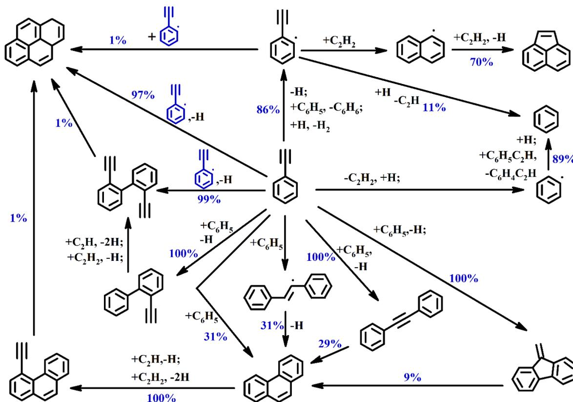
**Scheme 5.14:** The reaction pathways leading to the PAH formation at  $T_5$  of 1450 K in neat phenylacetylene pyrolysis.. The percentage numbers represent the contributions of the corresponding reactions in the formation of PAH species.
