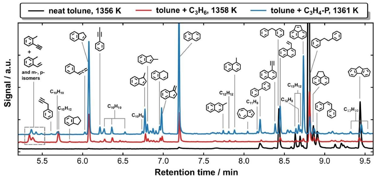
**Figure 3.12:** GC signals recorded in neat toluene, toluene + propylene (C<sub>3</sub>H<sub>6</sub>) and toluene + propyne (C<sub>3</sub>H<sub>4</sub>-P) pyrolysis at T<sub>5</sub> around 1360 K [141].
