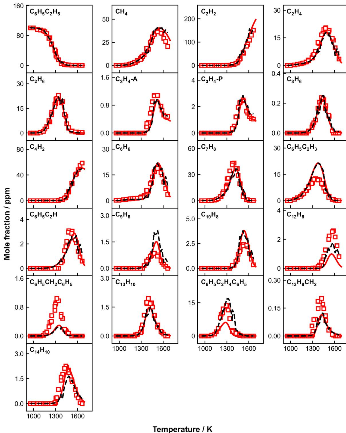
**Figure 5.89:** Species mole fractions as a function of  $T_5$  in ethylbenzene pyrolysis. Symbols: measurements; solid lines: modeling results at constant 20 bar within a fixed reaction time of 4.0 ms; dashed lines: simulations with measured pressure profiles up to a time scale of 10 ms.
