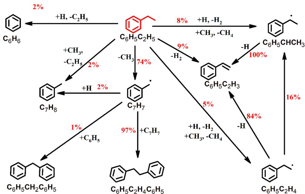
**Scheme 5.15:** Fuel consumption pathways in ethylbenzene pyrolysis based on integrated ROP analysis at 1250 K. The percentage numbers are the contributions by the corresponding reactions to the consumption of the species on the source side.
