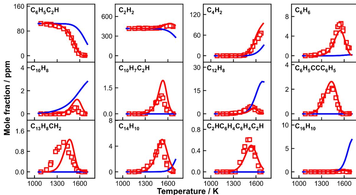
**A 16:** Measured (symbols) and simulated (lines) species mole fraction profiles as a function of  $T_5$  in 104 ppm phenylacetylene+ 415 ppm acetylene co-pyrolysis. Thick solid red lines: simulations using the current kinetic model with the constant  $p_5$  of 20 bar and the nominal reaction time of 4 ms; thick solid blue line: simulations using CRECK model with the constant  $p_5$  of 20 bar and the nominal reaction time of 4 ms.
