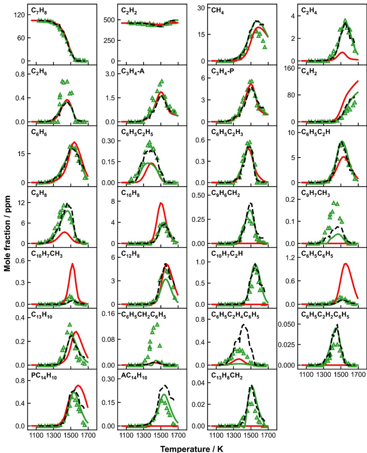
**A 11:** Measured (symbols) and simulated (lines) species mole fraction profiles as a function of  $T_5$  in 105 toluene+ 459 ppm acetylene co-pyrolysis. Thick solid green lines: simulations using the current kinetic model with the constant  $p_5$  of 20 bar and the nominal reaction time of 4 ms; thick dashed black lines: simulations using the current model with measured pressure profiles up
