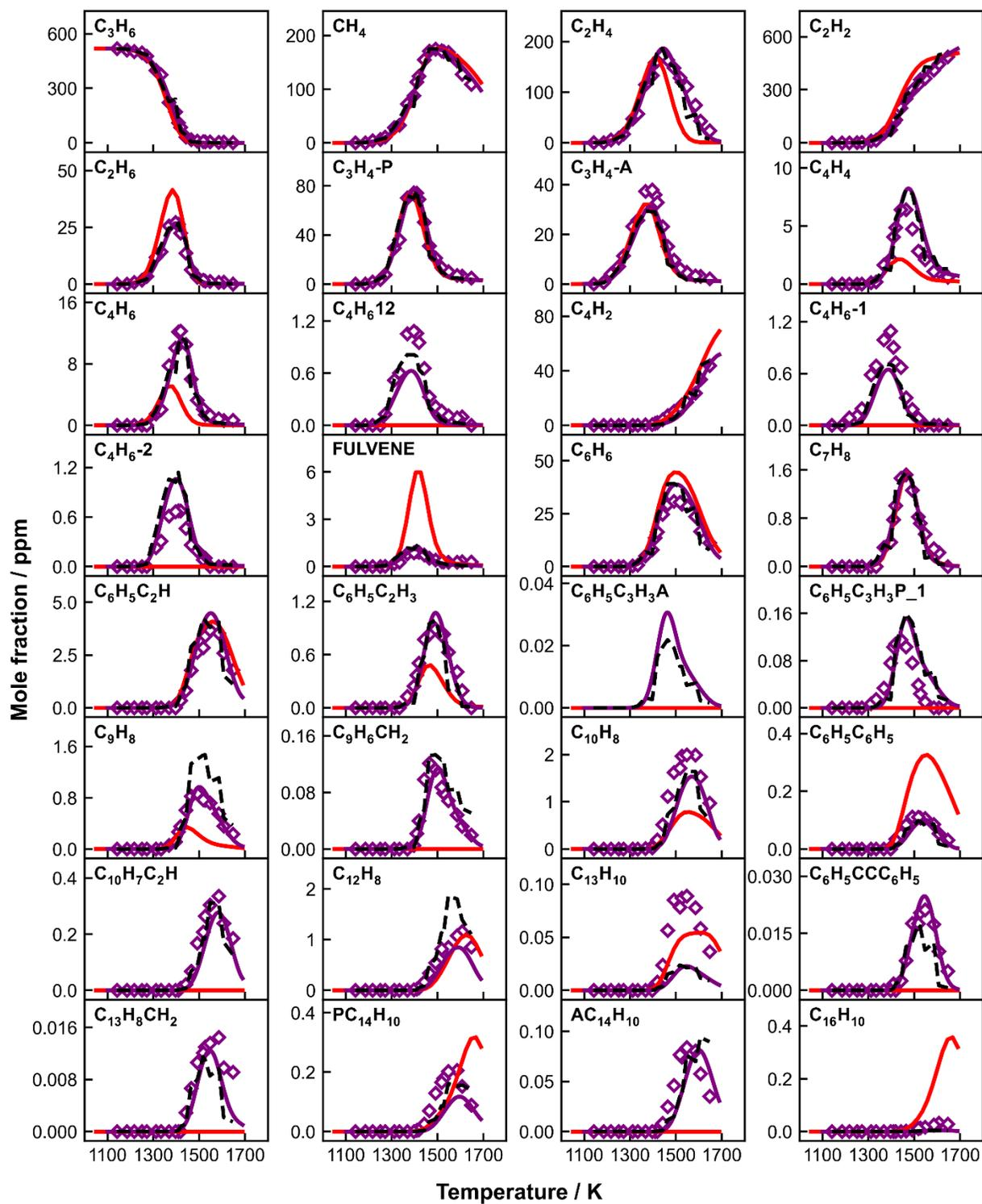
**A 2:** Measured (symbols) and simulated (lines) species mole fraction profiles as a function of  $T_5$  in propylene pyrolysis. Thick solid purple lines: simulations using the current kinetic model with the constant  $p_5$  of 20 bar and the nominal reaction time of 4
