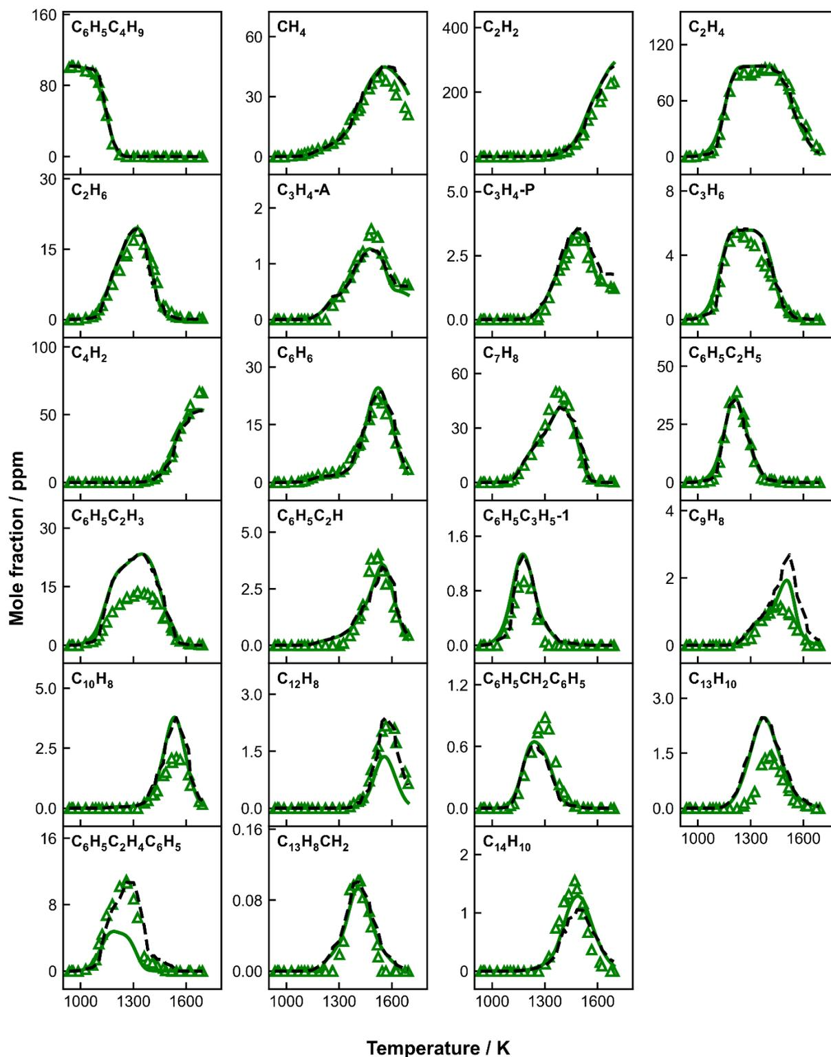
**Figure 5.91:** Species mole fractions as a function of  $T_5$  in *n*-butylbenzene pyrolysis. Symbols: measurements; solid lines: modeling results at constant 20 bar within a fixed reaction time of 4.0 ms; dashed lines: simulations with measured pressure profiles up to a time scale of 10 ms.
