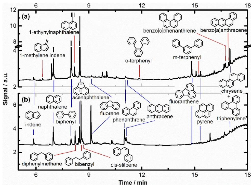
**Figure 3.13:** GC signals for PAH species detected in (a) 210 ppm benzene pyrolysis at T<sub>5</sub> = 1553 K, P<sub>5</sub> = 21.8 bar and (b) 216 ppm toluene pyrolysis at T<sub>5</sub> = 1435 K, P<sub>5</sub> = 21.1 bar [138].
