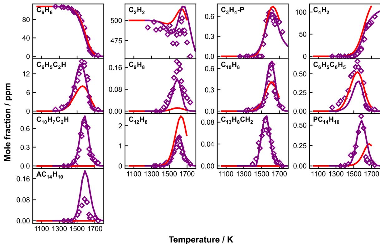
**A 4:** Measured (symbols) and simulated (lines) species mole fraction profiles as a function of  $T_5$  in 108 ppm benzene+ 500 ppm acetylene co-pyrolysis.. Thick solid purple lines: simulations using the current kinetic model with the constant  $p_5$  of 20 bar and the nominal reaction time of 4 ms; thick solid red line: simulations using CRECK model with the constant  $p_5$  of 20 bar and the nominal reaction time of 4 ms.
