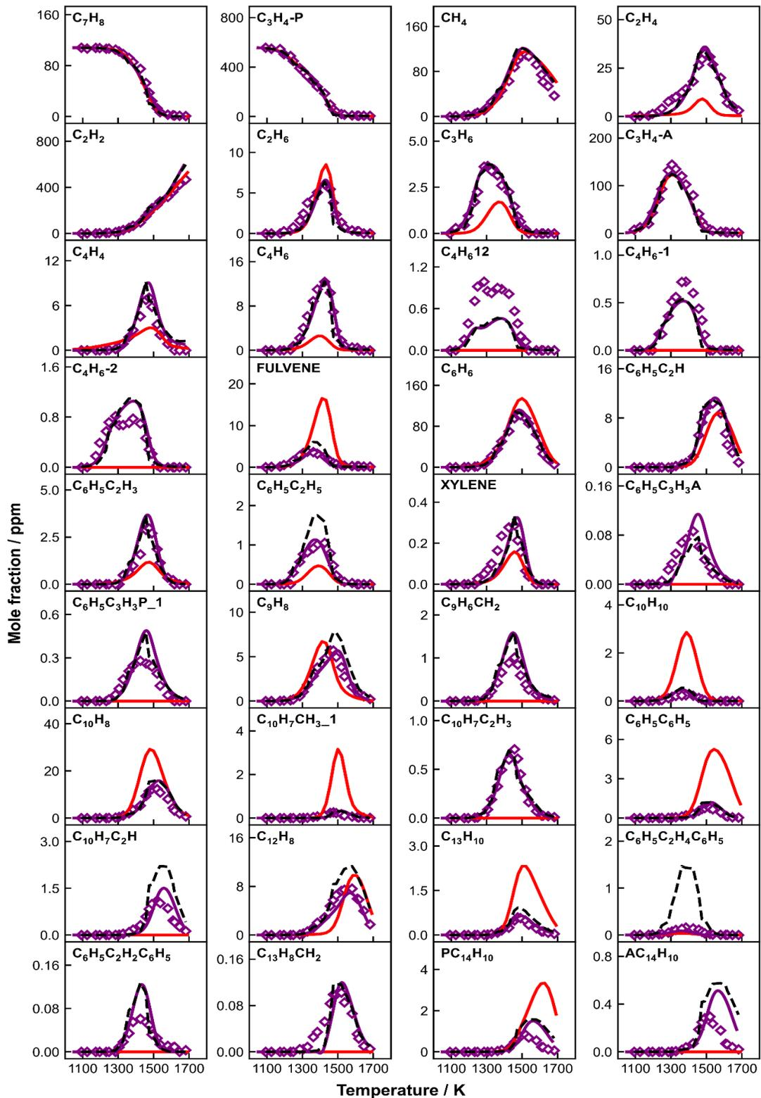
**A 13:** Measured (symbols) and simulated (lines) species mole fraction profiles as a function of  $T_5$  in 108 toluene+ 557 ppm propyne co-pyrolysis. Thick solid purple lines: simulations using the current kinetic model with the constant  $p_5$  of 20 bar and the
