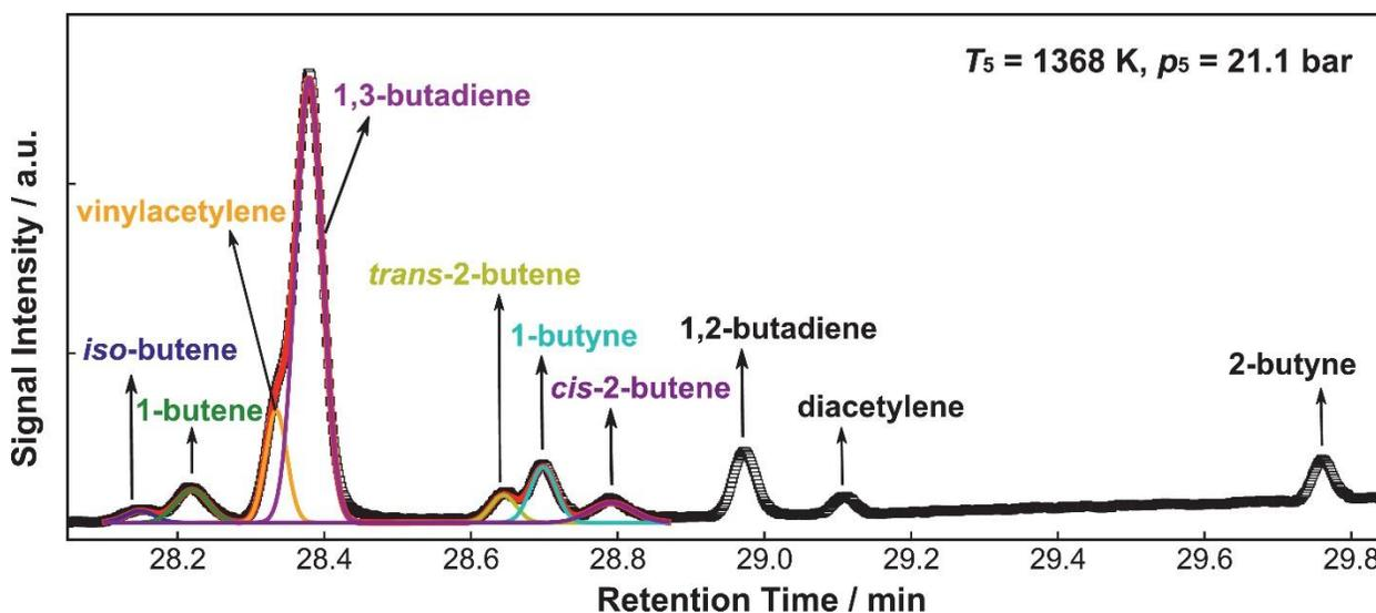
**Figure 3.11:** The signals detected for C<sub>4</sub> species in propylene pyrolysis at  $T_5 = 1368 \text{ K}$ ,  $p_5 = 21.1 \text{ bar}$ . The overlapping peaks are separated through multiple Gaussian fittings [140].
