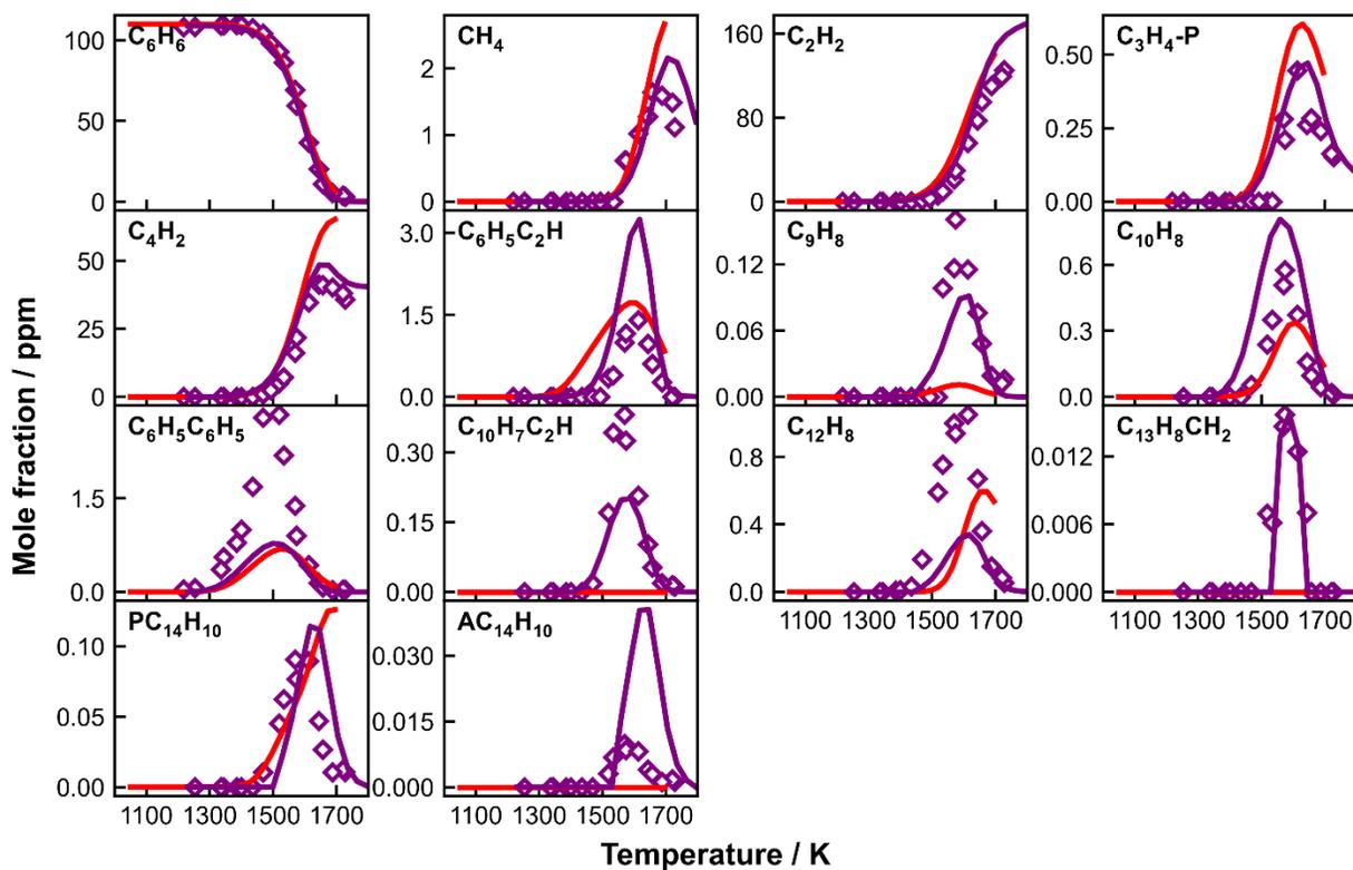
**A 3:** Measured (symbols) and simulated (lines) species mole fraction profiles as a function of  $T_5$  in 109 ppm benzene pyrolysis. Thick solid purple lines: simulations using the current kinetic model with the constant  $p_5$  of 20 bar and the nominal reaction time of 4 ms; thick solid red line: simulations using CRECK model with the constant  $p_5$  of 20 bar and the nominal reaction time of 4 ms.
