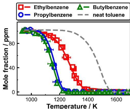
**Figure 5.83:** Experimental (symbols) and simulated (solid lines) fuel mole fractions as a function of  $T_5$  in C<sub>8</sub>–C<sub>10</sub> linear alkylbenzenes pyrolysis. Simulated fuel conversion profile in 100 ppm toluene pyrolysis is shown as the dashed line for comparison purpose.
