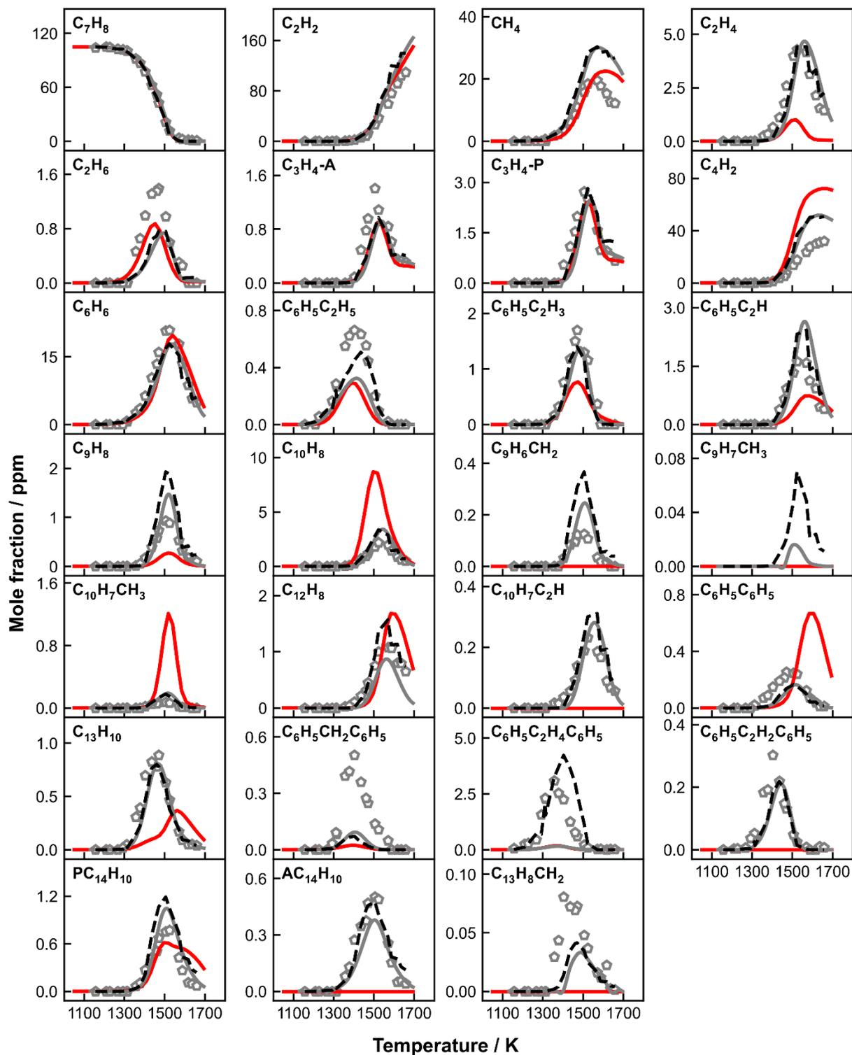
**A 8:** Measured (symbols) and simulated (lines) species mole fraction profiles as a function of  $T_5$  in 105 ppm toluene pyrolysis. Thick solid grey lines: simulations using the current kinetic model with the constant  $p_5$  of 20 bar and the nominal reaction time of
