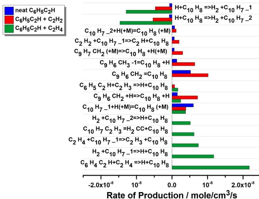
**Figure 5.80:** ROP analysis for  $C_{10}H_8$  production at  $T_5 = 1500$  K,  $P_5 = 20$  bar and reaction time = 4ms in the pyrolysis of neat  $C_6H_5C_2H$ ,  $C_6H_5C_2H+C_2H_2$  and  $C_6H_5C_2H+C_2H_4$ .
