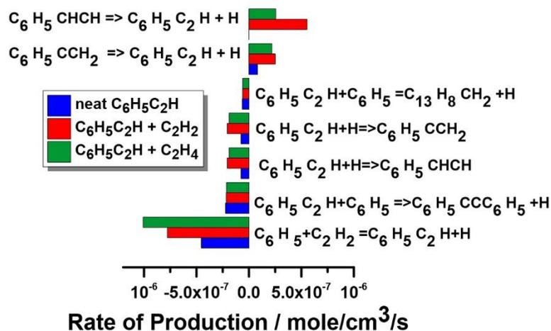
**Figure 5.76:** ROP-analysis for  $C_6H_5C_2H$  consumption at  $T_5 = 1450$  K and  $P_5 = 20$  bar in the pyrolysis of neat  $C_6H_5C_2H$ ,  $C_6H_5C_2H + C_2H_2$  and  $C_6H_5C_2H + C_2H_4$  mixtures.
