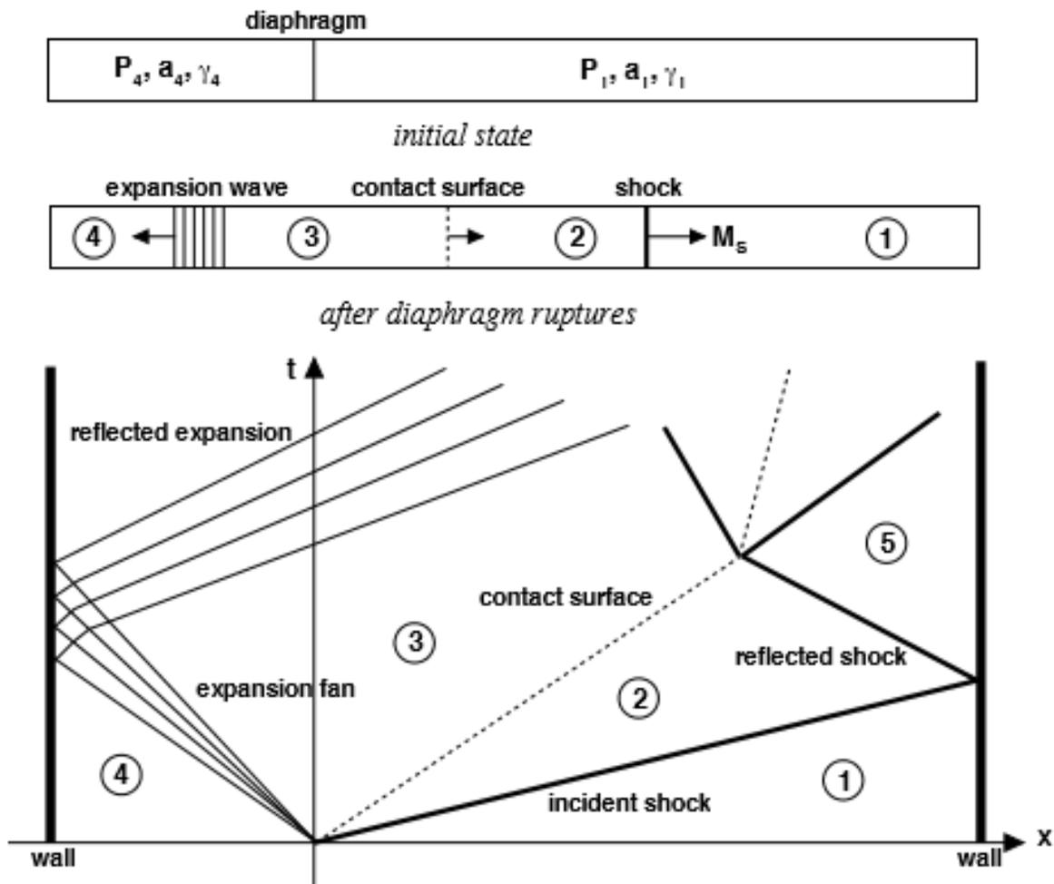
**Figure 3.1:** Schematic picture of a shock tube and  $(x, t)$  diagram showing the various regions associated with a shock wave at a time  $t$  after the bursting of the diaphragm at the origin  $O$
