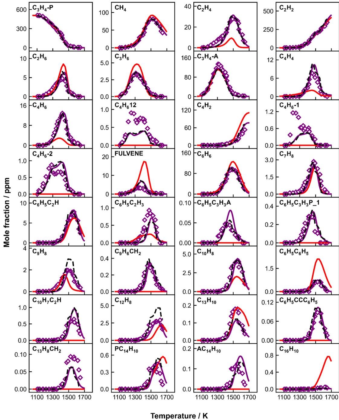
**A 1:** Measured (symbols) and simulated (lines) species mole fraction profiles as a function of  $T_5$  in propyne pyrolysis. Thick solid purple lines: simulations using the current kinetic model with the constant  $p_5$  of 20 bar and the nominal reaction time of 4
