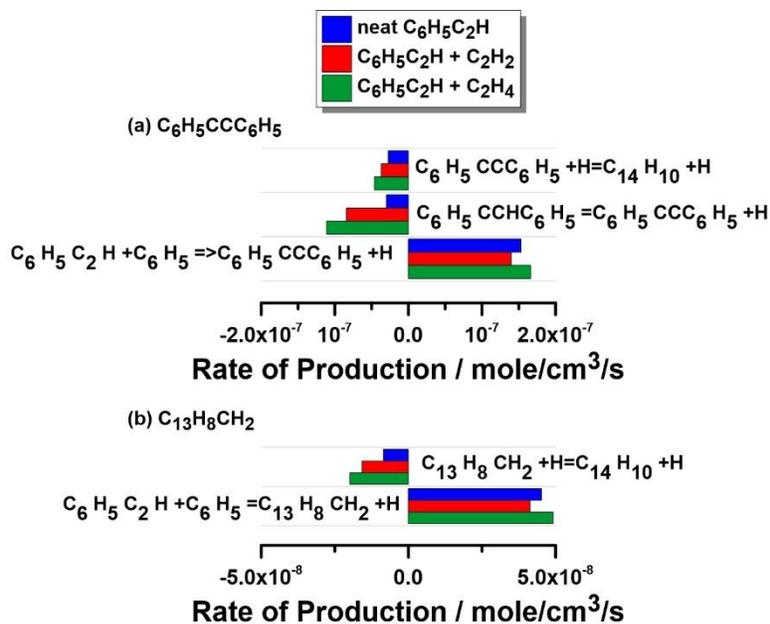
**Figure 5.82:** ROP analysis for (a)  $C_6H_5CCC_6H_5$  and (b)  $C_{13}H_8CH_2$  production at  $T_5 = 1400$  K,  $P_5 = 20$  bar and reaction time = 4ms in the pyrolysis of neat  $C_6H_5C_2H$ ,  $C_6H_5C_2H + C_2H_2$  and  $C_6H_5C_2H + C_2H_4$ .
