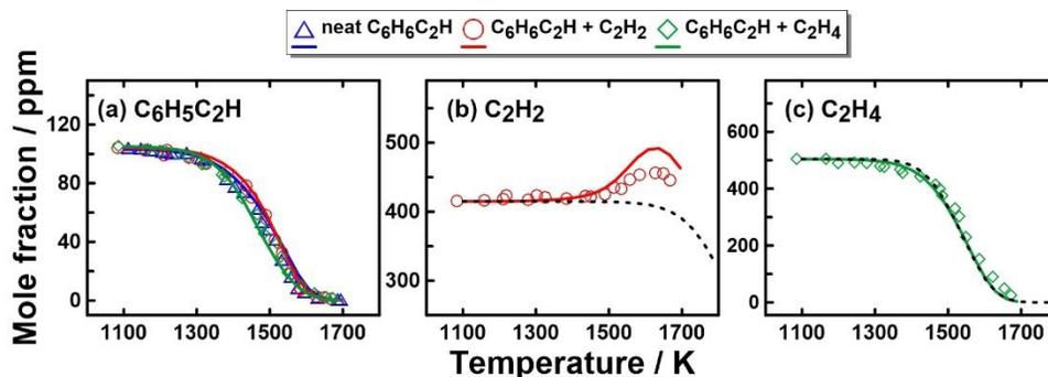
**Figure 5.75:** Experimental (symbols) and simulated (solid lines) mole fractions of (a)  $C_6H_5C_2H$  in the three investigated cases, (b)  $C_2H_2$  in the pyrolysis of 104 ppm  $C_6H_5C_2H$  + 415 ppm  $C_2H_2$  mixture and (c)  $C_2H_4$  in the pyrolysis of 105 ppm  $C_6H_5C_2H$  + 504 ppm  $C_2H_4$  mixture. The dashed lines in (b) and (c) represent the simulated mole fractions of  $C_2H_2$  and  $C_2H_4$  when  $C_6H_5C_2H$  is absent from the corresponding mixtures.
