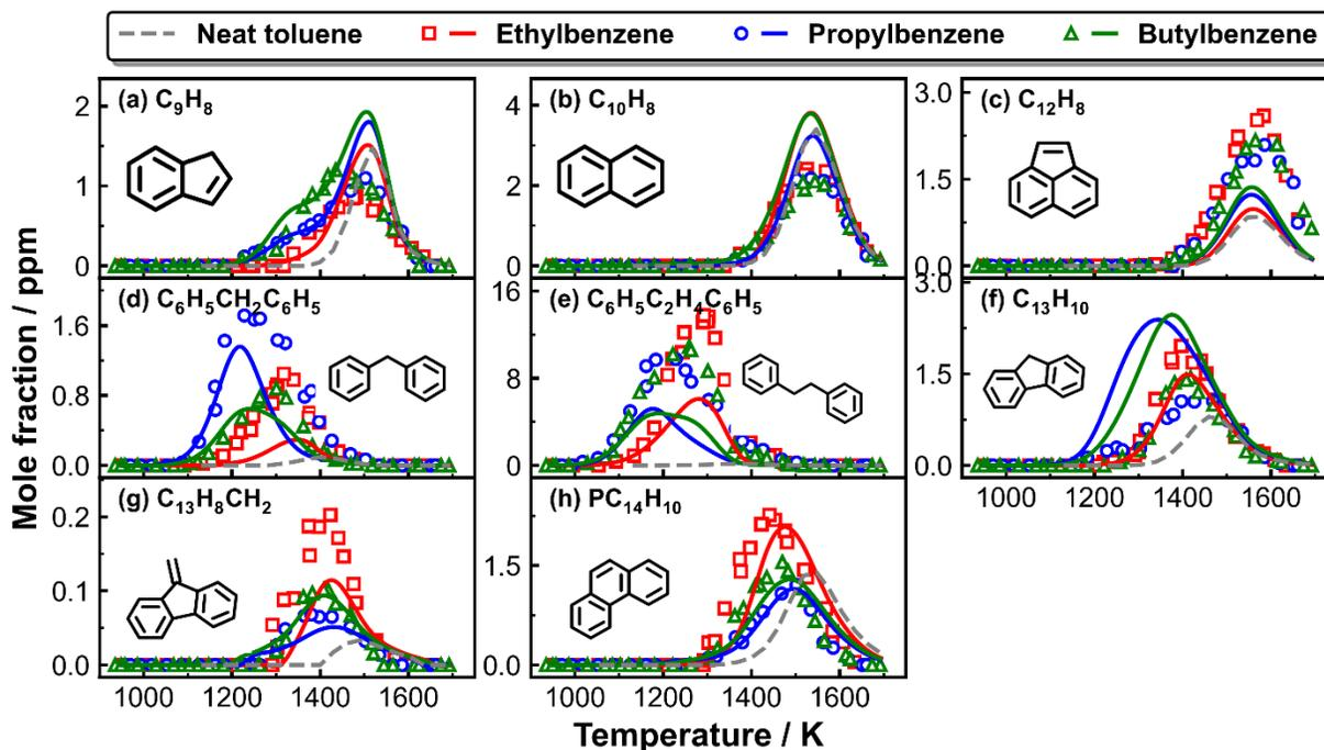
**Figure 5.88:** Experimental (symbols) and simulated (lines) mole fractions of PAH products as a function of  $T_5$  in  $C_8$ – $C_{10}$  linear alkylbenzenes pyrolysis. Simulated speciation profiles in 100 ppm toluene pyrolysis are shown as dashed lines for comparison purpose.
