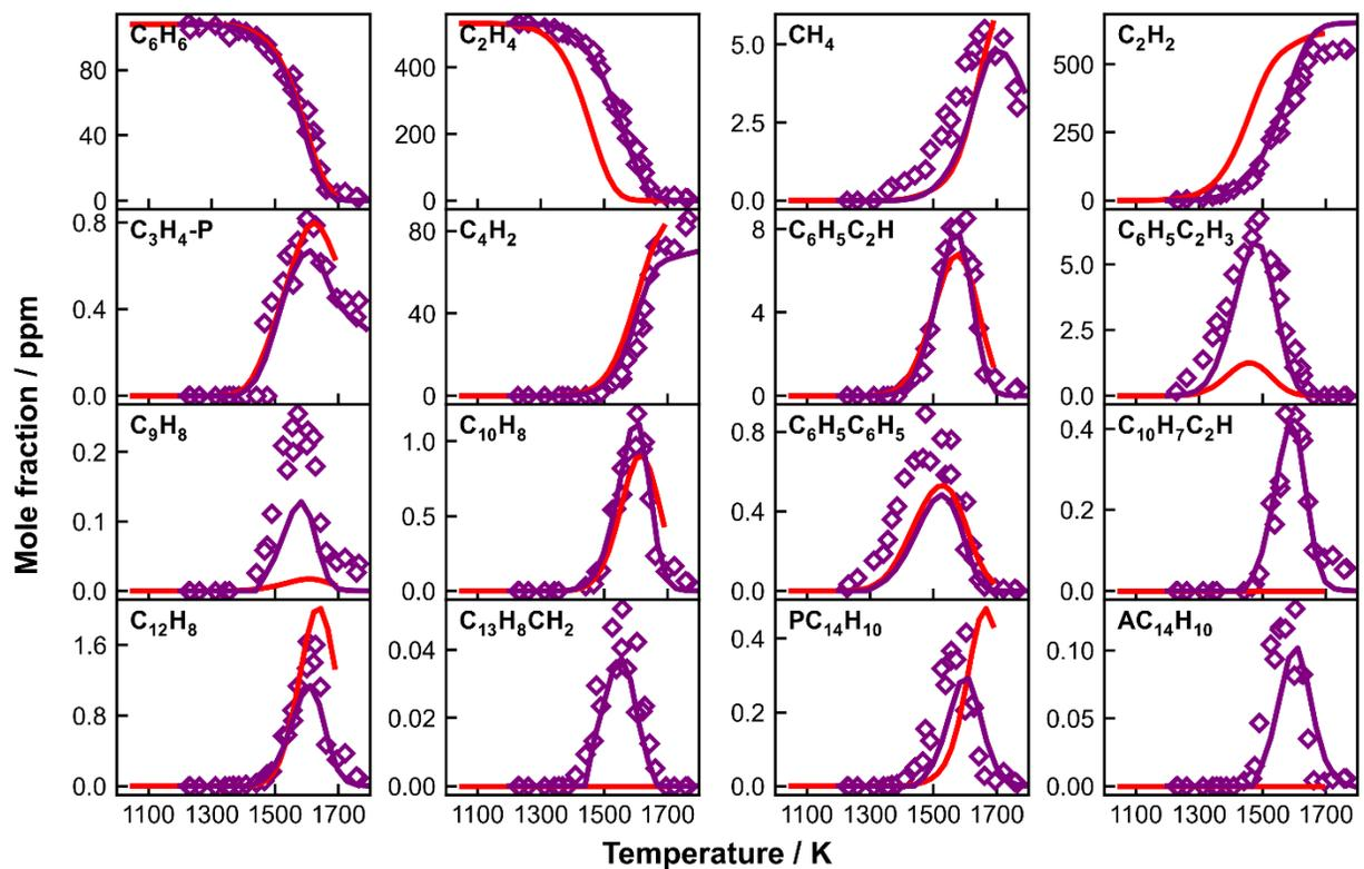
**A 5:** Measured (symbols) and simulated (lines) species mole fraction profiles as a function of  $T_5$  in 108 ppm benzene+ 532 ppm ethylene co-pyrolysis. Thick solid purple lines: simulations using the current kinetic model with the constant  $p_5$  of 20 bar and the nominal reaction time of 4 ms; thick solid red line: simulations using CRECK model with the constant  $p_5$  of 20 bar and the nominal reaction time of 4 ms.
