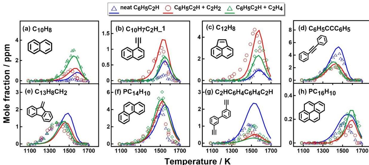
**Figure 5.79:** Measured (symbols) and simulated (lines) mole fractions of PAHs as a function of  $T_5$  from the pyrolysis of 104 ppm  $C_6H_5C_2H$ , 104 ppm  $C_6H_5C_2H + 415$  ppm  $C_2H_2$  and 105 ppm  $C_6H_5C_2H + 504$  ppm  $C_2H_4$  mixtures at the nominal  $P_5$  of 20 bar.
