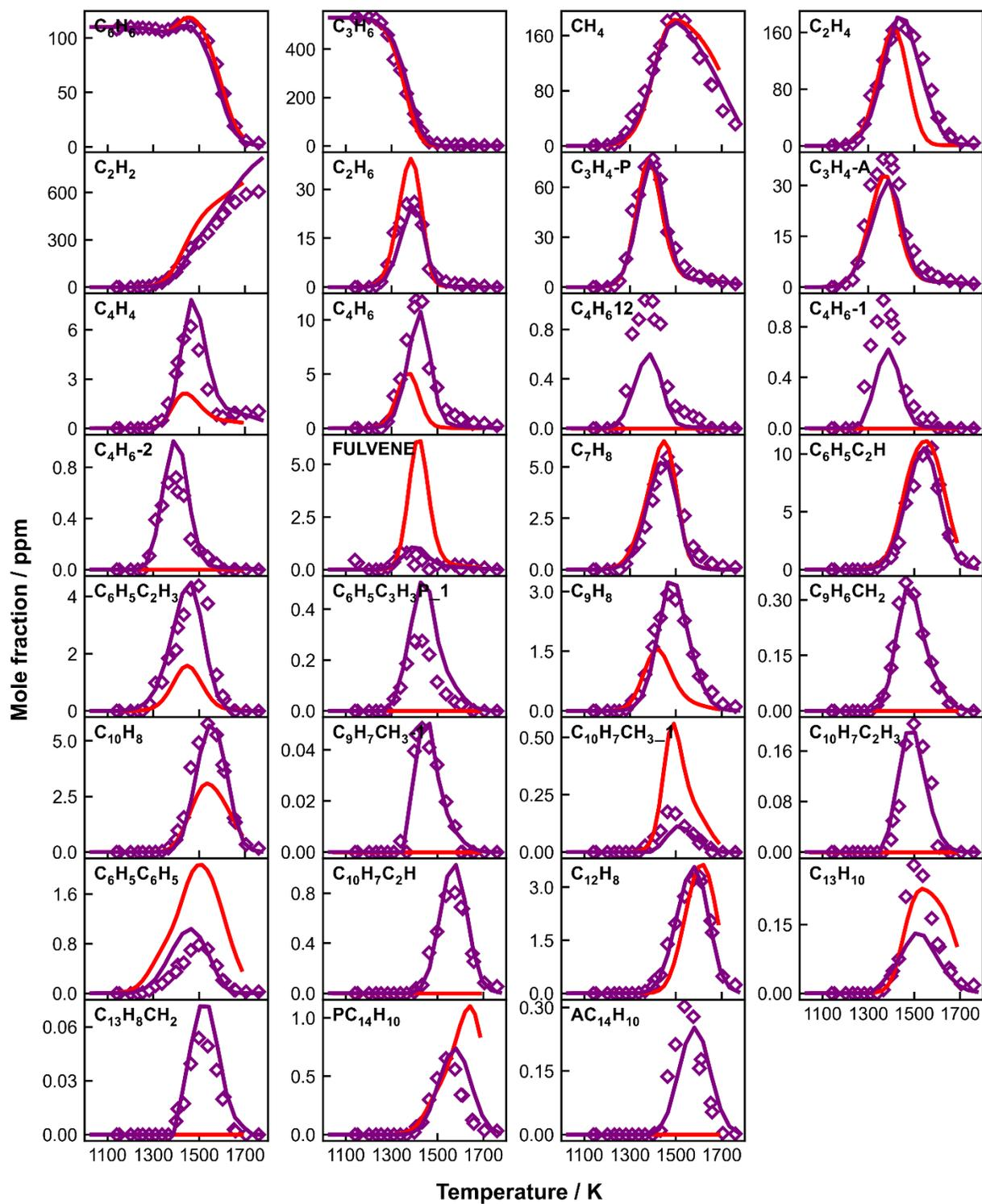
**A 6:** Measured (symbols) and simulated (lines) species mole fraction profiles as a function of  $T_5$  in 110 benzene+ 531 ppm propylene co-pyrolysis. Thick solid purple lines: simulations using the current kinetic model with the constant  $p_5$  of 20 bar and
