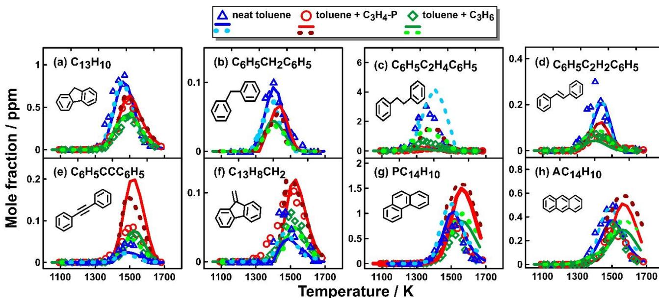
**Figure 5.71:**  $\text{C}_{13}$ - $\text{C}_{14}$  PAH mole fraction profiles as a function of the post-shock temperature  $T_5$  in neat toluene, toluene +  $\text{C}_3\text{H}_6$  and toluene +  $\text{C}_3\text{H}_4\text{-P}$  pyrolysis. Symbols: measurements; solid lines: simulations with a constant pressure of 20 bar within a reaction time of 4.0 ms; dashed lines: simulations with measured pressure histories up to 10 ms.
