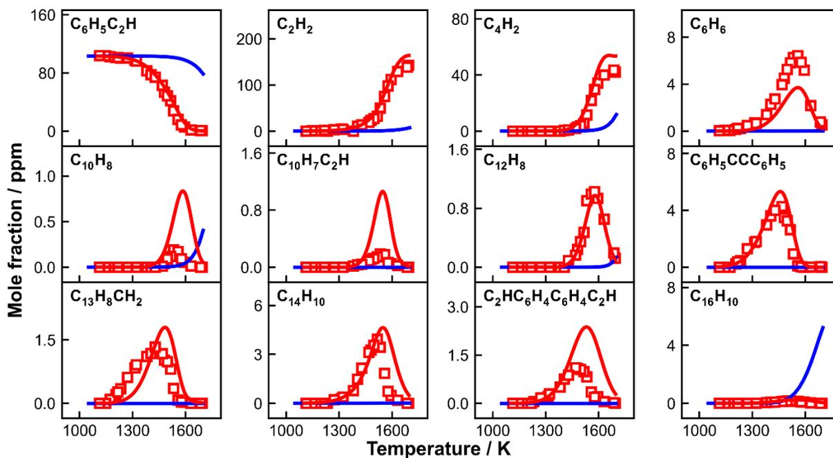
A 15: Measured (symbols) and simulated (lines) species mole fraction profiles as a function of  $T_5$  in 103 ppm phenylacetylene pyrolysis. Thick solid red lines: simulations using the current kinetic model with the constant  $p_5$  of 20 bar and the nominal reaction time of 4 ms; thick solid blue line: simulations using CRECK model with the constant  $p_5$  of 20 bar and the nominal reaction time of 4 ms.
