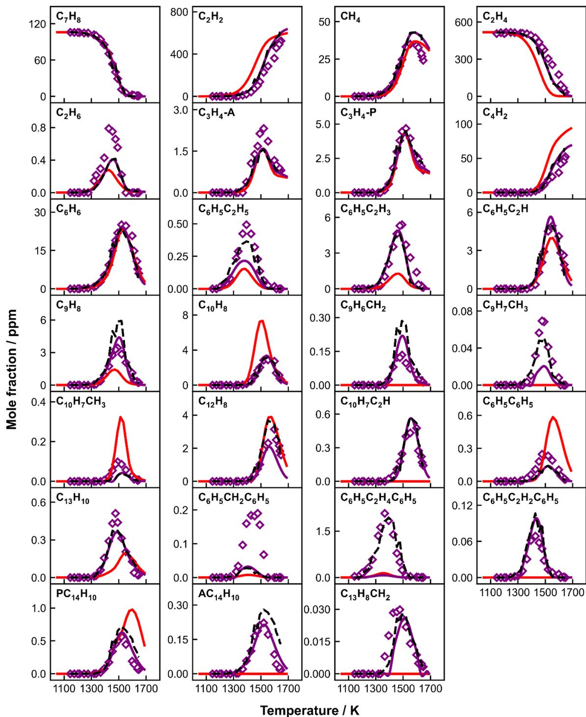
**A 12:** Measured (symbols) and simulated (lines) species mole fraction profiles as a function of  $T_5$  in 106 toluene+ 518 ppm ethylene co-pyrolysis. Thick solid purple lines: simulations using the current kinetic model with the constant  $p_5$  of 20 bar and the nominal reaction time of 4 ms; thick dashed black lines: simulations using the current model with measured pressure profiles up
