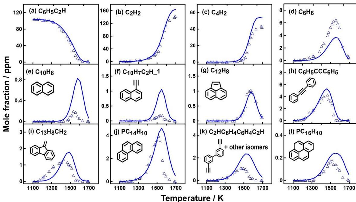
**Figure 5.73:** Mole fraction profiles (symbols) of fuel and its major products are measured from 103 ppm phenylacetylene pyrolysis in a shock tube at 20 bar. Solid lines indicate the model predictions.
