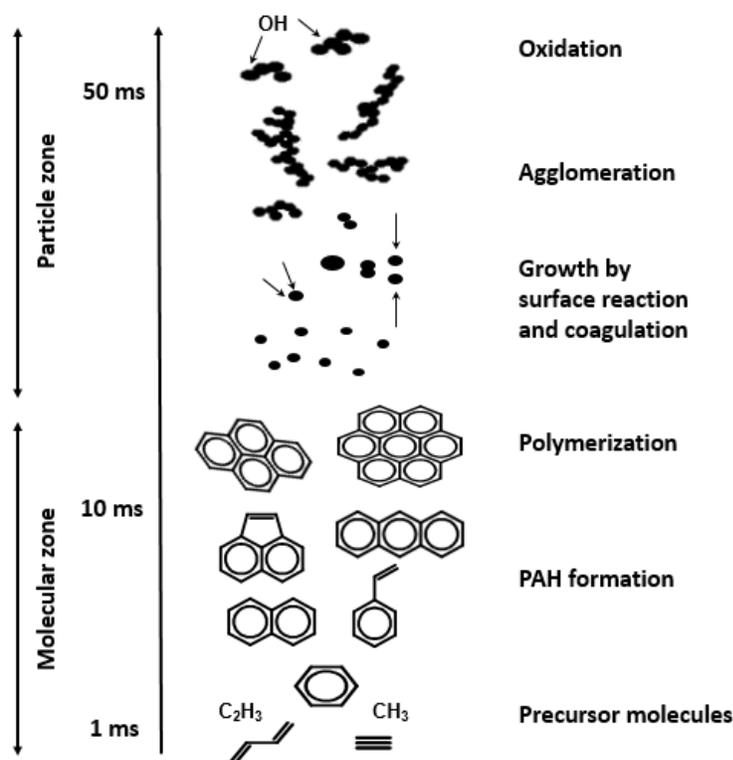
**Figure 1.1:** Schematic of soot formation steps
