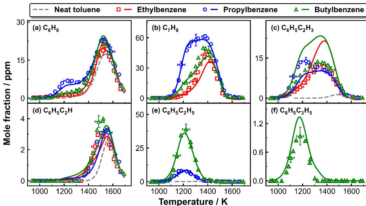
**Figure 5.87:** Experimental (symbols) and simulated (lines) mole fractions of MAH products as a function of  $T_5$  in  $C_8$ – $C_{10}$  linear alkylbenzenes pyrolysis. Simulated speciation profiles in 100 ppm toluene pyrolysis are shown as dashed lines for comparison purpose.
