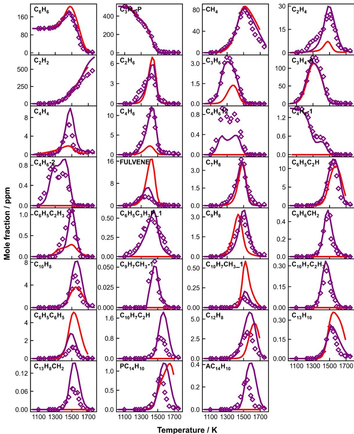
**A 7:** Measured (symbols) and simulated (lines) species mole fraction profiles as a function of T<sub>5</sub> in 108 benzene+ 508 ppm propyne co-pyrolysis. Thick solid purple lines: simulations using the current kinetic model with the constant p<sub>5</sub> of 20 bar and the
