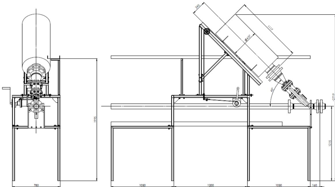
**Figure 3.3:** Schematic drawings of the dump tank
