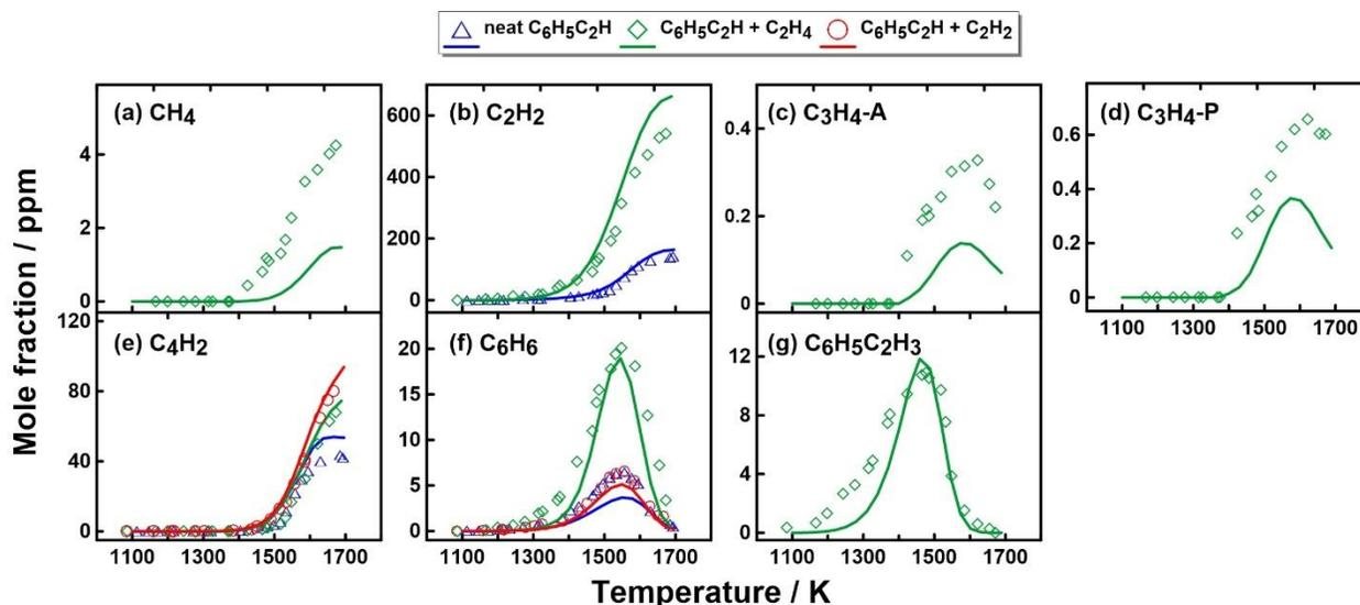
**Figure 5.77:** Measured (symbols) and simulated (lines) mole fractions of small molecule products as a function of  $T_5$  from the pyrolysis of 104 ppm  $C_6H_5C_2H$ , 104 ppm  $C_6H_5C_2H + 415$  ppm  $C_2H_2$  and 105 ppm  $C_6H_5C_2H + 504$  ppm  $C_2H_4$  mixtures at the nominal  $P_5$  of 20 bar.
