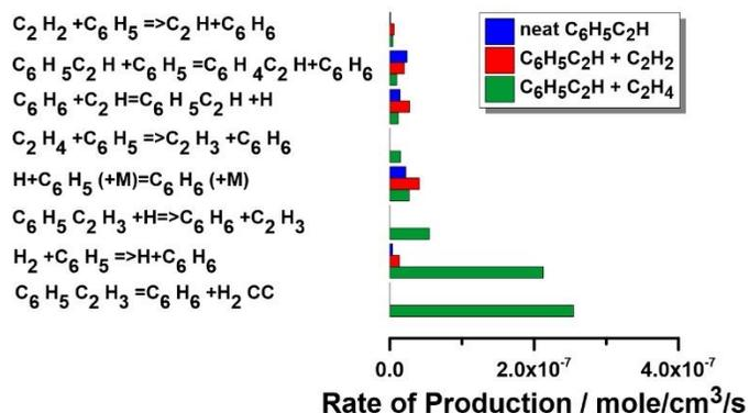
**Figure 5.78:** ROP analysis for  $C_6H_6$  production at  $T_5 = 1550$  K,  $P_5 = 20$  bar and reaction time = 4ms in the pyrolysis of neat  $C_6H_5C_2H$ ,  $C_6H_5C_2H + C_2H_2$  and  $C_6H_5C_2H + C_2H_4$ .
