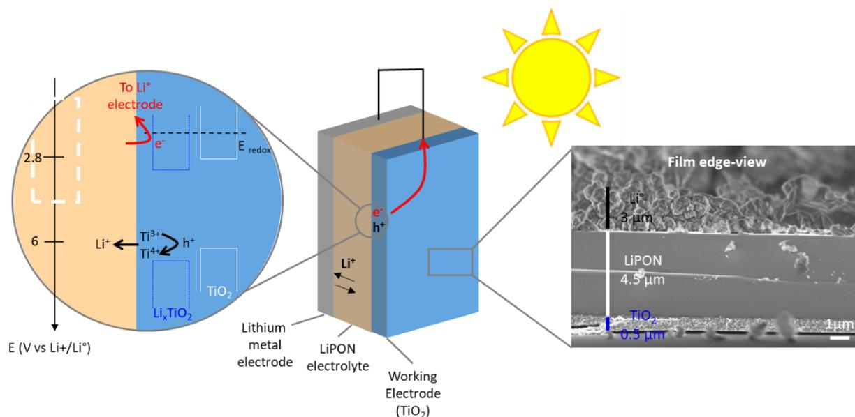
**Figure 49:** Schema of the system: glass/FTO/TiO<sub>2</sub>// LiPON// Li°. With a schema of the band diagram of TiO<sub>2</sub> and Li<sub>x</sub>TiO<sub>2</sub> and the LiPON electrochemical stability window in white dots scare on the left and on the right SEM-FEG images of the battery on an edge-view.
