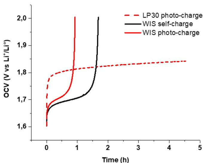
**Figure 37:** Comparison of OCV evolutions of pre-lithiated electrodes. The pre-lithiated electrodes were obtained after a discharge at 2C-rate in dark. Photo-charge in LP30 is presented in red dash, photo-charge in WIS is presented in red line. The Self-charge in WIS (OCV in dark) is presented in black as a reference.
