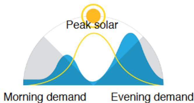
**Figure 3:** Electricity demand (blue curve) compared with solar power (yellow curve) over a day.<sup>6</sup>
