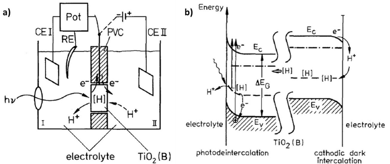
**Figure 15:** a) Two compartment electrochemical set-up. Both compartments are separated with a PVC plate, have a Pt counter electrode immersed in an acidic aqueous electrolyte. The  $TiO_2(B)$  electrode is mounted onto a hole in the center of the plate. b) The energy band scheme of the set-up presented in a).<sup>63</sup>
