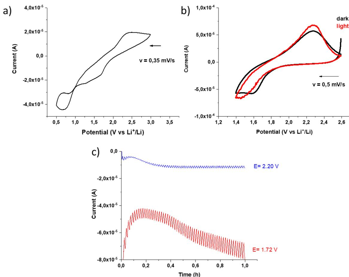
**Figure 47:** (a) CV at 0.35 mV/s starting from 3 to 0.5 V vs  $\text{Li}^+/\text{Li}^\circ$ , (b) CVs at 0.5 mV/s from 2.6 to 1.4 V vs  $\text{Li}^+/\text{Li}^\circ$  under dark (black line) and under illumination (red), (c) potentiostatic chopped (30s under illumination, 30 s under dark conditions) at 2.2 V (blue line) and 1.7 V (red line) the set up used is (+) b-Si/ $\text{TiO}_2$ //LP30 (1M)// $\text{Li}^\circ$ ,  $\text{Li}^\circ$  (-).
