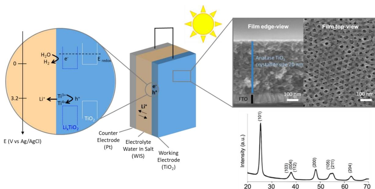
**Figure 21:** Schema of the system: glass/FTO/ $\text{TiO}_2$ // Water In Salt (WIS) 20 M of LiTFSI // AgAgCl (KCl saturated)/ Pt. With a schema of the band diagram of  $\text{TiO}_2$  and  $\text{Li}_x\text{TiO}_2$  on the left and on the right SEM-FEG images of the  $\text{TiO}_2$  film with an edge-view and a top-view, XRD of the  $\text{TiO}_2$  anatase thin film.
