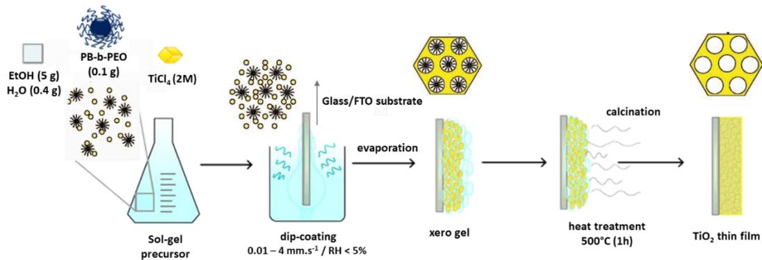
**Figure 23:** Sol-gel dip coating thin film fabrication process. Adapted from Hilliard.<sup>1</sup>
