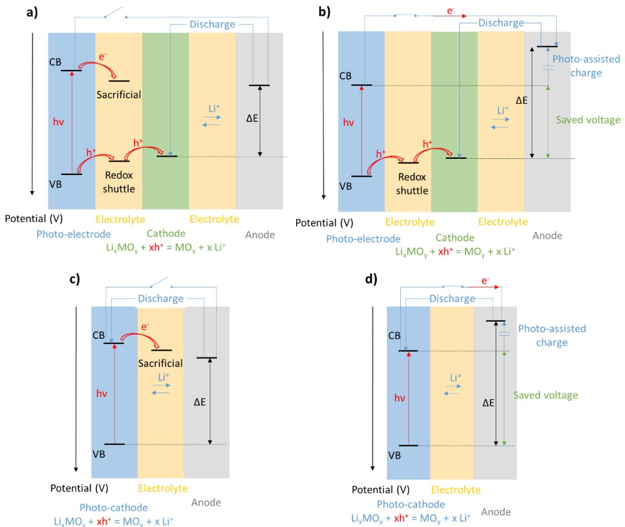
**Schema 1:** (a) Illustration of a photo-charge (OCV under illumination) of a 3 electrode-set-up, (b) Illustration of a photo-assisted charge (galvanostatic experiment under illumination) of a 3 electrode-set-up, (c) illustration of a photo-charge (OCV under illumination) of a 2 electrode-set-up, (d) illustration of a photo-assisted charge (galvanostatic experiment under illumination) of a 2 electrode-set-up.
