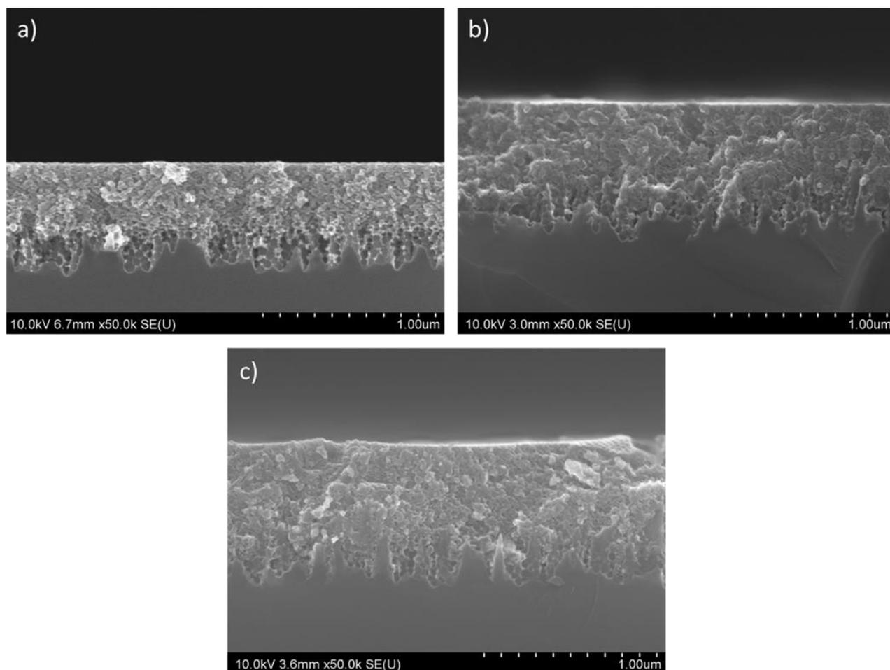
**Figure 48:** Side view of the film by SEM-FEG images. Study on the density of the first layer of  $\text{TiO}_2$  on the b-Si substrate. (a) 200 mg of Pb-b PEO, (b) 100 mg, (c) 50 mg.
