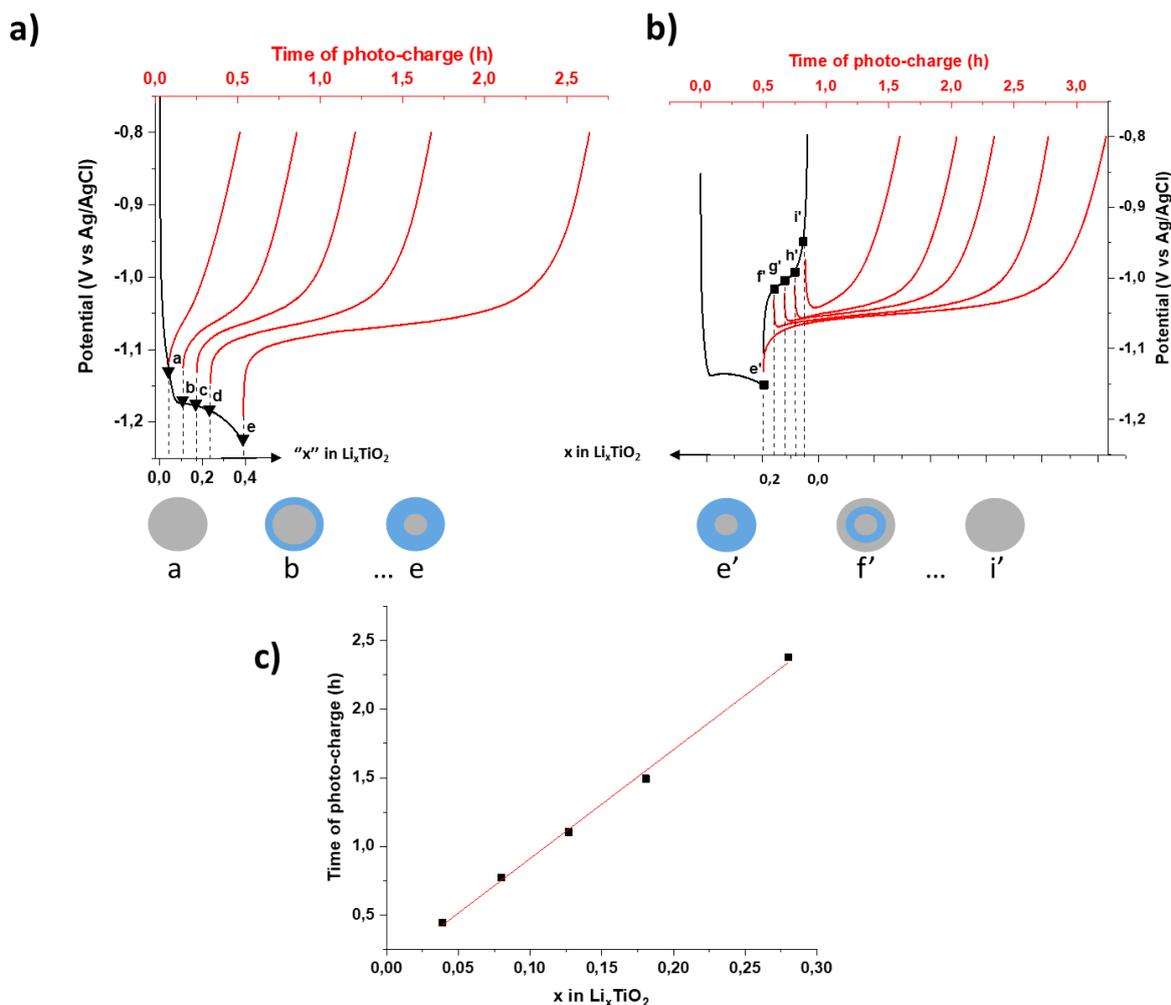
**Figure 41:** (a) Galvanostatic discharge stopped at different composition of lithium (a to e) followed by photo-charge (OCV under illumination), (b) galvanostatic charge stopped at different composition of lithium (e to i) followed by photo-charge (OCV under illumination), c) Time of photo-charge versus the lithium composition in the  $\text{TiO}_2$ .
