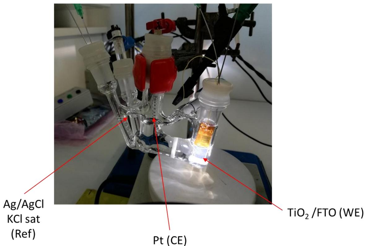
**Figure 26:** Picture of the 2 compartment set up. In the left compartment a platinum and a Ag/AgCl KCl saturated reference electrode are immersed in LiTFSI water in salt (WIS) 20 m. The right compartment is only composed of the  $TiO_2$  working electrode. Both compartments are separated by a ceramic membrane and gas tight.
