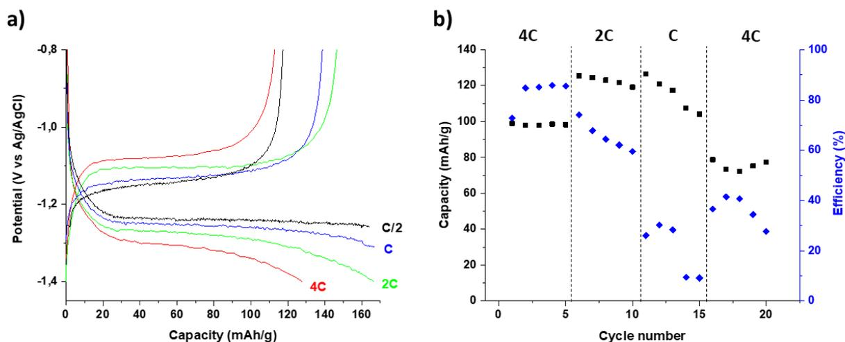
**Figure 31:** (a) Galvanostatic cycle at different C-rate from 4C to C/2. (b) Study of the evolution of the charge capacity (black) and the coulombic efficiency (blue) over cycling and C-rate. Cut-off in discharge: -1.4 V and in time. Cut-off in charge: -0.8 V.
