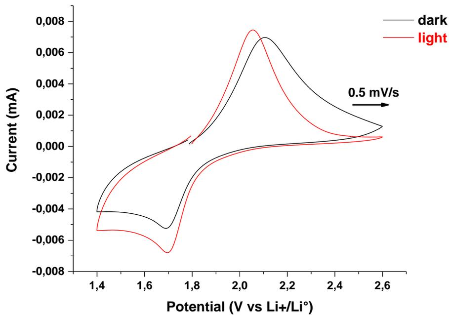
**Figure 50:** Cyclic voltammetry at 0.5 mV/s from 2.6 and 1.4 V of (+) FTO/TiO<sub>2</sub>/LiPON/Li<sup>o</sup> (-) under dark (black line) and light (red line) conditions. (Here the area is not normalized by the surface)
