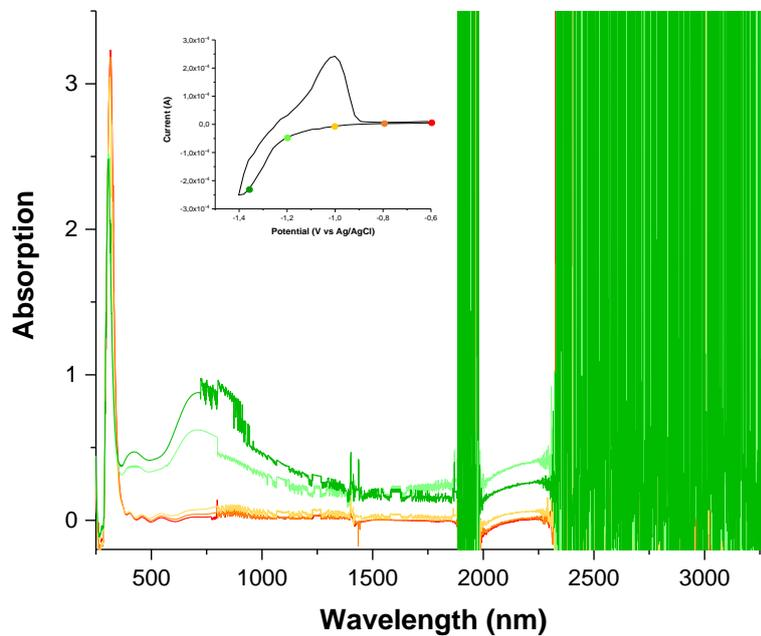
*Absorption spectra from 3500 nm to 250 nm at different state of charge during the reduction of the  $\text{TiO}_2$  electrode at 0.5 mV/s.*
