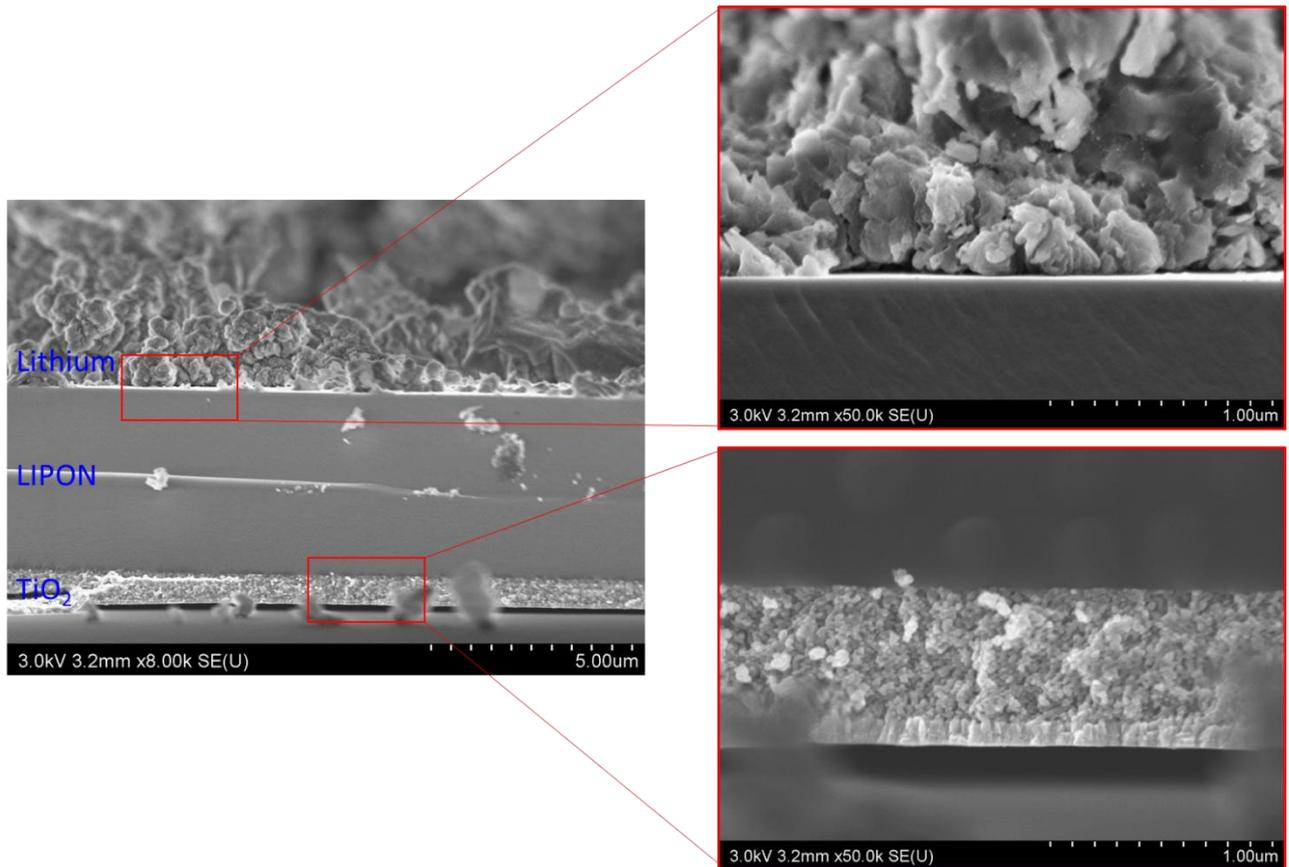
**Figure 51:** SEM-FEG images of the (+) FTO/TiO<sub>2</sub>/LiPON/Li<sup>o</sup> (-) from side view with a zoom of the LiPON/Li<sup>o</sup> interface (top) and a zoom of the TiO<sub>2</sub>/LiPON interface (bottom).
