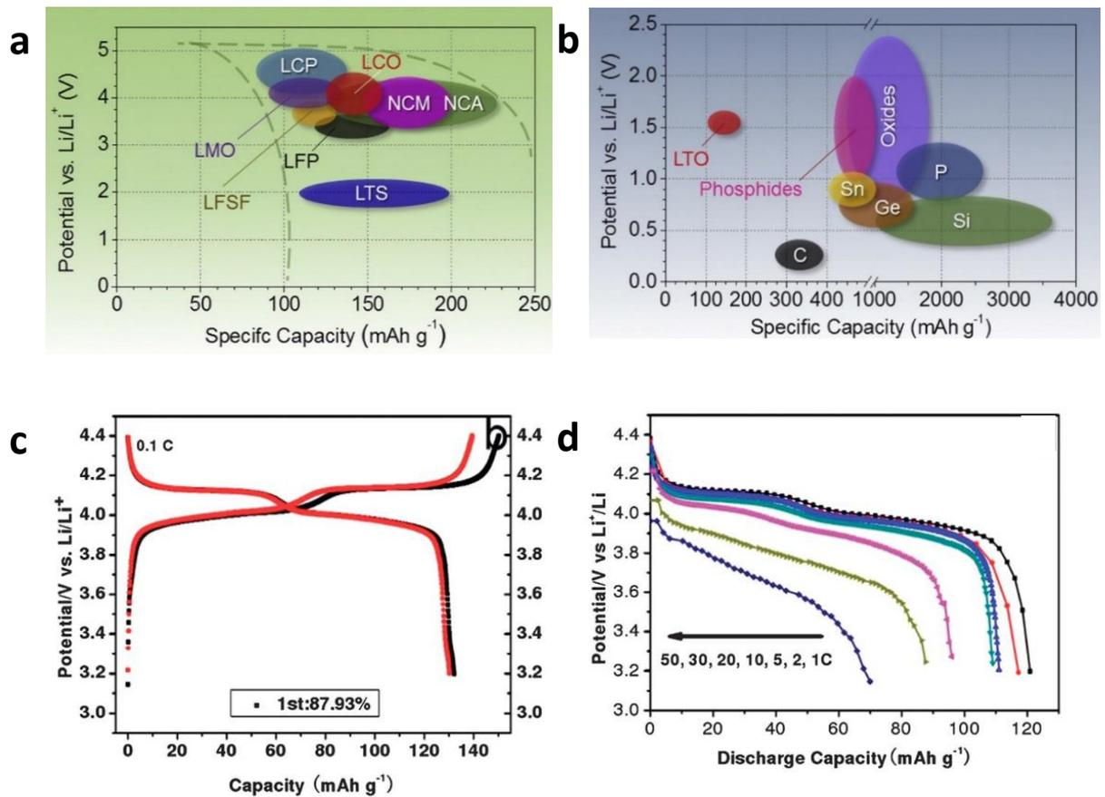
**Figure 5:** a) Approximate range of average discharge potentials and specific capacity of some of the most common (a) intercalation-type cathodes (experimental), (b) conversion type anodes (experimental) adapted from *Materials Today*, 18 (2015)<sup>19</sup>. c) discharge curves at different C-rate of an LMO (lithium manganese oxide) electrode, d) discharge-charge curves at 0.1 C. Adapted from *J. Mater. Chem. A* 1 (2013) 8170-8177.<sup>20</sup>
