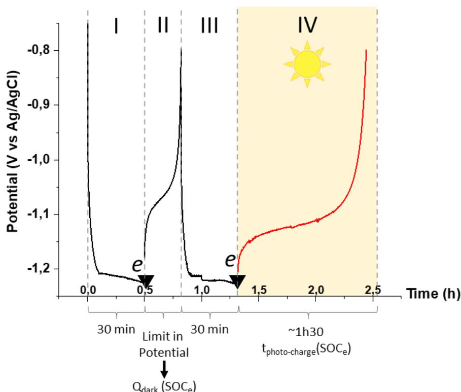
**Figure 40:** Sequence of the different steps from I to IV for one lithium composition ( $\text{SOC}_e$ ), the sequence is repeated for each  $\text{SOC}_i$ . Step I: galvanostatic discharge during 30 min ( $\text{SOC}_e$ ) at 2C, step II: galvanostatic charge with a potential limit of -0.8 V vs Ag/AgCl KCl sat, step III: galvanostatic discharge during 30 min ( $\text{SOC}_e$ ) at 2C, Step IV: Photo-charge (at OCV under illumination).
