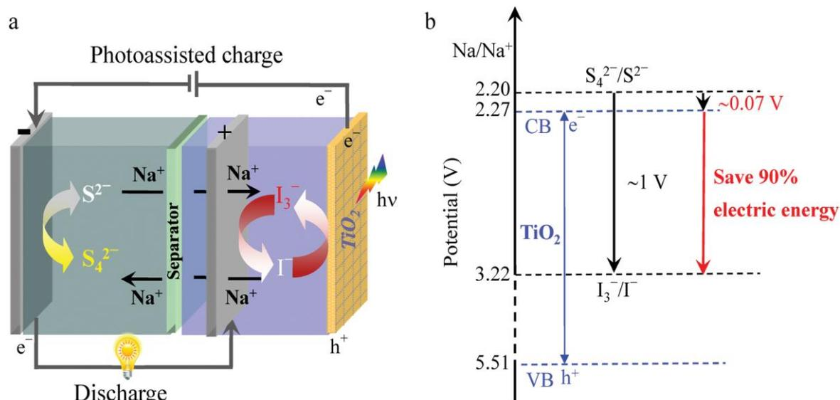
**Figure 10:** a) Schematic of a photo-assisted chargeable sodium polysulfide/iodine battery (SPIB) with a three electrode system. b) Potential diagram for the photo-assisted charging process. The saved voltage is determined by the energy difference between the charging voltage of SPIB and the quasi-Fermi level of electrons in the TiO<sub>2</sub> photo-electrode (near to its CB).<sup>42</sup>
