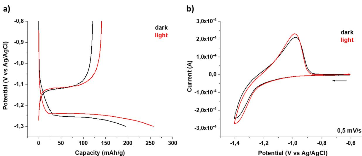
**Figure 43:** (a) Galvanostatic discharge and charge in dark conditions (black curves) and under illumination (red curves) at a 2C rate, (b) CV in dark conditions (black curves) and under illumination (red curves) at 0.5 mV/s from -0.6 V to 1.4 V vs Ag/AgCl of FTO/TiO<sub>2</sub>// WIS (20 m)// Ag/AgCl (KCl sat)/ Pt.
