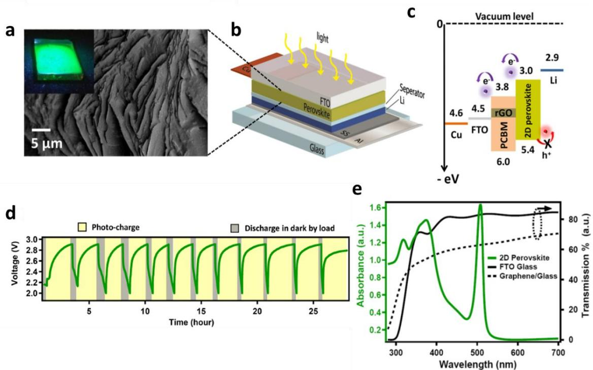
**Figure 17:** (a) SEM image of drop-cast 2D perovskite electrodes taken at 45° tilt. The inset shows a photo luminescence (PL) image of the corresponding perovskite film ( $\lambda_{ex} \sim 300$  nm LED source). (b) Schematic and (c) energy level diagram of perovskite photo-batteries. (d) Galvanostatic cycling discharge / photo-charge. (e) Optical absorption spectra of CHPI thin films and transmission of FTO glass and graphene substrates.<sup>74</sup>
