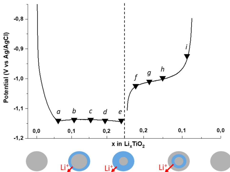
**Figure 38:** Galvanostatic discharge and charge curve at 2C in  $\text{TiO}_2//\text{WIS (20 m)//AgAgCl KCl saturated/ Pt}$ , the arrangement between the different phases at different SOC (from a to i) are illustrated under the galvanostatic experiment. Red arrows representing the photo-extraction of  $\text{Li}^+$ .
