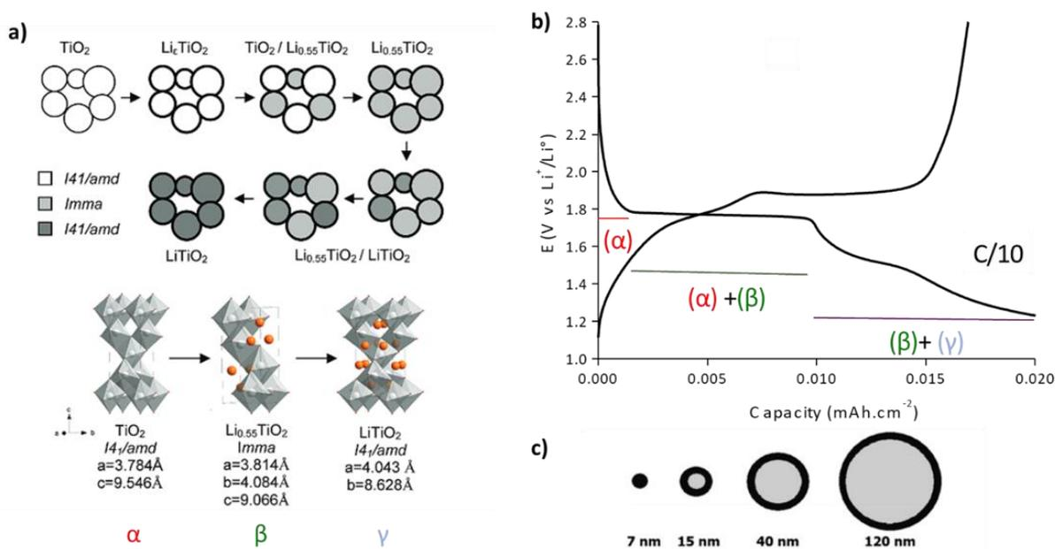
**Figure 27:** a) Phase transition upon Li insertion in anatase  $\text{TiO}_2$  (gray) Ti, red = O, orange = Li)<sup>8</sup>, b) distribution of the phases over a galvanostatic cycle at C/10 of a  $\text{TiO}_2$  anatase, c) spatial distribution of  $\text{LiTiO}_2$  phase in a lithium poor phase.<sup>9</sup>
