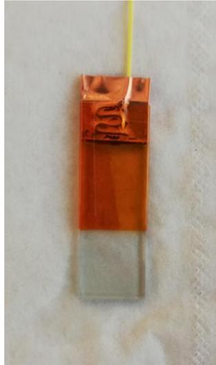
**Figure 24:** Picture of the FTO/TiO<sub>2</sub> electrode as describe above. With the Kapton tape used to delimitate the TiO<sub>2</sub> exposed surface at 1 cm<sup>2</sup>.
