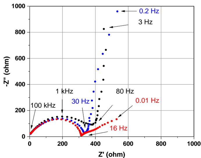
**Figure 39:** Impedance of initial  $\text{TiO}_2$  (●),  $\text{Li}_{0.3}\text{TiO}_2$  (●) and  $\text{TiO}_2$  (after the charge, ●).
