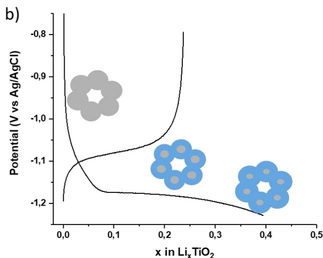
**Figure 32:** (a) SEM-FEG image of the surface of the TiO<sub>2</sub> with a zoom and a visualization of the crystallite materialized by blue circles, (b) galvanostatic cycle at a 2C rate with the evolution of the composition over a discharge schematized by circles with in grey the lithium poor and in blue the titanate phase.
