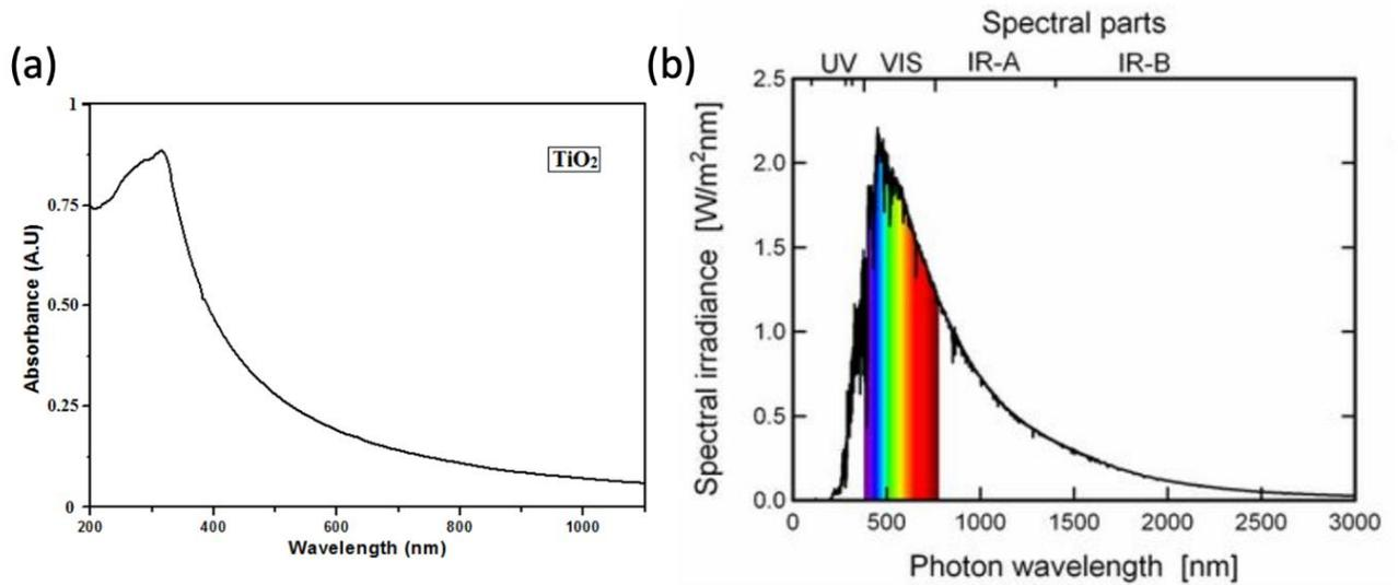
**Figure 4:** (a) UV-Visible absorption spectrum of  $\text{TiO}_2$  nanoparticles,<sup>17</sup> (b) Spectral irradiance at Air Mass 0 (AM0) vs photon wavelength.<sup>18</sup> Air Mass is explain in the **annex I**.
