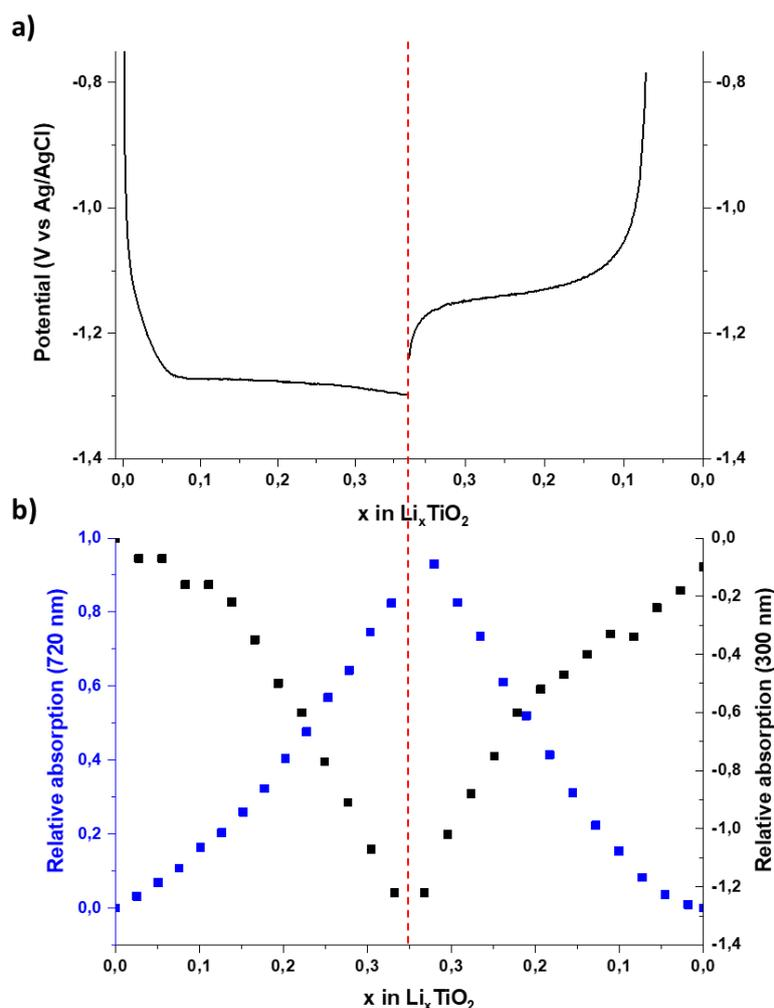
**Figure 34:** (a) Galvanostatic charge and discharge at a 2C rate potted with the lithium composition, (b) evolution of the 720 nm band (blue score) and the 300 nm band (black score) over the lithium composition.
