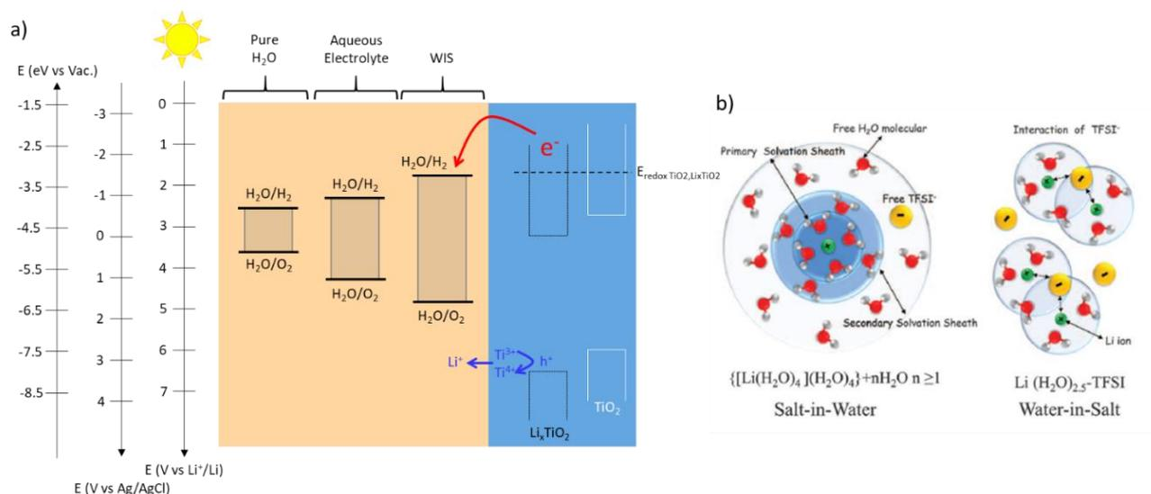
**Figure 22:** a) Stability window of pure water, aqueous electrolyte and water in salt electrolyte<sup>131</sup> regarding the band diagram of TiO<sub>2</sub> and lithiated TiO<sub>2</sub><sup>89</sup>. b) Illustration of the evolution of the Li<sup>+</sup> primary solvation sheath in diluted and water-in-salt solutions.<sup>131</sup>
