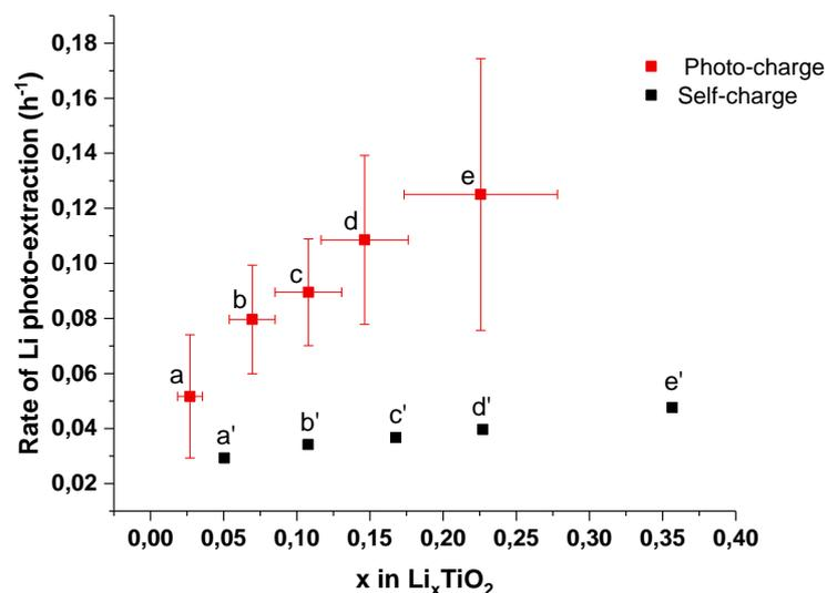
(red) Rate of the photo-extraction of the Li<sup>+</sup> over different composition of lithium (a to e) in the TiO<sub>2</sub>, (black) Rate of the self-extraction of the Li<sup>+</sup> over different composition of lithium (a' to e') in the TiO<sub>2</sub>.
