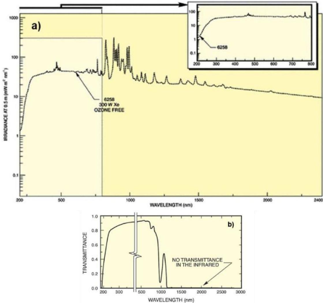
**Figure 25:** Newport 300 W Xe arc lamp ozone free spectrum (model 6258) (a) and Oriel liquid filter 61945 transmission (250-950 nm) (b).
