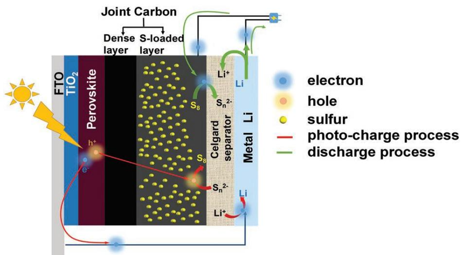
**Figure 8:** Schematic diagram of the fabricated PSC–Li–S battery FTO/ TiO<sub>2</sub>/perovskite/C/C-S/Celgard/ Li<sup>o</sup>.<sup>40</sup>
