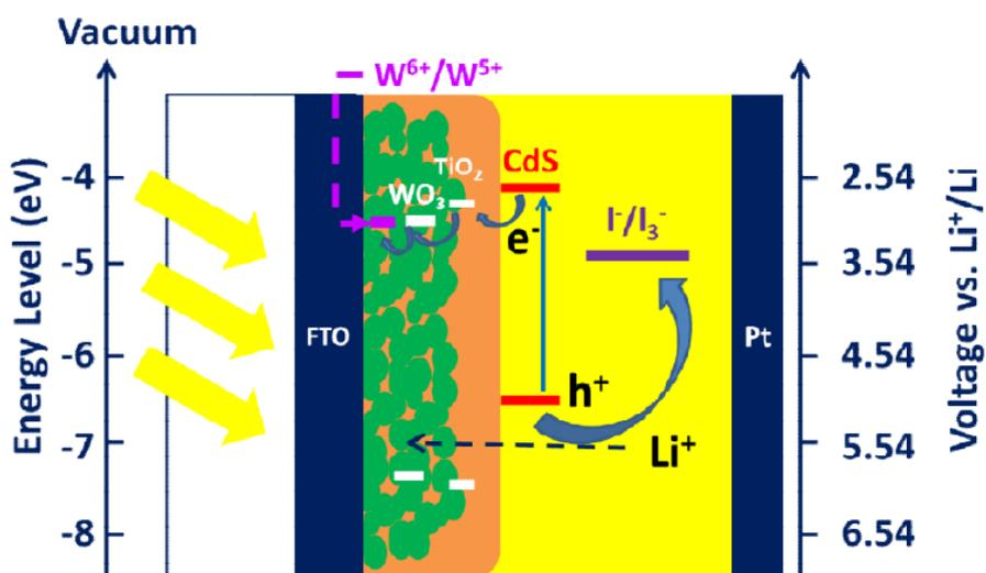
**Figure 14:** Schematic depiction of the photoelectrochemical system of CdS-sensitized WO<sub>3</sub> nanocomposite // LiI in propylene carbonate (PC) electrolyte // Pt cathode during photo-charging process.<sup>31</sup>
