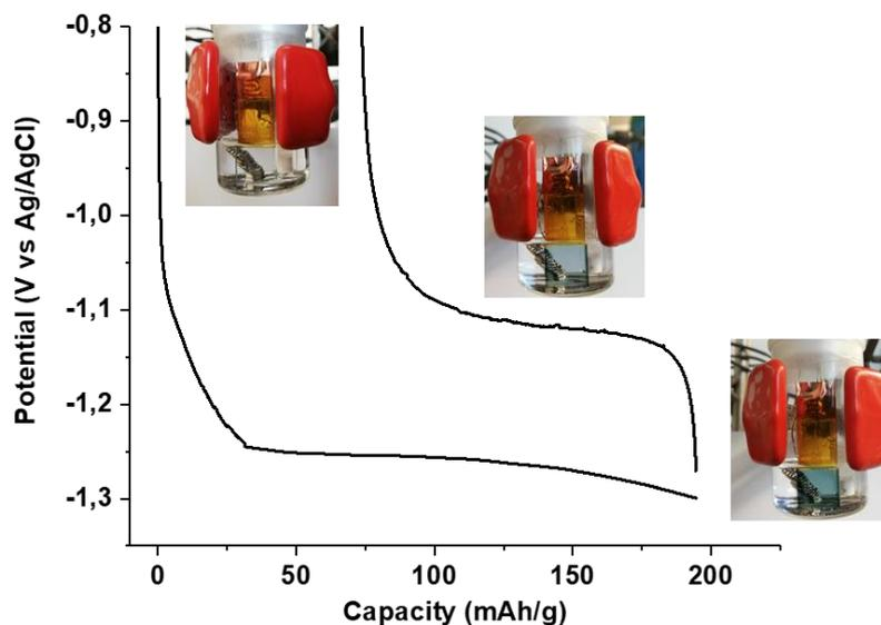
Pictures illustrating the change of color upon galvanostatic cycle at 2C-rate of  $\text{FTO}/\text{TiO}_2//\text{WIS (20m) // AgAgCl KCl saturated /Pt}$ .
