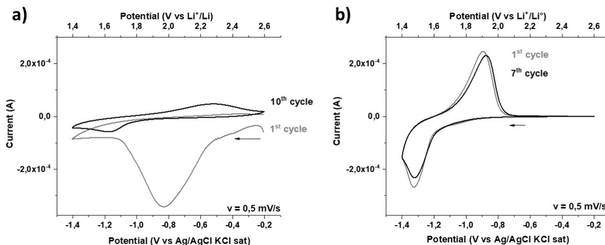
a) 1<sup>st</sup> and 10<sup>th</sup> cyclic voltammetry (CV) at 0.5 mV/s starting from 2.6 V to 1.4 V vs Li<sup>+</sup>/Li<sup>°</sup> in LP30 electrolyte (TiO<sub>2</sub>/LiPF<sub>6</sub> 1 M in EC: DMC (1: 1 vol) (LP30) // Li<sup>°</sup>/Li<sup>°</sup>), b) 1<sup>st</sup> and 7<sup>th</sup> cyclic voltammetry (CV) at 0.5 mV/s starting from -0.2 V to -1.4 V vs Ag/AgCl (KCl saturated) in Water In Salt (WIS) electrolyte (TiO<sub>2</sub>// WIS (20 m) // Li<sup>°</sup>/Li<sup>°</sup>).
