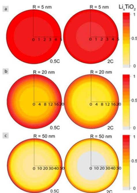
**Figure 28:** Final concentration profiles at the end of a simulation at 0.5C and 2C for particles with a radius of (a) 5, (b) 20, and (c) 50 nm.<sup>13</sup>
