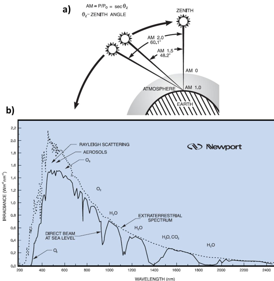
(a) the path length in units of Air Mass, changes with the zenith angle, (b) Normally incident solar spectrum at sea level on a clear day (AM 1). The dotted curve shows the extraterrestrial spectrum (AM 0).<sup>1</sup>
