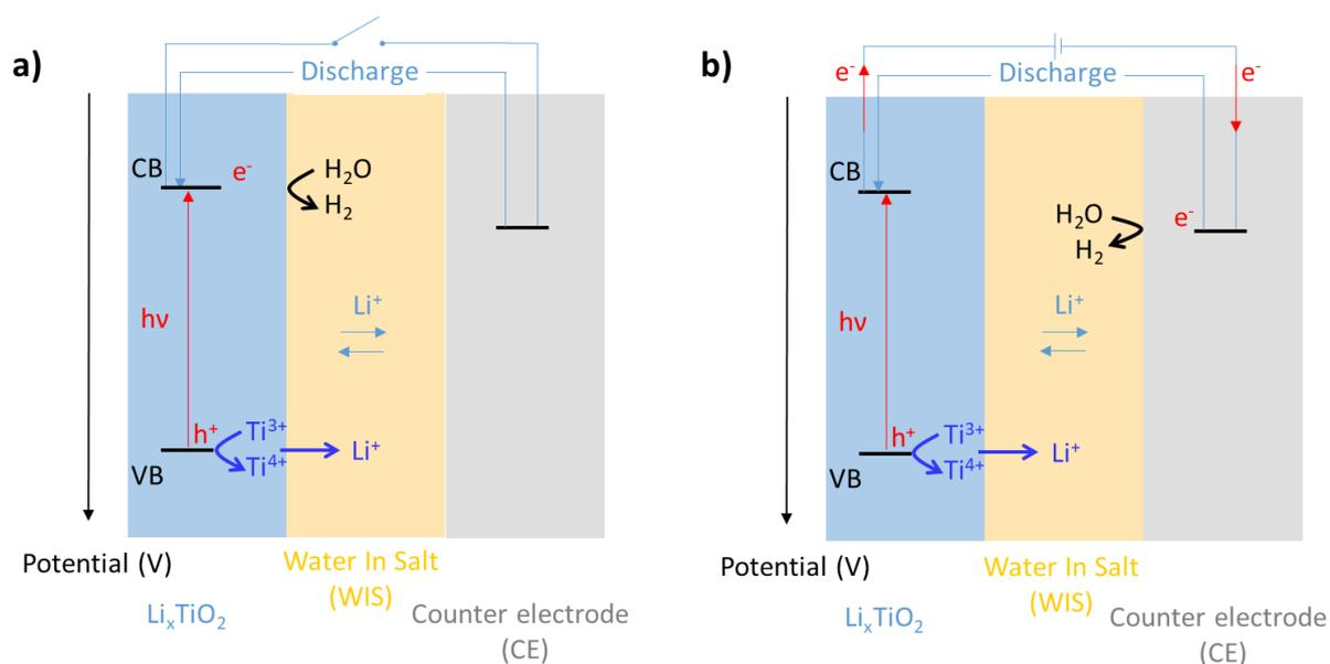
**Scheme 2:** Representation of the photo-mechanism of the of  $\text{TiO}_2// \text{LiTFSI}$  water in salt (WIS) 20 m//AgAgCl KCl saturated/ Pt half-cell for (a) a photo-charge (OCV under illumination) experiment, (b) a photo-assisted charge (galvanostatic experiment under illumination) experiment.
