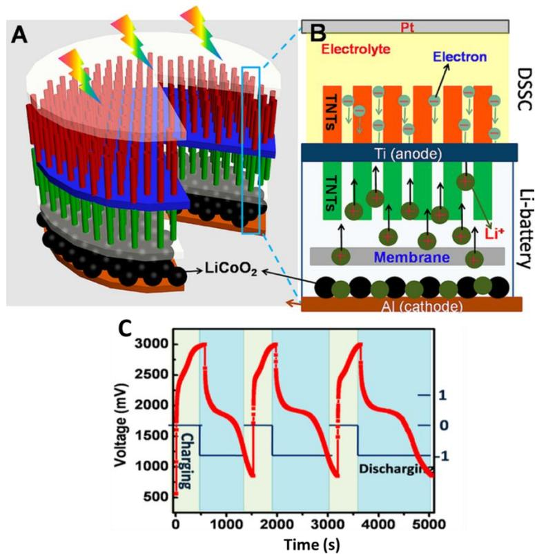
**Figure 7:** Design and principle of an integrated power pack system based on double-sided TiO<sub>2</sub> nanotube arrays. (A) TiO<sub>2</sub> nanotube arrays grown on the Ti foil substrate (B) Detailed structure and working principle of the integrated power pack system (C) Photo-charge (under open circuit voltage OCV) followed by 100  $\mu$ A discharge.<sup>39</sup>
