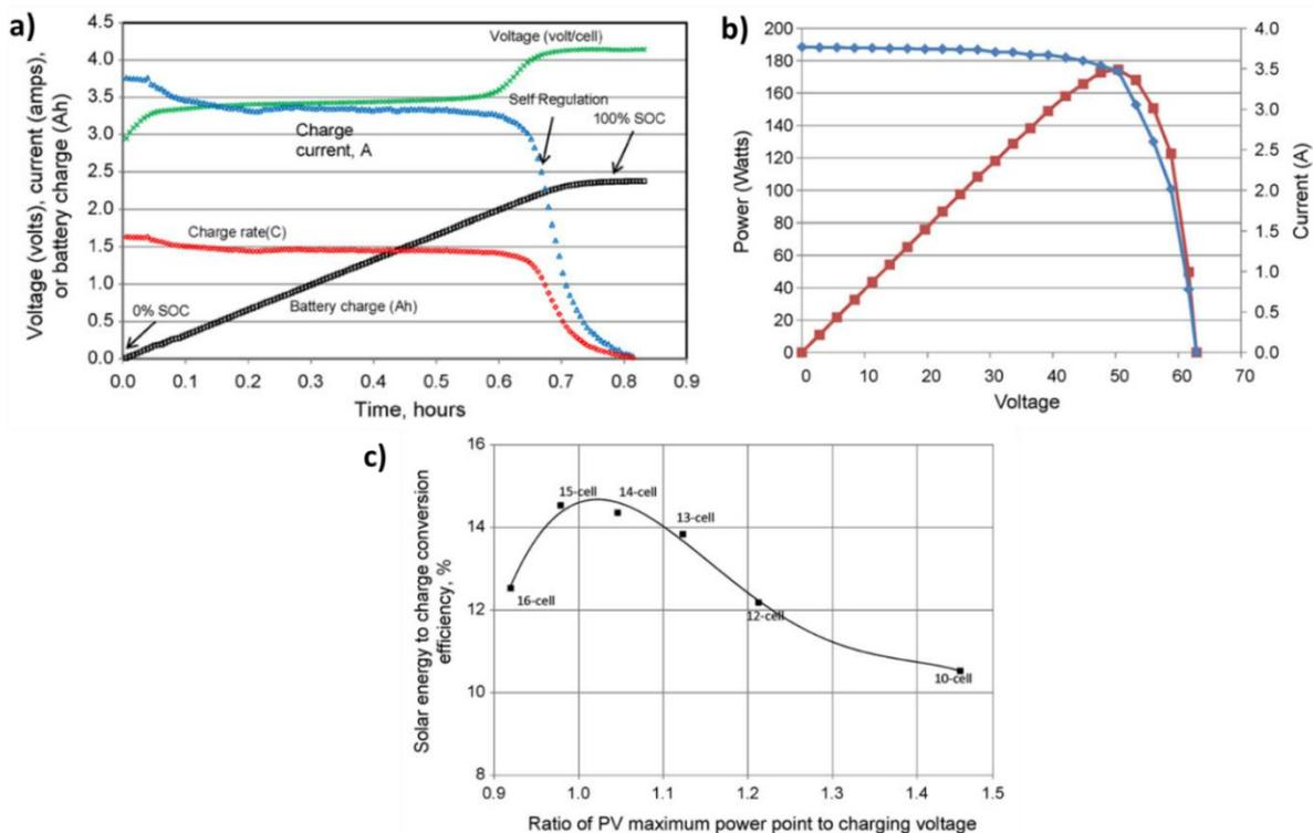
**Figure 6:** a) Solar charging of a 15-cell lithium-ion battery module—voltage per cell, current, charge rate, and battery charge capacity as a function of time, b) Current (diamonds) and power (squares) as a function of voltage for a Sanyo HIP-190BA3 module at 52 °C. c) Solar energy to battery charge conversion efficiency
