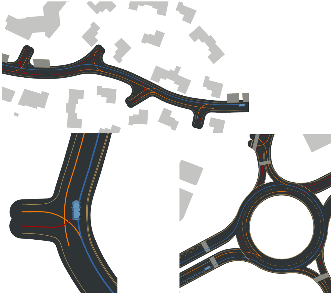
Figure 3.6: Interaction Graph models in a real-time experiment led in Compiègne. The ego-vehicle is represented in blue. The primary order lane keeping paths is represented by the blue center-line. Other primary order paths are shown in red. Secondary order paths are in orange. For visual convenience, lane changing primary order paths are not displayed. Furthermore, some paths may be both primary and secondary but are represented with only one color. (The buildings are displayed in gray)
