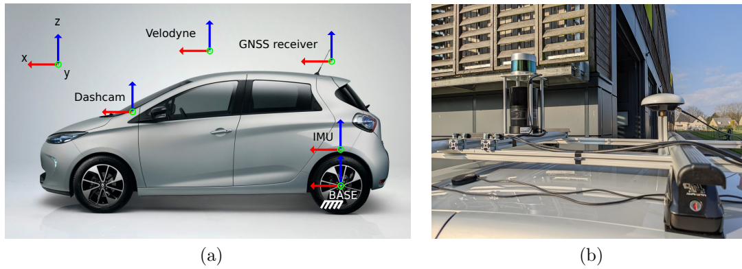
Figure A.2: Sensors setup on the ego-vehicle. (a) Sensors positioning. The origin frame corresponds to the base symbol. (b) GNSS receiver and VLP-32C sensors on the roof of a vehicle.
