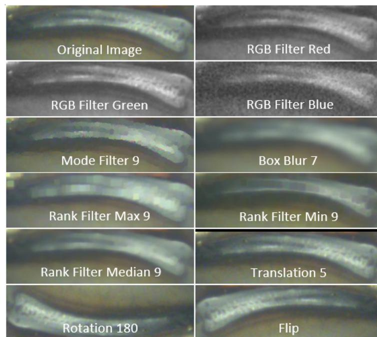
Figure 5.15: Examples of data augmentation techniques applied on weld1
