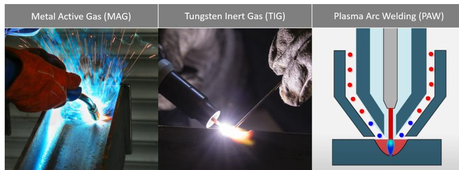
Figure 5.6: Types of welding technologies
