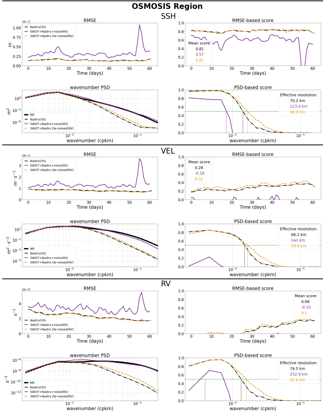
Figure 6: Comparison of BFN performance between the best nudging strategies of the Nadirs only, SWOT+Nadirs with noise and SWOT+Nadirs de-noised regimes. Plots show the time evolution of RMSE and RMSE-based score as well as the WPSD and WPSD based Score as a function of wavenumber. From top to bottom reconstructed fields of: SSH, Velocity (Vel) and Relative Vorticity (RV).
