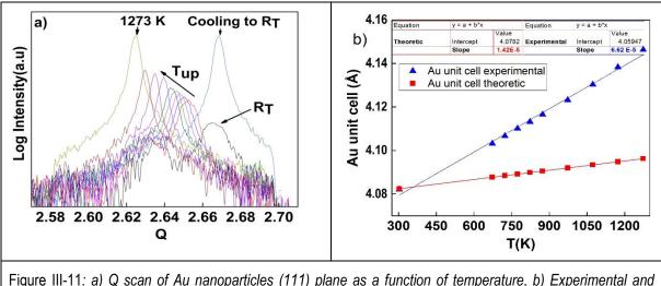
theoretical Au unit cell expansion as a function of temperature.
