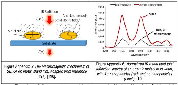
Figure Appendix 5 shows metal nanoparticles that are polarized by the incident photon field through the excitation of collective electron resonance (localized plasmon modes) and the dipole p induced in a nanoparticle generates a local electromagnetic field stronger than the incident photon field around the metal nanoparticles.
