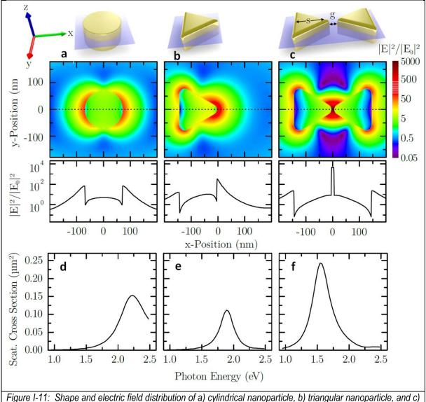
two triangular nanoparticles. Scattering cross-section for d) cylindrical nanoparticle, b) triangular nanoparticle, and c) and f) two triangular nanoparticles; Image is taken from [53].
