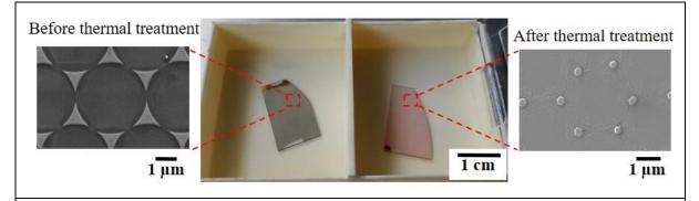
Figure III-4: Example of a sample containing Gold nanoparticles before and after a thermal treatment process (The initial factor **a**= 0.90  $\mu$ m becomes a final diameter of 0.40  $\mu$ m).
