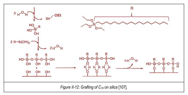
The functionalization with  $C_{18}$  takes place in two stages: first hydrolysis and then condensation, as shown in *Figure II-12* with  $C_{18}$ . Hydrolysis leads to the formation of alcohol and silanol. The condensation of silanol groups occurs on the hydroxyl sites on the microspheres' surface (in our case, polystyrene) and eventually forms covalent bonds.
