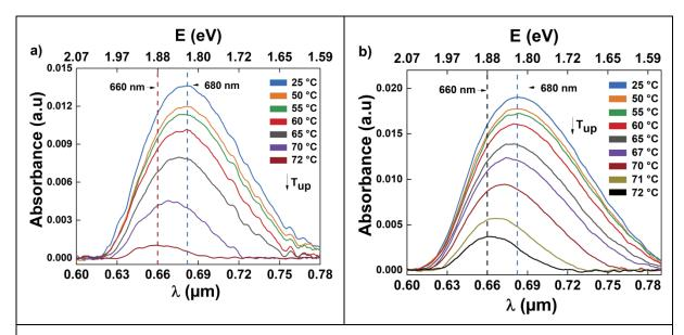
Figure IV-13: Temperature evolution of the plasmonic resonance peak located in the visible part of the electromagnetic spectrum of residue Au nanoparticles embedded into 100 nm of VO<sub>2</sub>. a) Au residue nanoparticles made by thermally treating at 532 °C; the Au nanoparticle array was made with 2  $\mu$ m polystyrene microspheres. b) Au residue nanoparticles made by thermally treating at 532 °C; the Au nanoparticle array was made with 3  $\mu$ m polystyrene microspheres.
