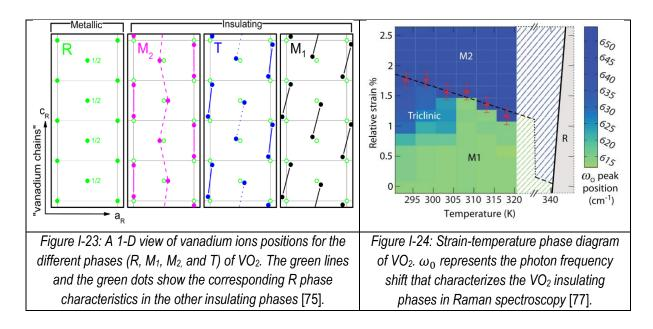
The T phase can be considered an intermediate phase between the  $M_1$  and the  $M_2$  phases (see *Figure I-23*). In T's case, the phase has two types of inequivalent vanadium chains in which the vanadium ions are tilted and paired to different degrees [75].
