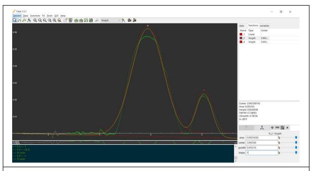
Figure IV-10: Example of resonance peak position determination of the Au nanoparticle arrays, made with 3  $\mu$ m polystyrene microspheres, and embedded into 200 nm of VO<sub>2</sub>. In this example, the experimental data (green curve) are collected at 70 °C. The baseline is subtracted from the experimental data, and a Voigt function is used for resonance peak determination.
