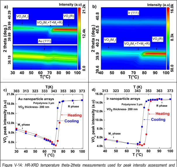
Figure V-14: HR-XRD temperature theta-2theta measurements used for peak intensity assessment and performed during heating up of 200 nm VO<sub>2</sub> containing Au nanoparticle arrays (a) and Ir nanoparticle arrays (b). c) Peak intensity evolution of VO<sub>2</sub> containing Au nanoparticle arrays, extracted using a Voigt fit of the experimental data. d) Peak intensity evolution of VO<sub>2</sub> containing Au nanoparticle arrays, extracted using a Voigt fit of the experimental data.
