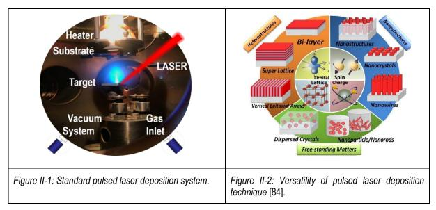
Pulsed laser deposition is a physical vapor deposition method often performed in a vacuum or a controlled environment (i.e., a gas). PLD process shares some common characteristics with molecular beam epitaxy or sputter
