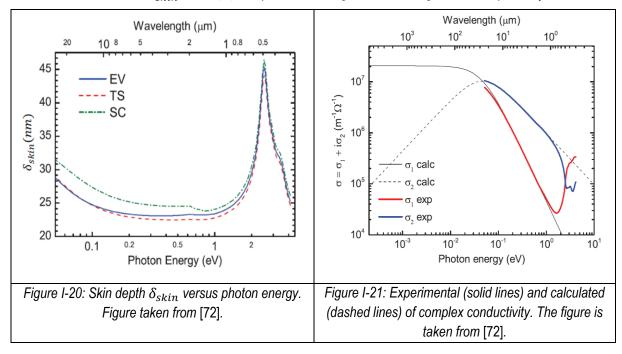
For Au thin films  $\delta_{skin}$  and  $\sigma(\omega)$  are presented in *Figure I-20* and *Figure I-21*, respectively.
