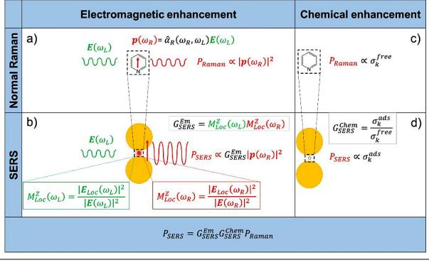
The electromagnetic and chemical enhancements are presented in Figure Appendix 3.
