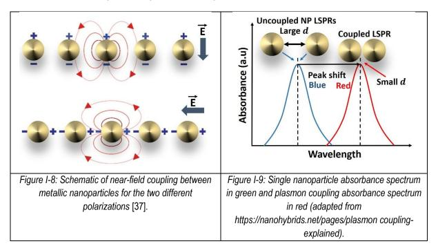
If the nanoparticles are sufficiently apart, one to each other, so that the restoring force acting on each nanoparticle is not influenced by the neighboring nanoparticles, the resonant frequency will not be affected by near-field coupling effects. Therefore, far-field dipolar coupling with a distance dependence of  $d^{-1}$  dominates. In this case, the resonant frequency is linked to Fröhlich's condition and shape-size considerations.
