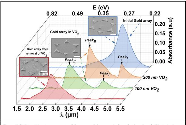
Figure IV-6: Optical absorbance spectra of Au nanoparticle arrays, before VO<sub>2</sub> deposition (in blue), in different thicknesses of the VO<sub>2</sub> matrix (200 and 100 nm, in orange and green resp.) and optical absorbance of the Au nanoparticle arrays after total removal of the VO<sub>2</sub> matrix (in red). The optical measurements are performed by FTIR spectroscopy on Au nanoparticle arrays made with 3  $\mu$ m polystyrene microspheres,
