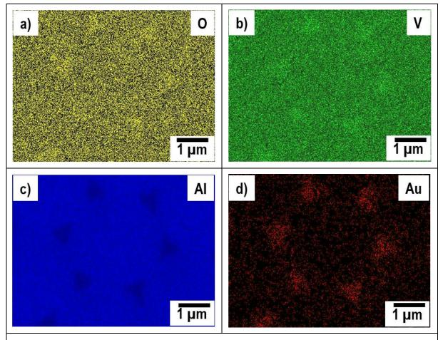
Figure V-2: Elemental mapping of a sample consisting of Au nanoparticle arrays made with 3 µm polystyrene microsphere and embedded into 200 nm of VO2. a) Elemental map of Oxygen. b) Elemental map of Vanadium. c) Elemental map of Aluminum. d) Elemental map of Iridium.
