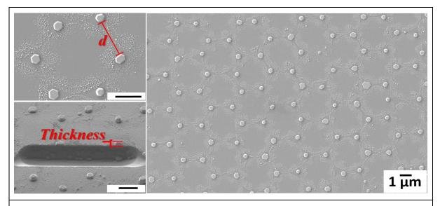
Figure III-7: SEM-FIB image of Au nanoparticle arrays after thermal treatment in a conventional furnace at 1000 °C (1273 K).
