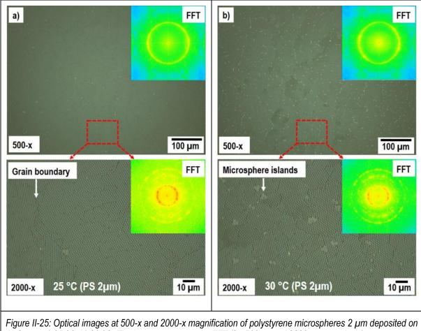
Al<sub>2</sub>O<sub>3</sub>-c at a) 25 °C, b) 30 °C. The inserts represent the FFT (for 500 –x and 2000-x respectively).
