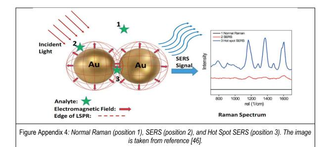
The electric field distribution at a surface of a plasmonic element (substrate, nanoparticle) is highly inhomogeneous, and in the case of nanoparticles, the field can be localized in the small spatial regions called "**hot spots**".
