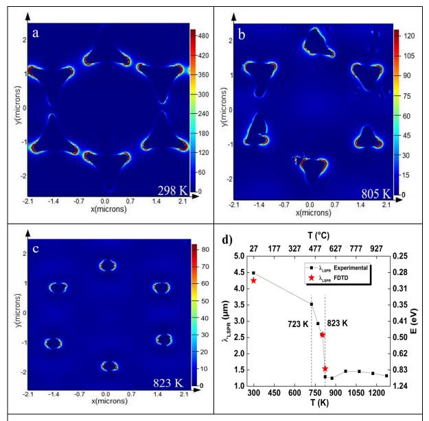
Figure IV-2: a-c: Electric field cartography, obtained by FDTD, of LSPR of Au nanoparticles arrays as a function of thermal treatment temperature a) at  $\lambda$ =4.45 µm for RT sample b)  $\lambda$ =2.58 µm for sample treated at 805 K and c)  $\lambda$ =1.54 µm for sample treated at 823 K d) Evolution of the LSPR position - Comparison between experimental and theoretical (FDTD) values. The FDTD calculation at 1273 K (lambda LSPR = 1.59) are written in the Table IV 1.
