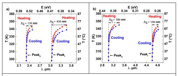
Figure IV-15: a) Temperature evolution of resonance peak of Au nanoparticle arrays made with 2  $\mu$ m polystyrene microspheres thermally treated at 532 °C and then covered by 100 nm of VO<sub>2</sub>. b) Temperature evolution of resonance peaks of Au nanoparticle arrays made with 3  $\mu$ m polystyrene microspheres thermally treated at 532 °C then covered by 100 nm of VO<sub>2</sub>.
