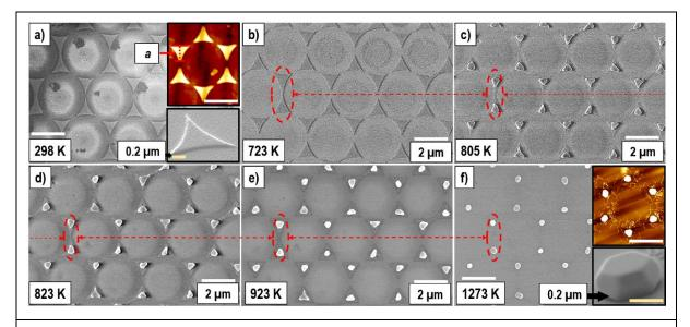
Figure III-6: Dewetting of Au nanoparticle, with a thickness of 50 nm and initial **a**=0.90  $\mu$ m on an Al<sub>2</sub>O<sub>3</sub>-c substrate. The thermal treatment is made in furnace inside a SEM system. The starting temperature is R<sub>T</sub> and the process stops at 1273 K or 1000 °C. The white scale bar is 2  $\mu$ m and the yellow one is 0.2  $\mu$ m. The inserts are AFM and SEM-FIB analyses of samples submitted to conventional thermal treatment (see also SEM movie).
