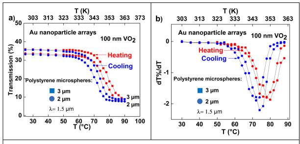
Figure V-7: a) Optical transmission of 100 nm VO<sub>2</sub> thin films that contain Au nanoparticles arrays made with 2 and 3  $\mu$ m polystyrene microspheres and thermally treated at 532 °C before VO<sub>2</sub> deposition. b) Derivatives of the temperature dependence of optical transmission of 100 nm VO<sub>2</sub> thin films that contain Au nanoparticles arrays made with 2 and 3  $\mu$ m polystyrene microspheres and thermally treated at 532 °C before VO<sub>2</sub> deposition.
