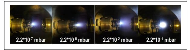
Figure II-7: Plasma plume dynamics of vanadium metal at different oxygen pressures. The ablation was made with a KrF excimer laser at a fluence of 3 J/cm<sup>2</sup>.
