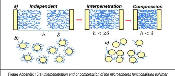
chains, b) and c) Possible bridging interactions between the polymer chains [114].
