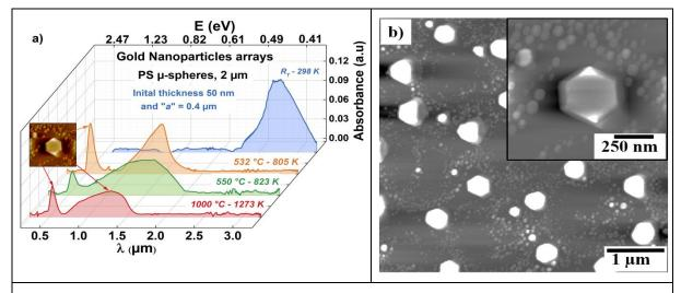
Figure III-13: Effect of the thermal treatment on Au nanoparticle arrays deposited on an  $AI_2O_3$ -c substrate and made with 2  $\mu$ m polystyrene microspheres. a) Absorbance spectrum pointing out the wavelength blue shift. b) Au nanoparticle array made with 2  $\mu$ m polystyrene microspheres and thermally treated at 1000°C (1273 K).
