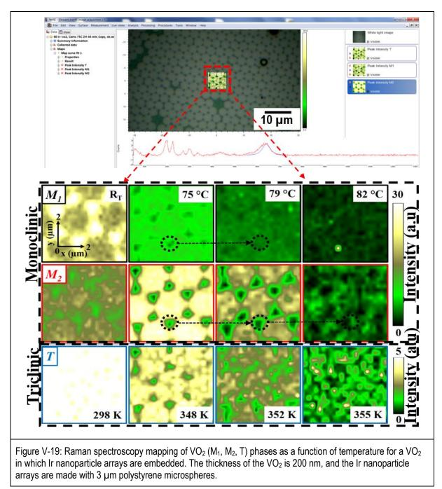
Figure V-19 shows that the Raman mapping result obtained for  $VO_2$  containing Ir nanoparticles is similar to that of  $VO_2$  with Au nanoparticles inside. The Raman mapping's proves that the  $VO_2$  in the immediate vicinity of
