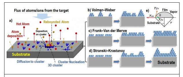
Figure II-8: Basic atomistic nucleation process. a) Thin film growth, b) Volmer–Weber (island), c) Frank–Van der Merwe (layer-by-layer), and d) Stranski–Krastanov growth, e) Interfacial tensions between the thin film, vapor, and substrate [95], Picture a) is adapted from https://www.bnl.gov/ nsls2/sciOps/chemSci/growth.asp.
