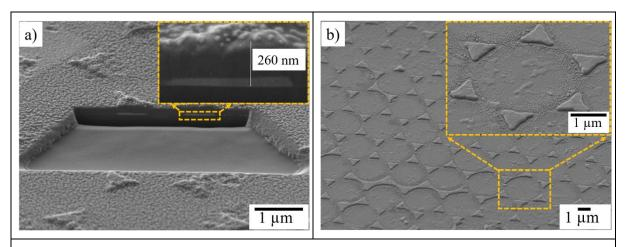
Figure IV-5: Gold nanoparticle array embedded into a VO<sub>2</sub> matrix. a) FIB image of gold nanoparticle arrays with 200 nm VO<sub>2</sub> matrix. b) FIB image taken after removing the VO2 matrix (by chemical etching). The initial thickness of the Au nanoparticles, made with 3  $\mu$ m polystyrene microspheres, is 50 nm. For FIB measurements, a 20 nm layer of Platinum was deposited on top of the samples by thermal evaporation.
