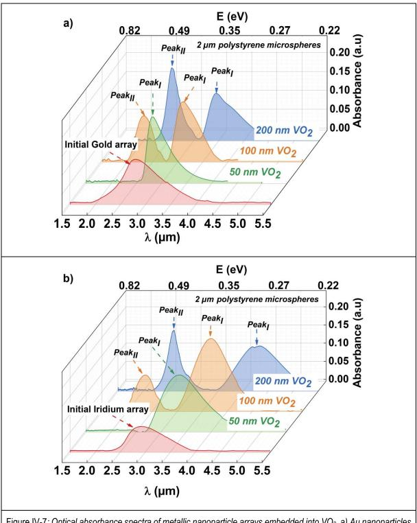
Figure IV-7: Optical absorbance spectra of metallic nanoparticle arrays embedded into VO<sub>2</sub>. a) Au nanoparticles with 50, 100, and 200 nm of VO<sub>2</sub>. b) Ir nanoparticles with 50, 100, 200 nm of VO<sub>2</sub>, The FTIR measurements are made on metallic nanoparticles made with 2  $\mu$ m polystyrene microspheres and with initial thickness of 50 nm.
