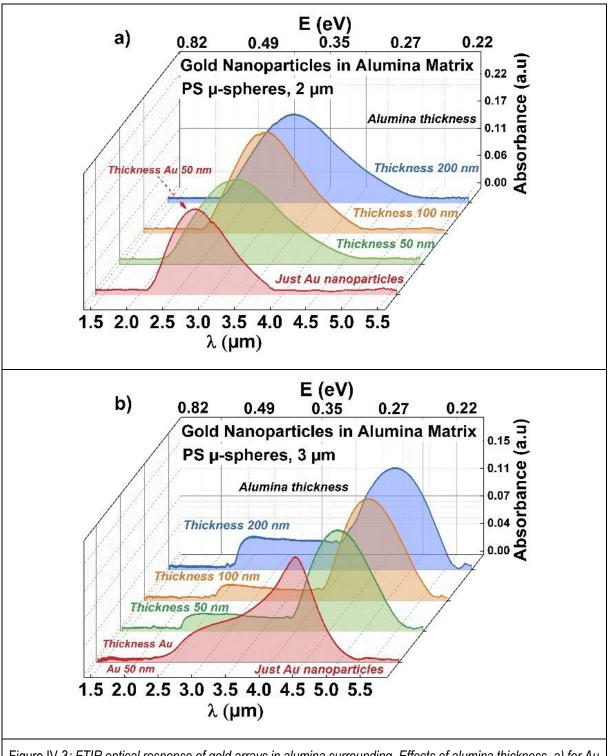
Figure IV-3: FTIR optical response of gold arrays in alumina surrounding. Effects of alumina thickness. a) for Au nanoparticle array made with 2  $\mu$ m polystyrene microspheres. b) for Au nanoparticle array made with 3  $\mu$ m polystyrene microspheres.
