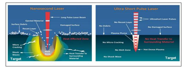
Figure Appendix 11: Nanosecond laser ablation vs femtosecond laser ablation. Source: https://www.ipgphotonics.com/en/products/lasers/pico-femtosecond-fiber-lasers/1-03-1-06-micron/ylpp-r-series#[nanosecond-vs-ultra-short-pulse].
