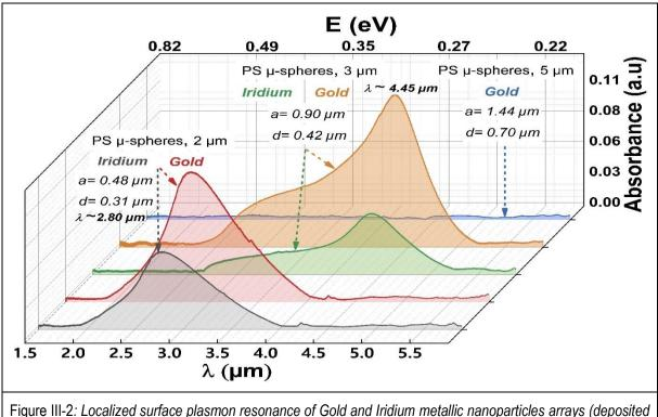
on an Al<sub>2</sub>O<sub>3</sub>-c substrate) as a function of the diameter of the polystyrene microsphere used in the Langmuir-Blodgett process.
