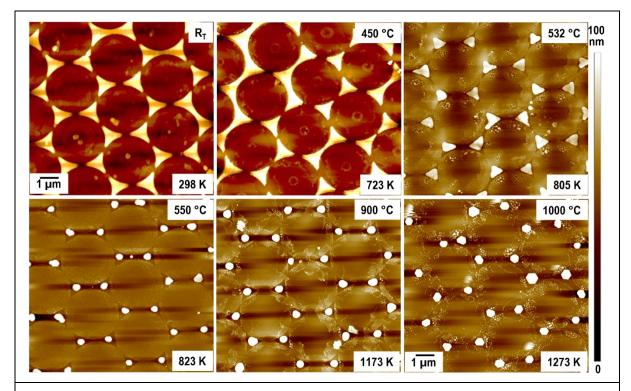
Figure III-5: Conventional thermal treatment of Au nanoparticle array made with 3  $\mu$ m polystyrene microspheres and initially having a=0.90  $\mu$ m and a thickness of 50 nm. The thermal treatment starts every time with a sample made at room temperature.
