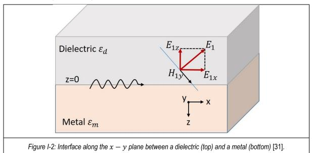
The conditions for the continuity of the normal and transversal field components on this interface are given by the following equations [31]:
