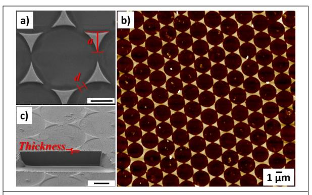
Figure III-1: a) Scanning electron microscopy picture of Au nanoparticle showing the nanoparticles characteristic size **a** and the distance tip to tip **d** between two adjacent nanoparticles. b) AFM image of the global nanoparticle arrays. c) Focused ion beam scanning electron microscopy image used for nanoparticle's precise thickness quantification.
