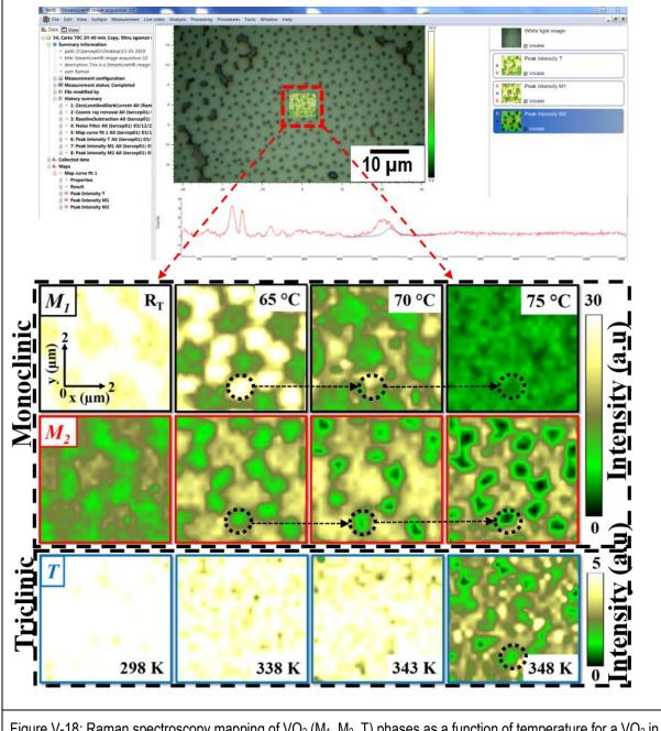
Figure V-18: Raman spectroscopy mapping of VO<sub>2</sub> (M<sub>1</sub>, M<sub>2</sub>, T) phases as a function of temperature for a VO<sub>2</sub> in which Au nanoparticle arrays are embedded. The thickness of the VO<sub>2</sub> is 200 nm, and the Au nanoparticle arrays are made with 3  $\mu$ m polystyrene microspheres.
