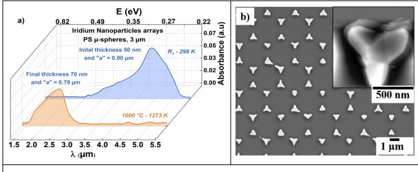
Figure III-14: Thermal treatment of the Iridium nanoparticle arrays. a) Optical absorbance of the Ir nanoparticle arrays before and after thermal treatment at 1000 °C. b) SEM image of Iridium nanoparticle arrays thermally treated at 1000 °C.
