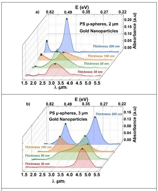
Figure III-3: Influence of metallic thickness on the Localized surface plasmon resonance of Gold metallic nanoparticles arrays: a) and b) Au nanoparticles arrays made with 2, respectively 3  $\mu$ m polystyrene microspheres; "o" ( $\lambda_{max1}$ ) corresponds to dipole resonances while "x" corresponds to the resonances ( $\lambda_{max2}$ ) given by the thickness. All samples are made on the Al<sub>2</sub>O<sub>3</sub>-c substrate
