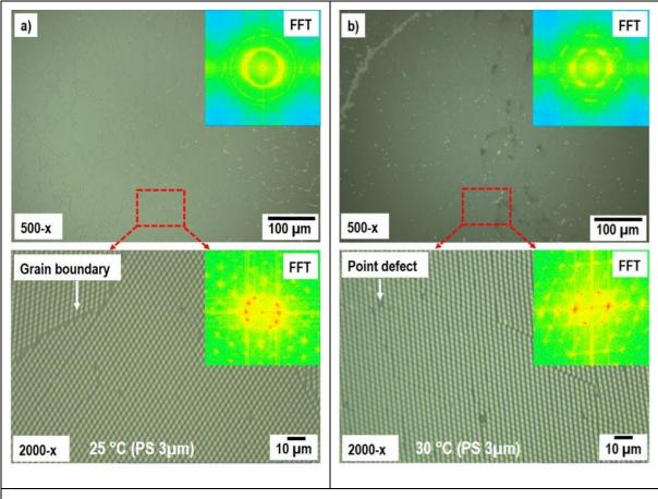
Figure II-24 Optical images at 500-x and 2000-x magnification of polystyrene microspheres 3  $\mu$ m deposited on Al<sub>2</sub>O<sub>3</sub>-c at a) 25 °C, b) 30 °C. The inserts represent the FFT (for 500 –x and 2000-x respectively).
