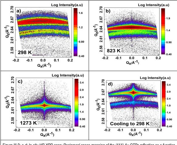
Figure III-9: a-d: In-situ HR-XRD scan; Reciprocal space mapping of the (111) Au QTPs reflection as a function of the terminal treatment temperature, from (a)room temperature up to (c)1000 °C (1273 K) and back to room temperature(d). The maps are plotted as a function of the diffraction space coordinates  $Q_z$  and  $Q_x$ .
