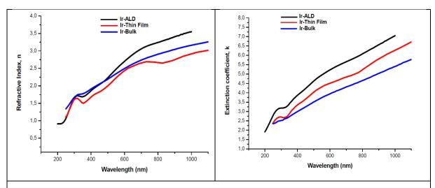
Figure I-16: Refractive index n (left) and Extinction coefficient k (right) of Ir thin films compared to the n and k of bulk Ir [64]. The Ir-ALD represents an 20 nm Ir thin film deposited on BK7. The Ir-Thin film represents a 115 nm thin film deposited by electron beam evaporation on a fussed silica substrate. And Ir-Bulk characterizes the optical characteristics measured on bulk Iridium.
