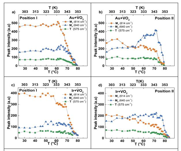
Figure V-17: The evolution of Raman peak vibrations intensity of VO<sub>2</sub> M<sub>1</sub>, M<sub>2</sub>, and T phases, extracted using a mix function (Gauss and Lorentz), as a function of temperature. a-b) The intensity of VO<sub>2</sub> phases containing Au nanoparticle arrays (Position "I" and "II"). c-d) The intensity of VO<sub>2</sub> phases containing Ir nanoparticle arrays (Position "I" and "II"). The data are collected during heating.
