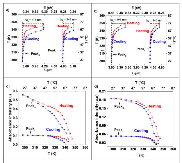
Figure IV-11: Temperature evolution of a) resonance peaks wavelength of Au nanoparticle arrays in 200 nm VO<sub>2</sub> matrix. b) resonance peaks wavelength of Au nanoparticle in 100 nm VO<sub>2</sub> matrix. c) resonance peaks intensity of Au nanoparticle arrays in 200 nm VO<sub>2</sub> matrix. d) resonance peaks intensity of Au nanoparticle arrays in 100 nm VO<sub>2</sub> matrix. Au nanoparticles are made with 3  $\mu$ m polystyrene microspheres and thickness of 50 nm in both cases.
