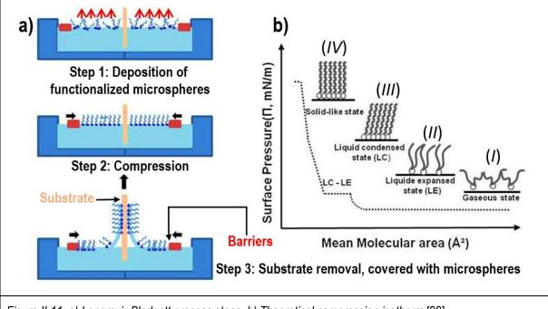
The Langmuir-Blodgett process is controlled by compression isotherm as presented in Figure II-11 b).
