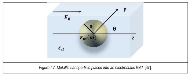
Since we assume that the space inside and outside the metallic nanoparticle is free of charges, the electrostatic problem can be solved by using the Laplace equation for the potential  $\nabla^2 \Phi = 0$  to deduce the electric field  $\vec{E} = -\vec{\nabla} \Phi$ , with the general solution given by Equation (1.25) (for a detailed description, see [39]).
