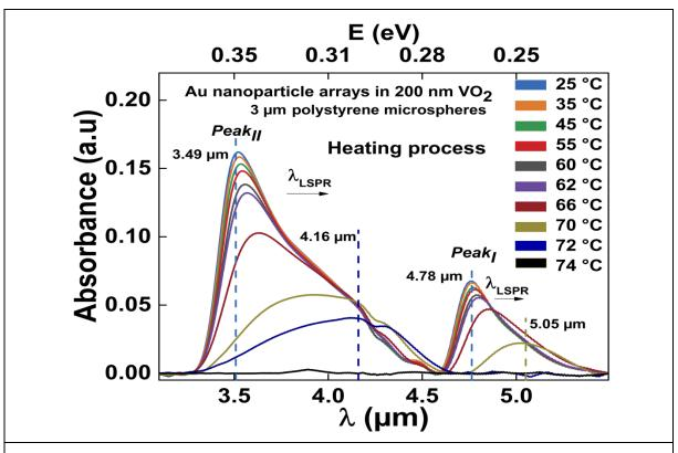
Figure IV-9: Optical absorbance spectra of Au nanoparticle arrays embedded into a 200 nm VO<sub>2</sub>, as a function of the temperature matrix. The Au nanoparticles are made using 3  $\mu$ m polystyrene microspheres and have an initial thickness of 50 nm. The data are measured by FTIR spectroscopy, and the baseline was subtracted using OriginPro 2015 software.
