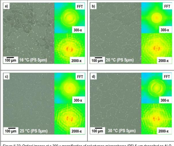
Figure II-23: Optical images at a 300-x magnification of polystyrene microspheres (PS) 5  $\mu$ m deposited on Al<sub>2</sub>O<sub>3</sub> -c at a) 16 °C, b) 20 °C, c) 25 °C, c) 30 °C. The inserts represent the FFT (for 300 –x and 2000-x respectively).
