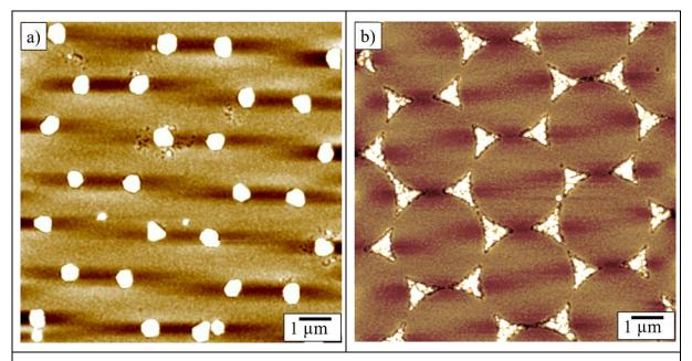
Figure IV-4: AFM image of metallic nanoparticle array embedded into a 200nm-VO<sub>2</sub> matrix. a) gold nanoparticle arrays. b) Iridium nanoparticle arrays. The initial thickness of the Au and Ir made with 3  $\mu$ m polystyrene microspheres nanoparticles is 50 nm.
