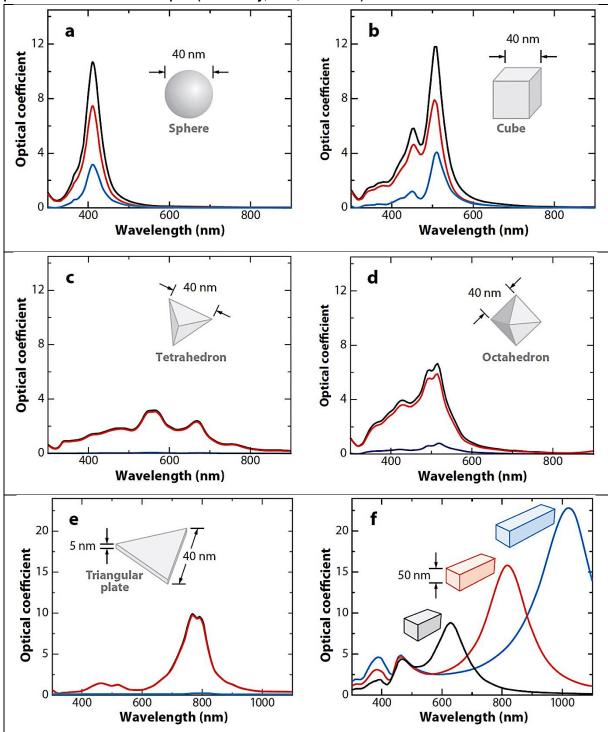
I.2.4. LSPR theoretical spectra of nanoparticles with different shapes, obtained by implementing the plasmonic simulation techniques (Mie Theory, DDA, and FDTD)
