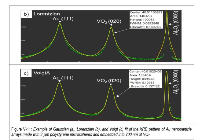
In Scherrer's formula, the k parameter is linked to the function used in fitting the data and is equal to 0.9 for a Gaussian fit, 0.64 for a Lorentzian fit. However, when using a Voigt fit, we must use the Stokes and Wilson formula [177]:
