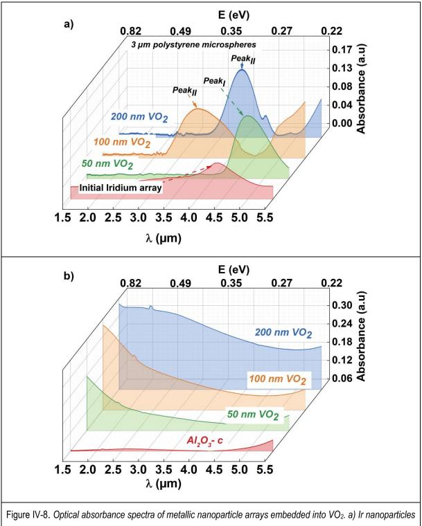
with 50, 100, and 200 nm of VO<sub>2</sub> made with 3  $\mu$ m polystyrene microspheres and an initial thickness of 50 nm. b) Optical absorbance of VO<sub>2</sub> thin films with thickness 50, 100, and 200 nm and of the Al<sub>2</sub>O<sub>3</sub>-c substrate. These contributions were extracted to obtain the spectra in Figure IV-6, Figure IV-7and Figure IV-8.a. The measurements are made by FTIR.
