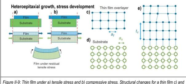
a substrate, d) within an epitaxial over layer structure. e) Strain relaxation with a thickness (the relaxation is elastic until a critical layer thickness ( $t_c$ ), after which plastic relaxation starts via the introduction of heteroepitaxy edge dislocations) [96].
