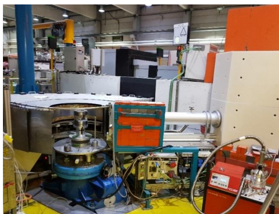
Figure 30. Instrument layout of the D1B diffractometer at the ILL (top) and the actual experimental set-up (bottom). Small inset shows a sample diffraction pattern. Radial oscillating collimator eliminates parasitic diffraction. Image taken from ILL website.
