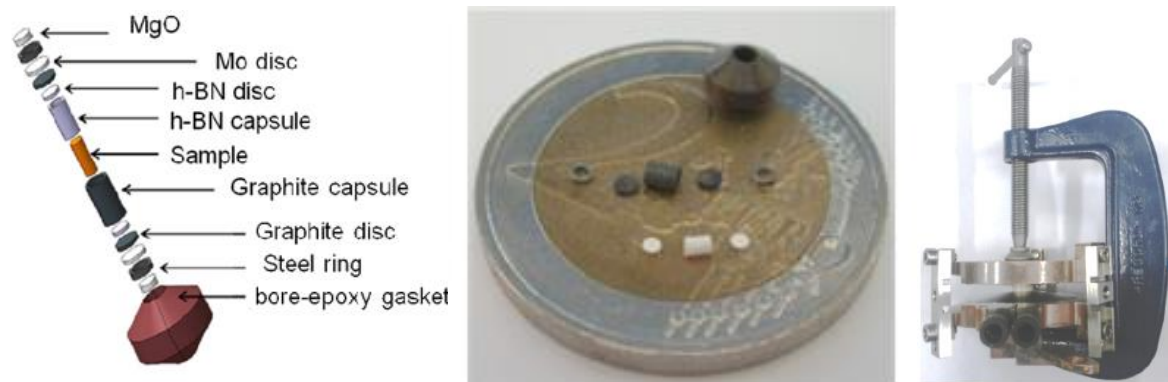
Figure 25. The different components in the assembly shown as arranged (left photo) and how they look like using a coin as a scale (middle photo) and clamped anvils with the sample in the middle (right photo)
