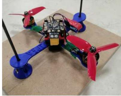
Figure D.3: 1(2)-DOF(s) Bi-rotor platform
