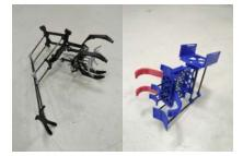
Figure D.6: Aerial mechanical gripper
