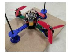
Figure D.3: 1(2)-DOF(s) Bi-rotor platform
