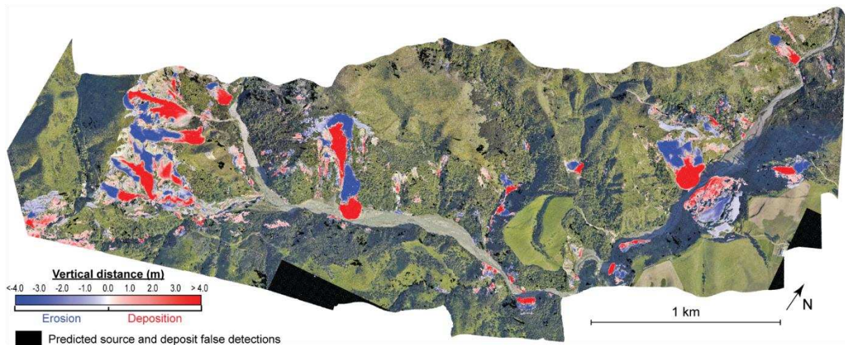
Figure 3.11 - Map of the 3D-predicted inventory with vertical-M3C2 distances after the application of TCDD = 18m and TSNR = 1.45 in forest-free areas and TCDD = 28m in forested areas. The landslide inventory is overlaid on the post-EQ orthoimagery (15 December 2016, Aerial Surveys, 2017). Landslide sources are in blue, and landslide deposits are in red.
