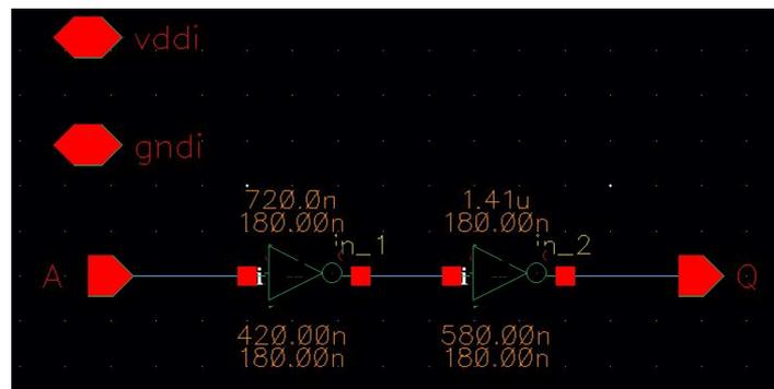
Figure 6.16: Schematic of the buffer (BUFx1)
