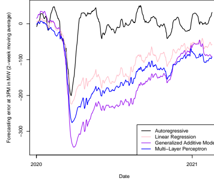
Figure 8.5 – Evolution of the forecasting error for the different models introduced in Section 8.3 trained on the data up to January 1 st 2020.
