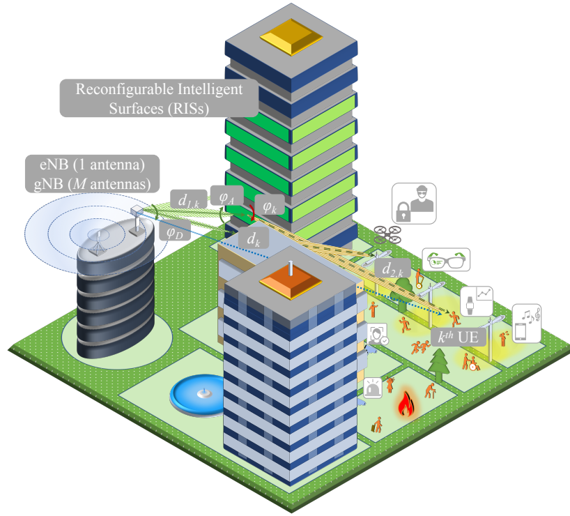
Figure 7.1 – Radio massive access scenario overcoming NLoS issues by means of RISs installed on the building glasses. It might support different use cases, such as Augmented Reality (AR)-glasses, e-health, video-surveillance, Industrial-IoT
