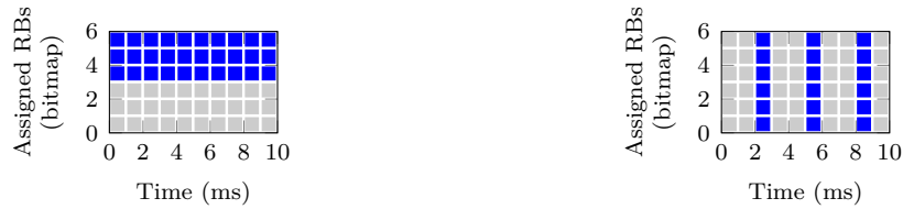
(a) Static slicing; each slice has 3 assigned RBs each slot. (b) Slicing using NVS; slices have 33% and 66% resources over 10 ms.
