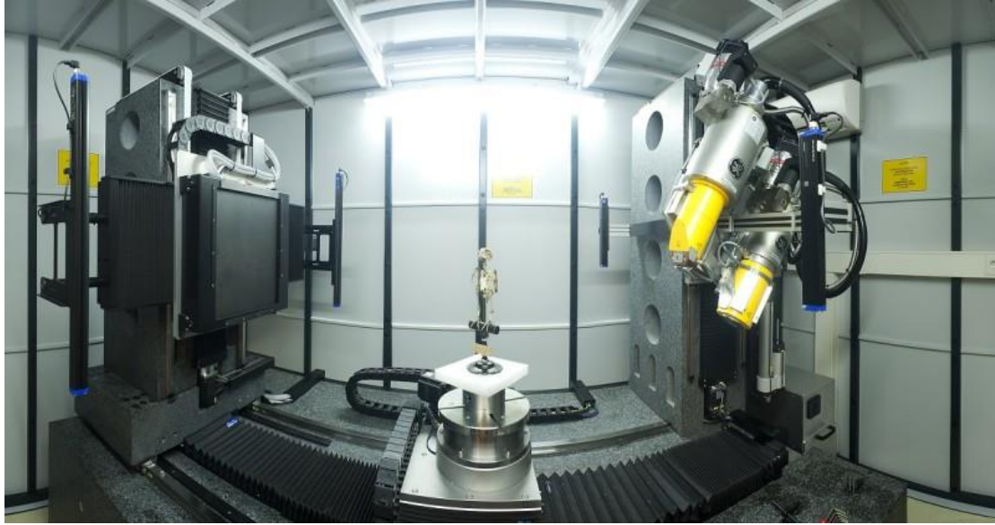
Fig. 2-24. X-ray tomography set-up in the AST-RX platform.
