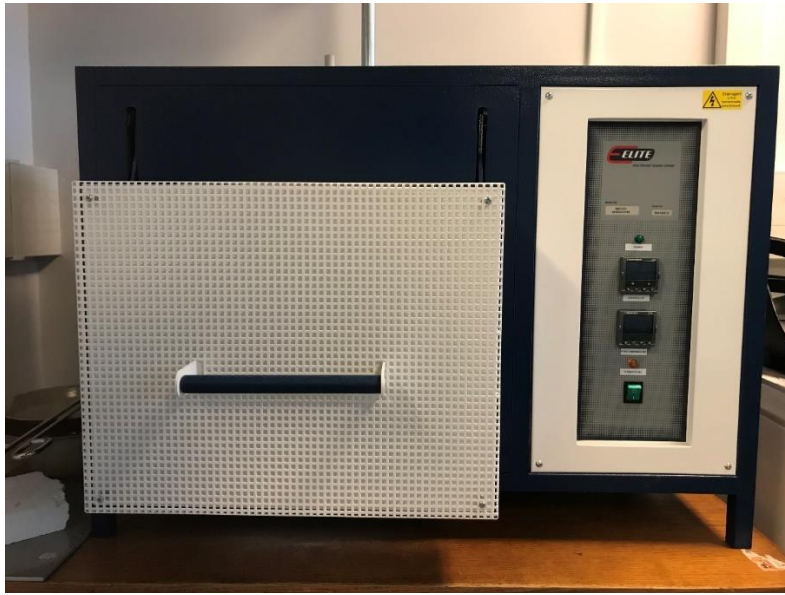
Fig. 2-2. Photo of BRF17/5 furnace used in our experiments.
