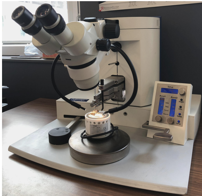
Figure 2.10: Photo of the wire bonding machine used in this thesis.
