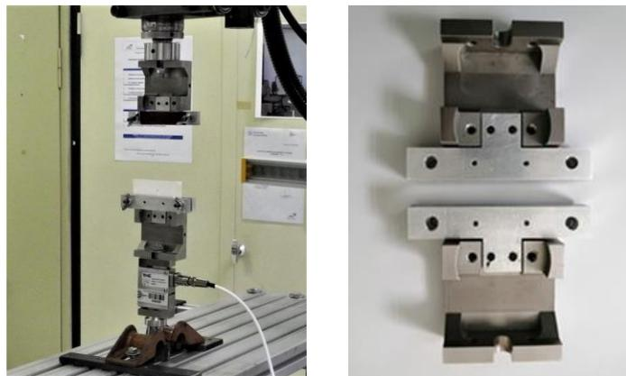
Figure 3.2-4. The configurations of the loading cell on the INSTRON machine (on the left) and the fixture (on the right) for the bias and large band tests.
