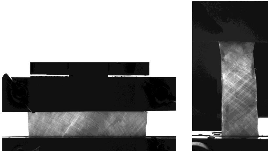
Figure 3.2-7. Example of an image (0% strain) obtained for the observation of fibers for the large band test (left) (sample 133\_L\_03) and bias test (right) (front face of sample 107\_L\_07).
