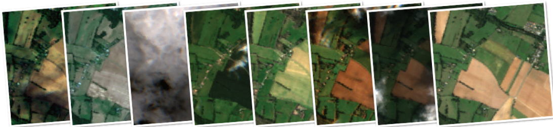
Figure 4: Multispectral image time series. Sentinel-2 image time series of the same zone across the year 2019 (RGB bands shown only). Note the evolution of the agricultural parcels' appearance. This sample time series also highlights the problem of clouds that can partially (fourth and seventh observation) or totally (third observation) occlude the acquisition.
