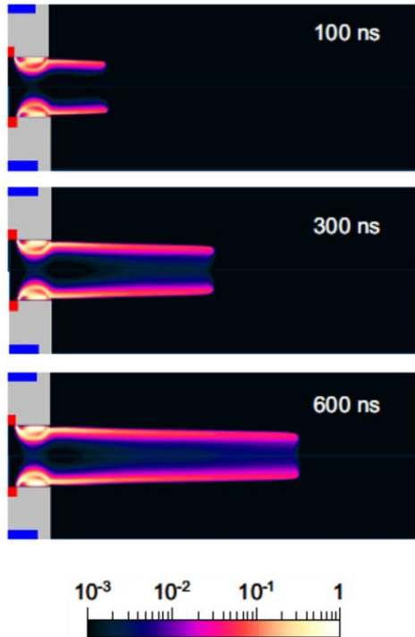
Figure 2.7 This demonstration electron distribution used the same configuration as Figure 2.6. The units of the electron density are 5 \times 10^{13} \text{ cm}^{-3} , 3 \times 10^{13} \text{ cm}^{-3} , 2 \times 10^{13} \text{ cm}^{-3} at 100 ns, 300 ns and 600 ns [154].
