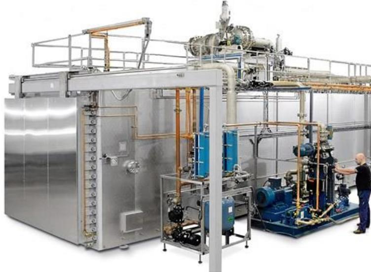
Figure 1.5 The ethylene oxide sterilization chamber [42].
