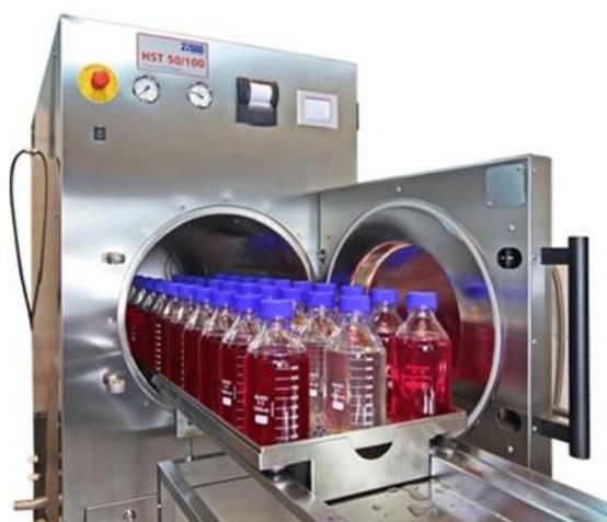
Figure 1.3 The autoclave and sterilized items (medium) [39].
