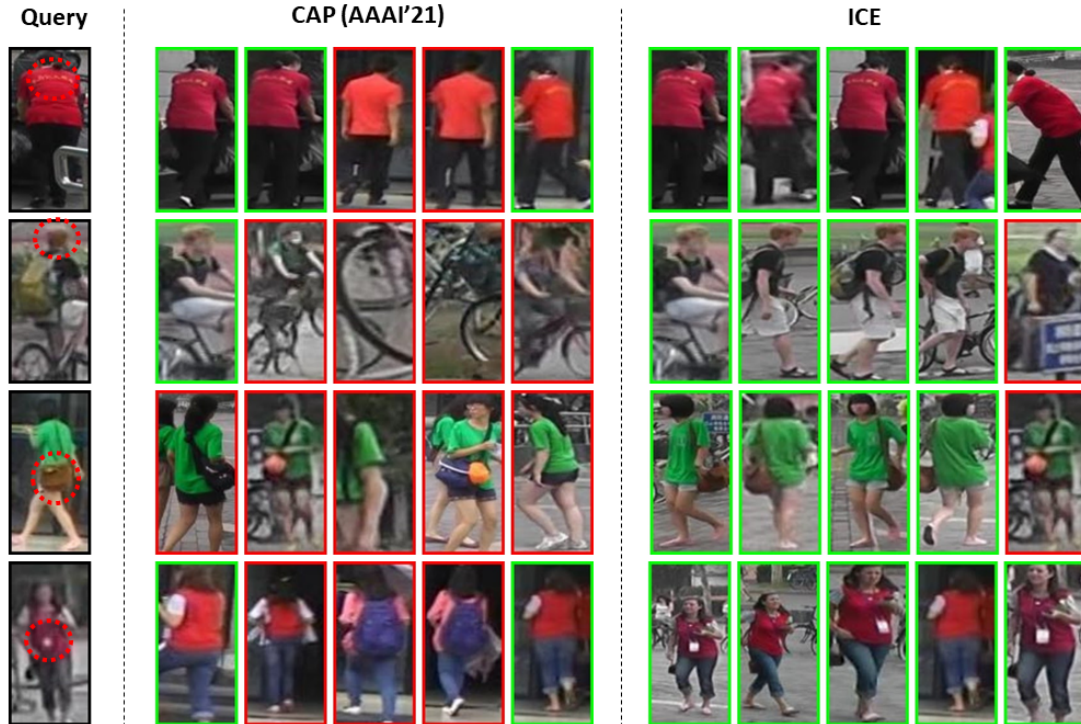
Figure 6.10: Comparison of top 5 retrieved images on Market1501 between CAP [130] and ICE. Green boxes denote correct results, while red boxes denote false results. Important visual clues are marked with red dashes.
