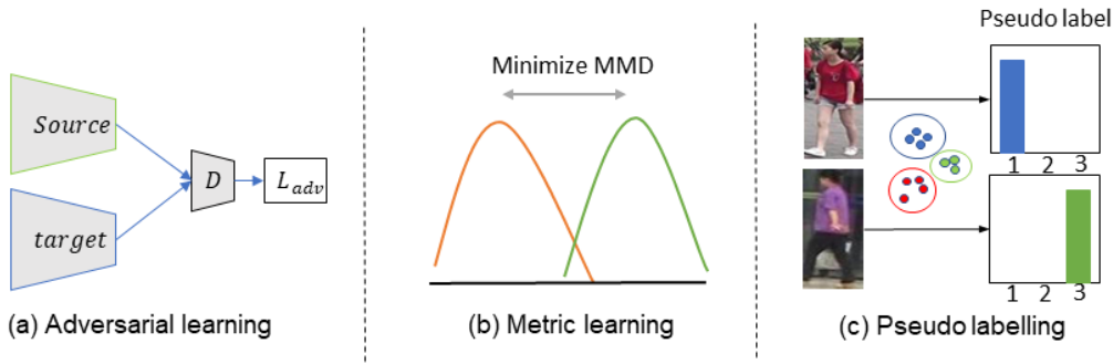
Figure 2.8: Three main approaches for unsupervised person ReID: (a) Adversarial learning, (b) Metric learning and (c) Pseudo labelling.
