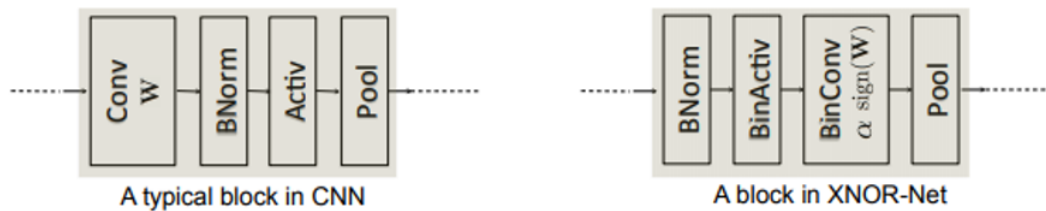
Figure 3.6: A CNN block (left) vs a XNORNET block (right) [Rastegari et al., 2016]. In a typical CNN block, the order of operations is the following: CONV, Batch Norm, activation function. In a XNORNET block, the input is first normalized and, then, we apply a binary activation and a binary CONV. The Pooling operation is in the last position in both cases.
