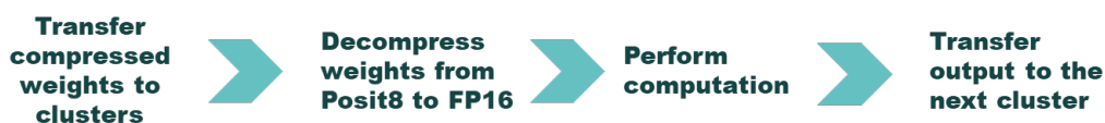
Figure 6.2: Runtime steps. The weights are compressed during pre-processing. At runtime, the compressed weights are transferred from the external memory of the platform to internal memory of each cluster. After the transfer, they are decompressed and the computation is performed. Finally, the output given by the computation is transferred to the next cluster
