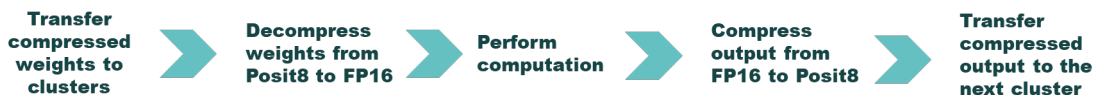
Figure 6.5: Runtime steps. The weights are compressed during pre-processing. At runtime, the compressed weights are transferred from the external memory of the platform to internal memory of each cluster. After the transfer, they are decompressed and the computation is performed. The output of the computation is compressed and ready to be transferred to the next cluster.
