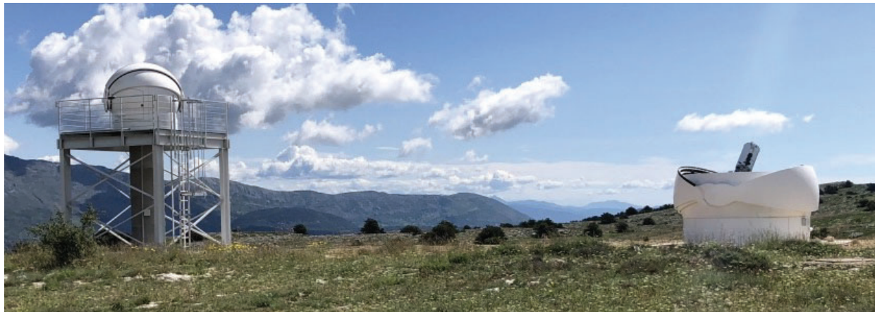
Figure 1. CATS station installed on the Calern Observatory. The left instrument is the G-DIMM, and the right one is the PML.
