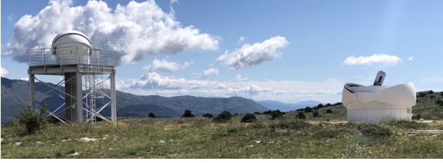
Figure 3. Calern Atmospheric Turbulence Station (CATS). The generalized differential image motion monitor (GDIMM) installed on a 4-m tower can be seen on the left, and the profiler of moon limb (PML) instrument observing the Sun limb can be seen on the right.
