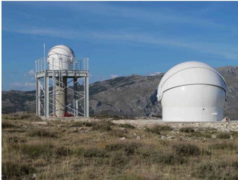
Figure 1. CATS station installed on the Calern Observatory. The left instrument is the G-DIMM, and the right one is the PML.
