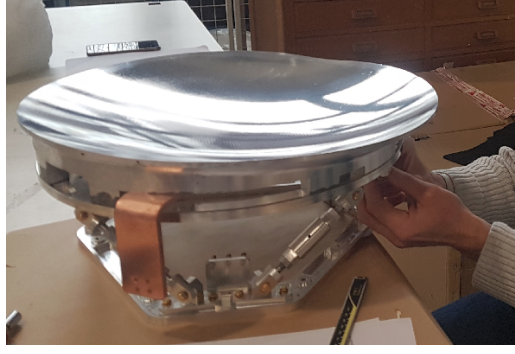
Figure 1.7: TD primary mirror being mounted on its adjustable support (hexapode).
