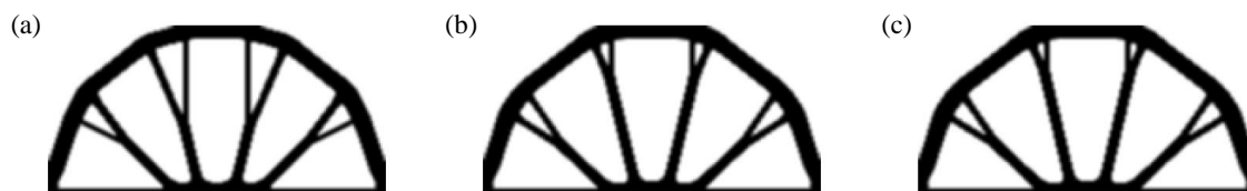
Fig. 4.10 Topological designs for uncertain loads with different spatial correlation lengths: (a) Deterministic design ( l_x = \infty , for comparison); (b) Robust design ( l_x = 30 ); (c) Robust design ( l_x = 120 ).
