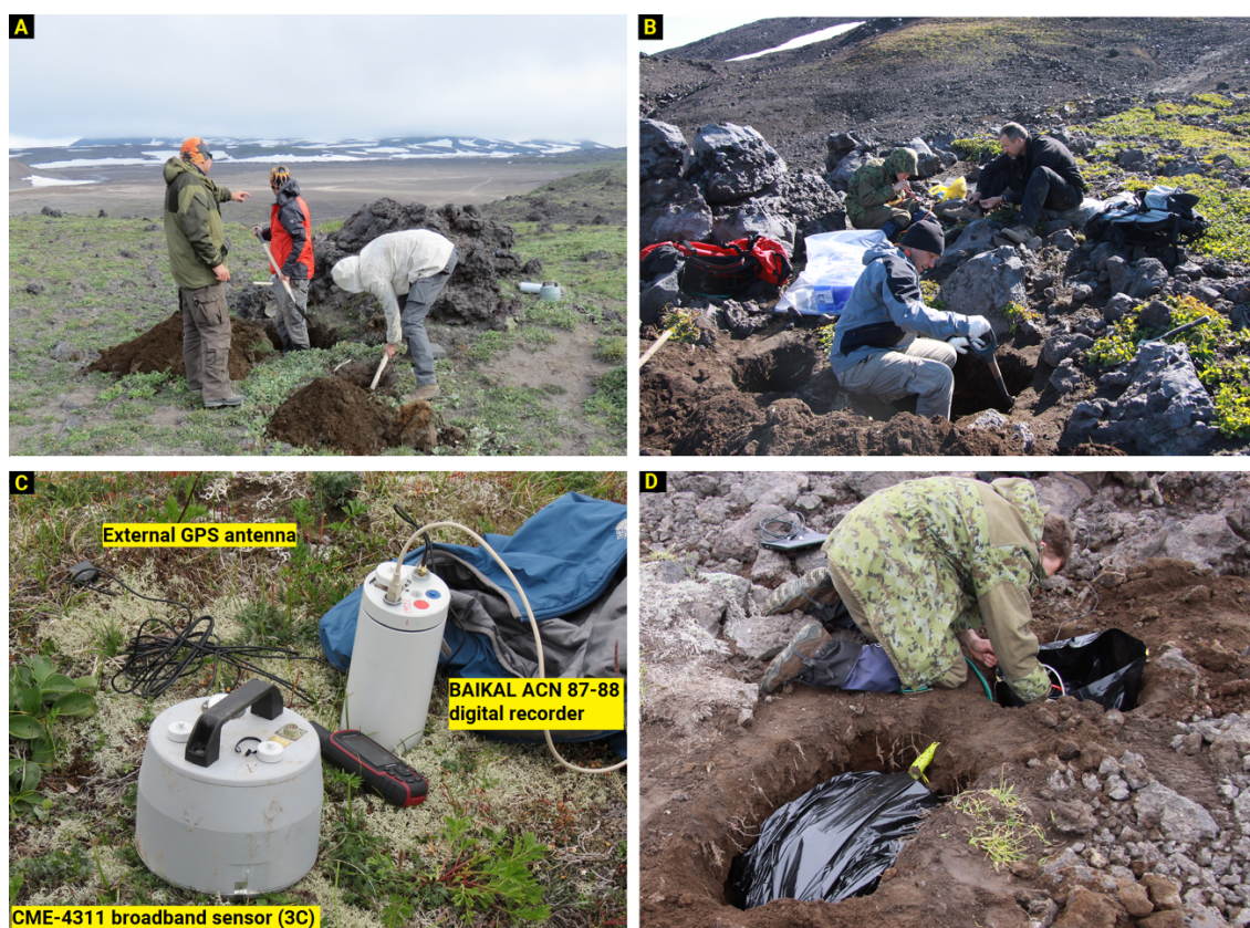
Figure 3.7 – Equipment of a temporary seismic station and the installation process. Photos are courtesy of field experiment team members: Nikolai M. Shapiro, Ilyas Abkadyrov and Andrey Jakovlev.
