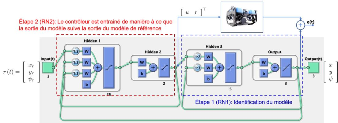
Figure 6.3 – Architecture CAMR utilisant Recurrent Neural Network
