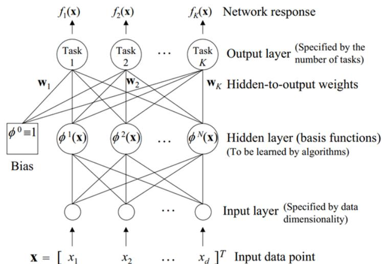
Figure 6.13 – Architecture de Radial Basis Function Network (RBF)
