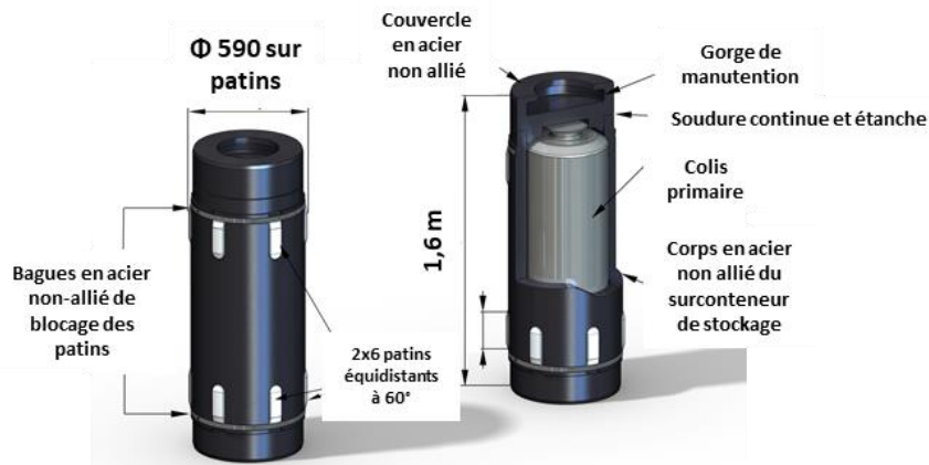
Figure I-2. Surconteneur en acier non-allié[2].
