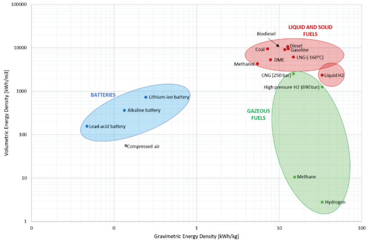
Figure 1.13: Volumetric and gravimetric energy densities of different energy storage systems. Figure from Panzone et al. (2020).
