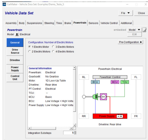
Figure 6.8: Powertrain configuration of Tesla-S
