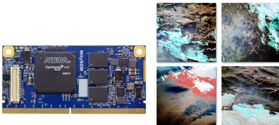
(a) Altera FPGA featured on OPS-SAT (b) Inference done onboard in 2021
